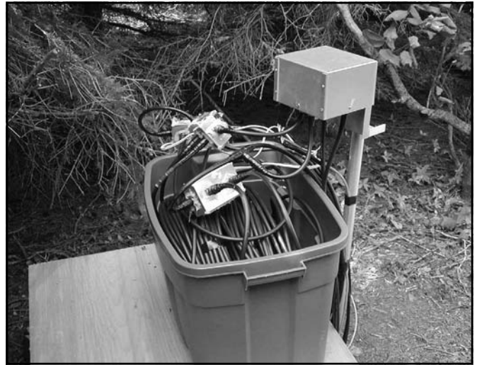
View of the 160-meter array phasing control system.
