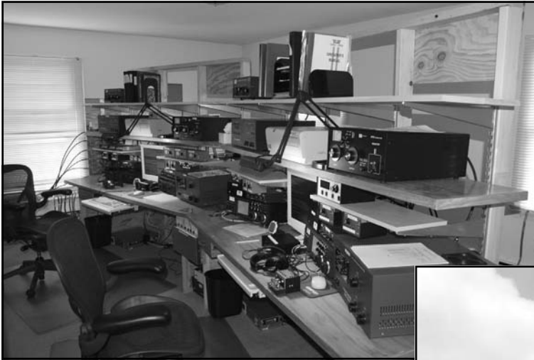
Figures 4 and 5—The new station and antennas at John, N3HBX's, contest station in Poolesville, MD. The station has four 190 foot rotating towers with stacks on 40–10 meters. In the shack there are two SO2R operating positions. See N3HBX's two-part series in the November/December 2005 and January/February 2006 issues of NCJ for more details on this contest station. Mark KD4D and John entered as a multi-single using KD4D. Mark did CW and John worked phone. John notes that looking at the scores of those who beat them indicates that they spent too much time on phone and too little time on 10 meters. However, he says they had a lot of fun and nothing broke! Their score put them in 4th place in the W/VE M/S category.
