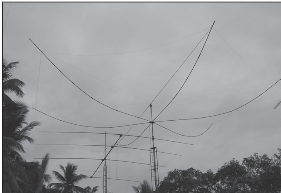
The 4S7AB antennas—a 4-element SteppIR in the back and a 40-meter homebrew Hex Beam in front.
