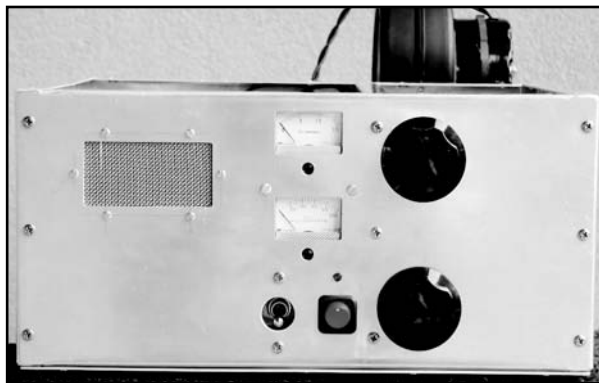
Fig 1—Front view, showing exhaust port on left, plate current meter on top at center, grid current meter at center, recessed power switch and amplifier IN/OUT switch with ground-trip LED above. On the top, the removable knob on the upper right is PLATE TUNE. The lower removable knob is PLATE LOADING. The air intake for the power supply is on the bottom of cabinet. The RF compartment is pressurized so that 95% of the air exhausts through the anode cooler and the rest exits thru the cathode compartment.
