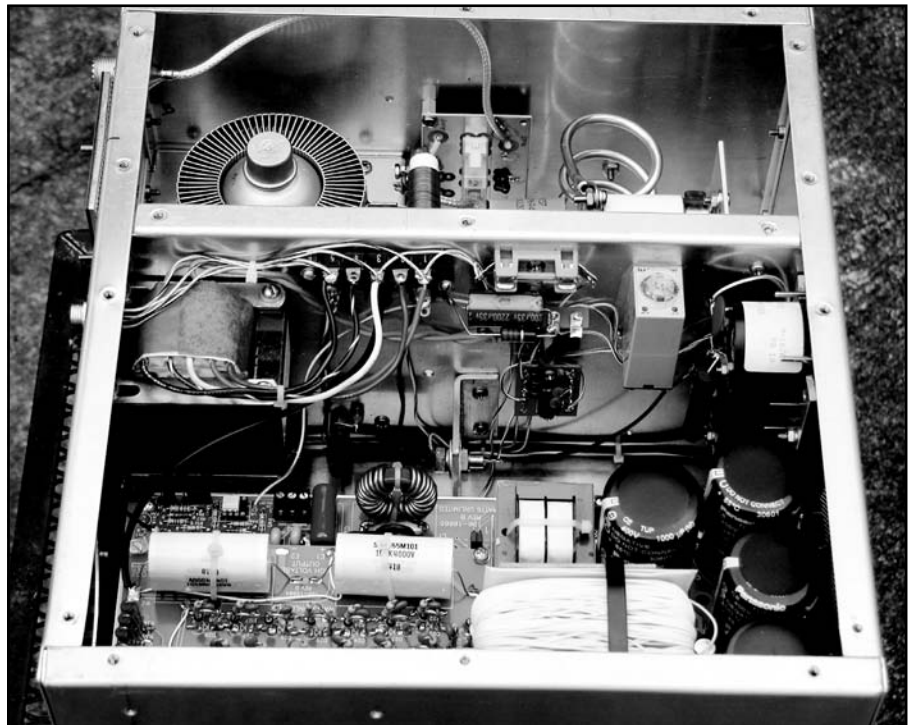
Fig 6—Another view of RF deck, showing the 8877, anode clamp and input/output relay-switching board, featuring the Schrack relays. Also note the Teflon RG-142 coax for the output. This coax will handle the 1.5 kW without meltdown! Also shown is part of the control circuitry—the Omron time delay relay and Tripplett 120G series plate and grid meters. The fuse at the center is for the amplifier cathode circuit. The filament/control transformer at the left is an Ameritron 406-1419-3J.
