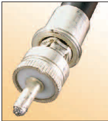
Figure 2 — You can easily see the cracks in the connector body in this photo.
