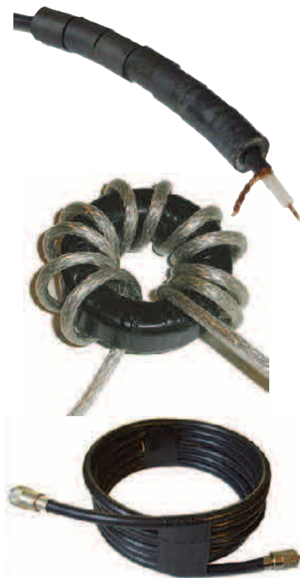
Figure 1 — All three of these choke baluns work by forming an inductance from the outside of the coax shield. The resulting reactance blocks RF currents from flowing, while leaving the currents inside the coax unaffected.
