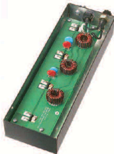
Figure 7 — MFJ addressed all of the concerns in this review in the MFJ-1164B. The new version uses PC board construction.
