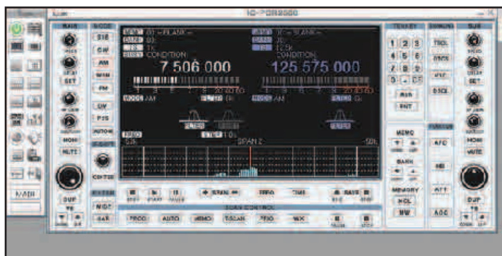
Figure 2 — Listening to a shortwave broadcast on the main receiver (left side of display) while monitoring aviation traffic on the sub receiver (right).
