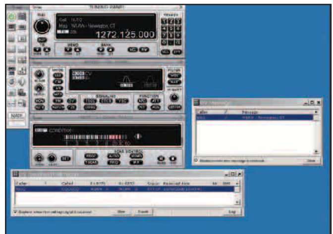
Figure 4 — Receiving a W1AW D-STAR transmission. The DV Received Call Record and DV Message windows open automatically.
