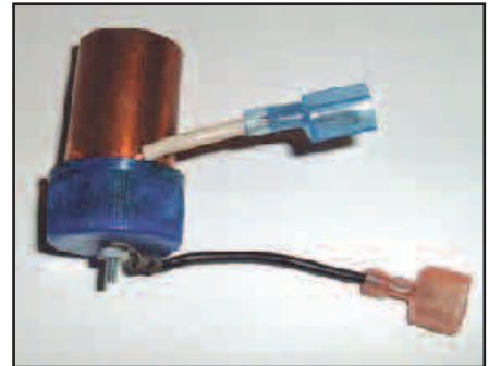
Figure 9 — K2PNK made a cigarette lighter receptacle using a 3/4 inch copper pipe coupling. This photo shows how he used a small machine screw in a soda bottle cap for the center pin connection. The ground lead is soldered to the pipe coupling and the cap is glued in place using epoxy.
