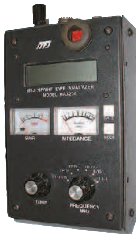
Figure 7 — W1VAK glued a rubber grommet to the front of his MFJ Antenna Analyzer to prevent the unit from being turned on during transit or storage.
