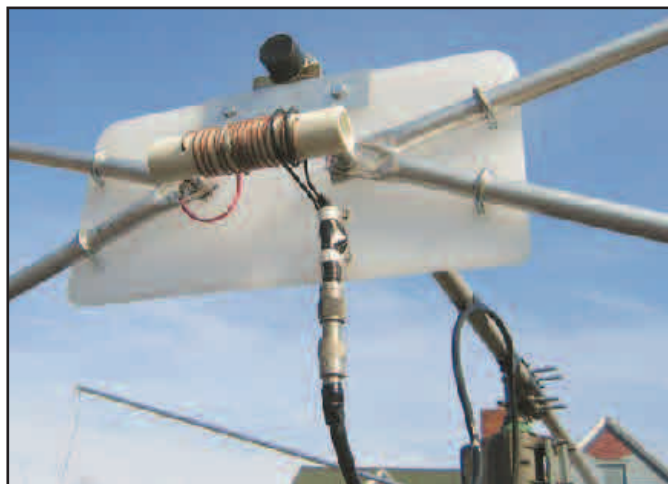
Figure 4 — The front side of the center support showing the loading coil, the coupled coil and the element radial mounting. Note the two plastic cable clamps that hold the coax and the coupling coil mechanically solid.
