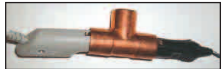
Figure 8 — K2PNK used a 3/4 inch copper pipe T to join two cigarette lighter plugs. The center pins of the plugs make contact in the center and the T provides the ground connection. If you are not using the side tap on the T, you might consider closing it with a pipe cap to prevent fingers or loose objects from falling into the T and shorting the center pins to ground.
