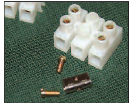
Figure 3 — Remove one of the contacts in the nylon barrier strip to make room for the LED and dropping resistor. Once the small flat-head terminal screws are removed (you may have to pry them out), the contact barrel can be pushed out.
