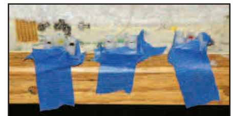
Figure 5 — After the LEDs are pushed into the barrier-block body, glue the LEDs in place. Here, epoxy was used, but other adhesives might be less messy. See the text for other ideas.
