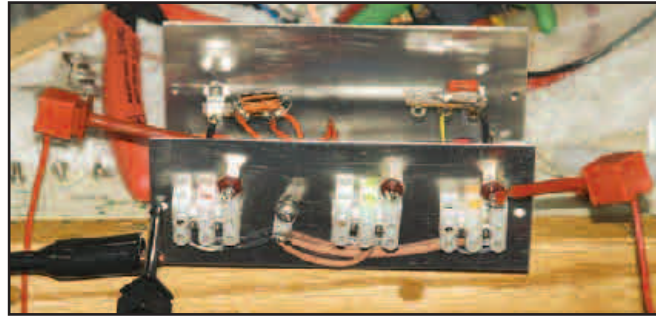
Figure 1 — KH6WZ recently built this dc-to-dc converter. It has three outputs, but has little room for a nice panel label, so an alternative “marking method” was needed.
