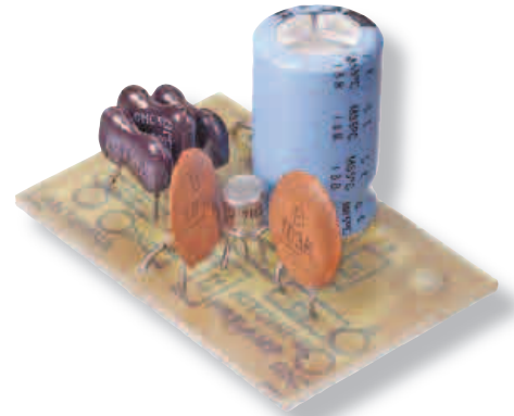
Figure 3 — A PC board version of the RF stage, including installed RFC, available from FAR Circuits ( www.farcircuits.net ).
