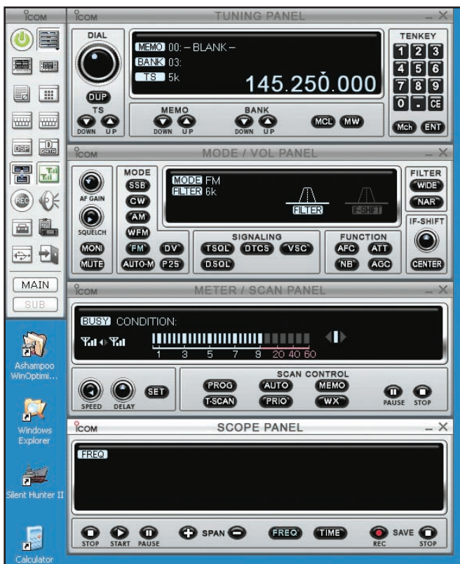
Figure 3 — Diversity reception on 2 meter FM. The Meter/Scan Panel shows the varying signal strength as the IC-R2500 "chooses" the main or sub receiver. Only the main receiver is displayed in the Tuning Panel while in the diversity mode.
