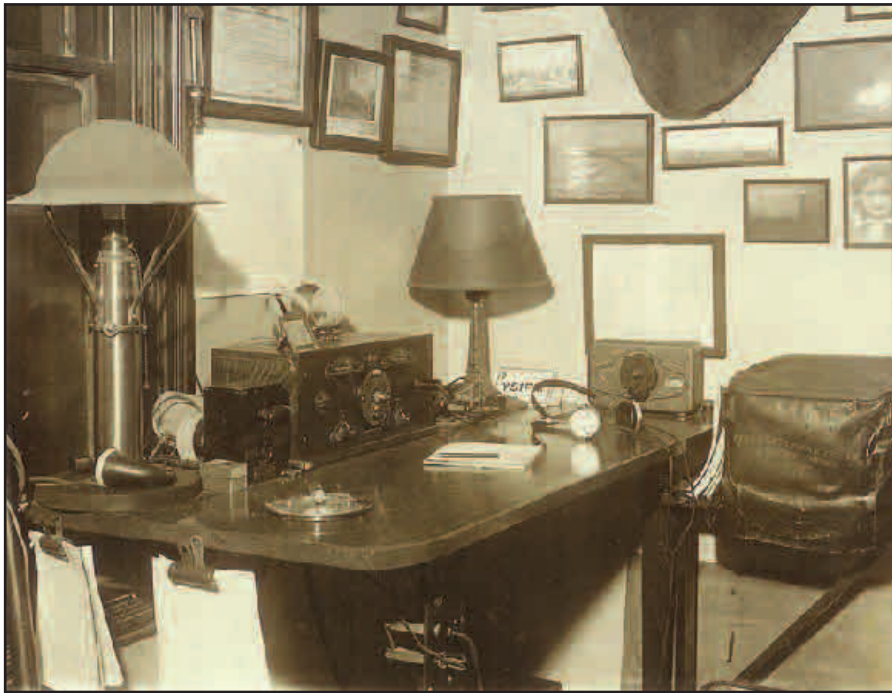
A late 1920s station owned by Roger W. Barrington, W3KW. If you look closely at the center of the set, you will see he replaced the small fine-tuning capacitor and dial with a larger dial and probably a larger capacitor. This would allow him fine-tuning over a much greater range. Also note the small metal box at the right end of the desk. I will have a column about this important ham station accessory in the near future. Do you know its purpose?
