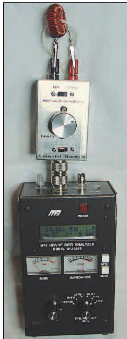
Figure 3 — Measuring the equivalent series resistance of an inductor.
