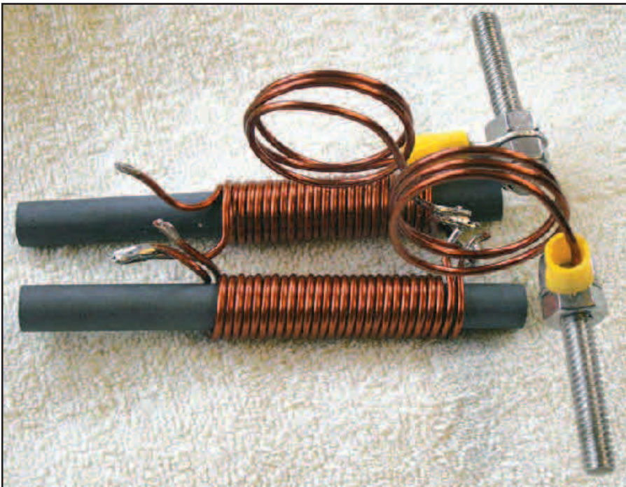
Figure 4 — Balun and loading coils.
