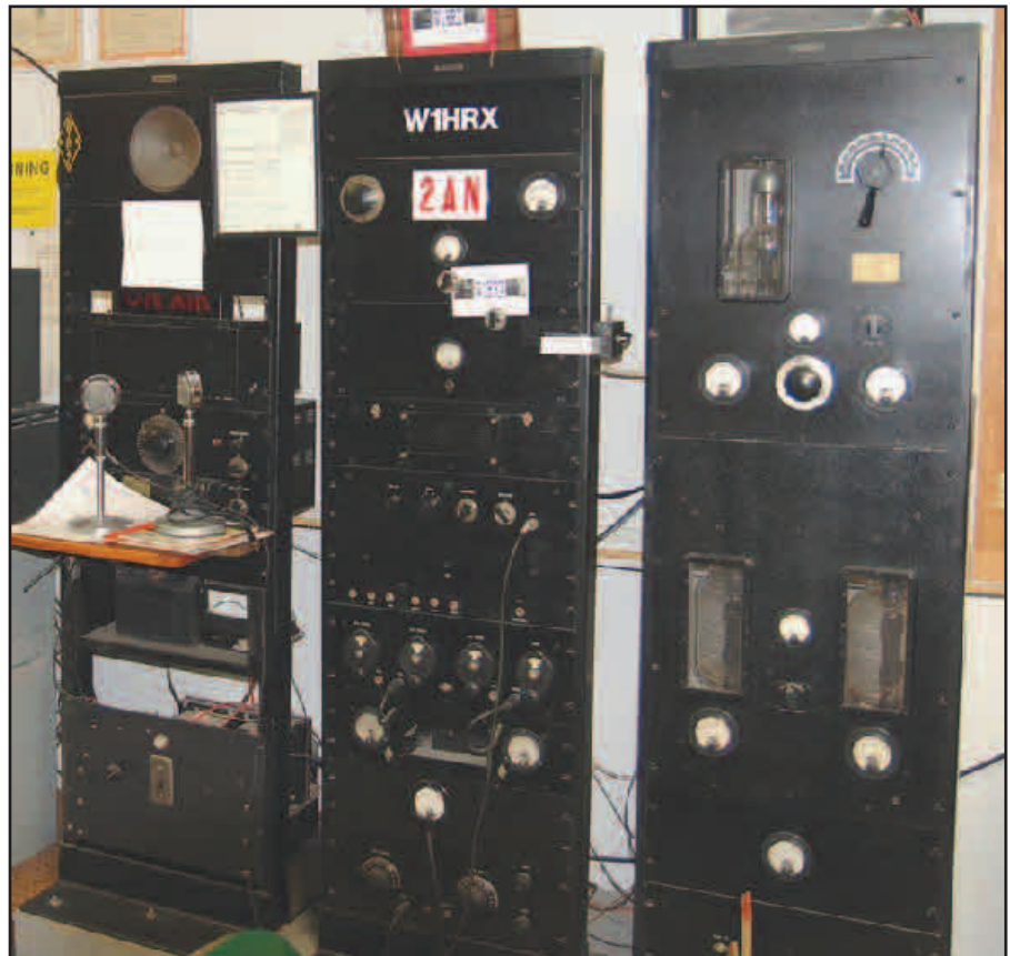
Figure 1 — An extreme example of early vacuum tube equipment: The James Millen memorial station, c 1936, in operation at the AWA museum annex in Holcomb, New York. Millen, W1HRX, was the chief designer of the original National Radio HRO receiver (in left rack, above shelf) and later formed his own company. The transmitter was built by Millen and then QST Associate Editor Ross Hull.
