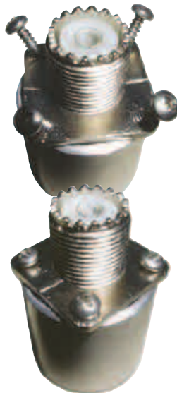
Figure 1 — The screws are started into the aluminum tubing.
