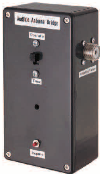
Figure 1 — Front view of the audible antenna bridge.
