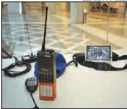
One of the San Jose RACES portable ATV monitoring positions with a cable ready portable LCD TV.
