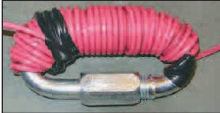
Figure 4 — Here is the completed inductor, ready to be wrapped in electrical tape or some other method to hold the turns tightly in place on the form.
