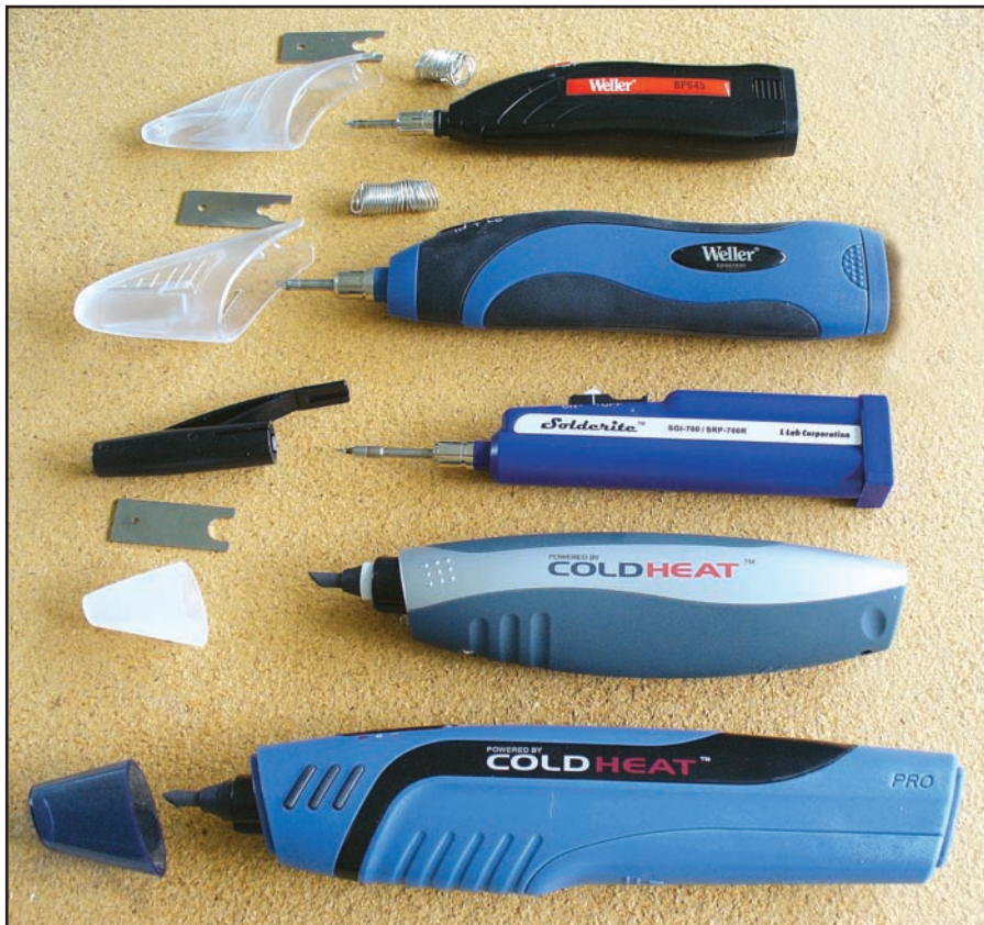
Here are the five battery powered soldering tools reviewed this month, along with their protective caps, tip wrenches and solder (if included). Top to bottom: Weller BP645MP and BP860MP, Solderite 700, ColdHeat Classic and ColdHeat Pro.
