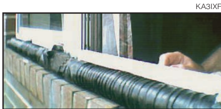
Figure 10 — This photo shows the completed KA3IXF Apartment Dweller's Antenna on the windowsill outside his apartment.
