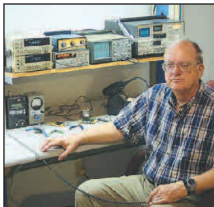
Figure 5 — The author at his electronics bench, two surplus commercial ESD workstations. His wrist strap and ESD-safe soldering iron are visible.
