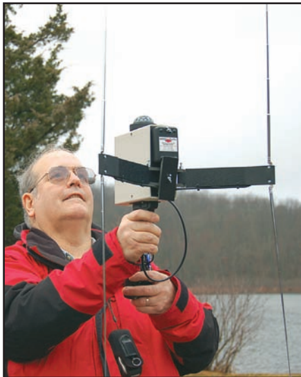
Figure 1 — WR1B using the National RF VF-142QM TDOA radio direction finding unit.
