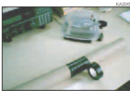
Figure 8 — This photo shows how KA3IXF wrapped Christmas-wrapping-paper tubes with electrical tape to form a core for his helically wound antenna.
