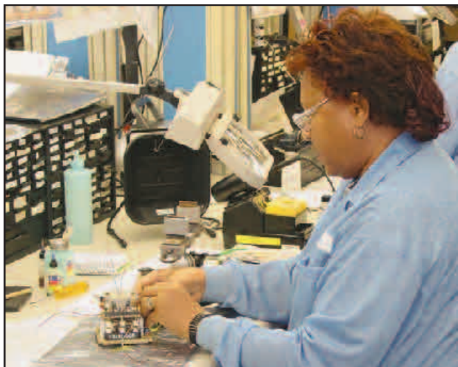
Figure 1 — Ora Remmer at a typical industrial ESD workstation showing the various ESD safeguards (see text).
