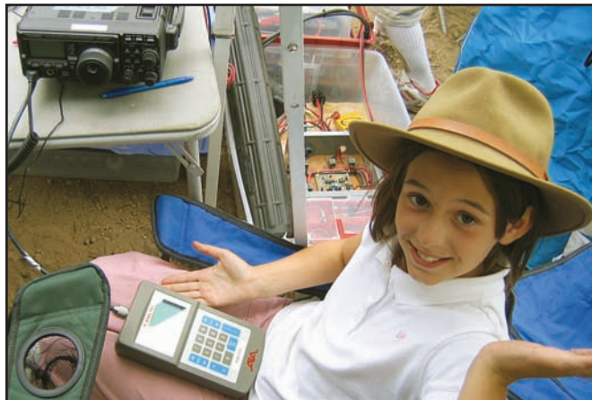
Becky, KI6CRN, uses her grandfather's SWR-121 to check the match on the Buddipole antenna from the Independent Radio Club 2006 FD site at Table Mountain Campground in Wrightwood, California. This time the match was 1.2:1 — not bad!
