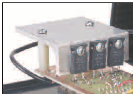
Figure 3 — Close-up view of three Caddock TO-220 style bridge resistors mounted on the heat sink.
