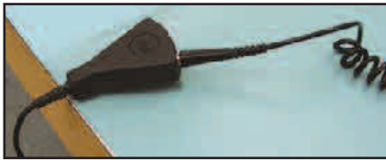
Figure 3 — Common ground point that is a part of the 3M mat with the wrist strap attached.
