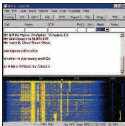
Figure 3 — Screen shot of PSK31 reception using DigiPan software. Note the spectral display indicates multiple signals, one with each line. The DigiPan filtering allows you to tune a signal with just a click.
