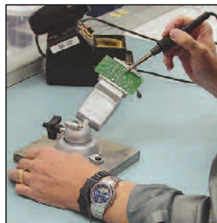
Figure 2 — An ESD-safe work mat and wrist strap. This is the setup I use to develop prototype electronics at work.
