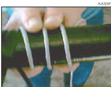
Figure 9 — After securing the coaxial cable feed line to the center of the cardboard tubes, KA3IXF wound the antenna wire around the tube to form a helically wound antenna.
