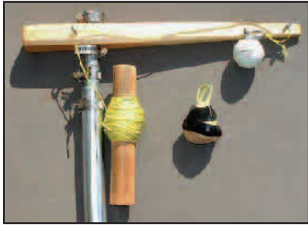
Figure 5 — The top of the pole in its collapsed state, showing the cross arm, hose clamps and weights.
