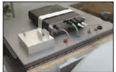
Figure 7 — A rear view of the KH6WZ 24 GHz system. The aluminum block houses a "keylock" switch for sending a carrier beacon. The small shaft peeking out of the block is connected to a microswitch, for CW keying.
