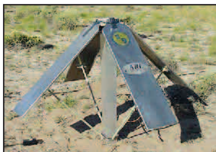
A wide-bandwidth inverted-V "blade" antenna under test at the Long Wavelength Array.
