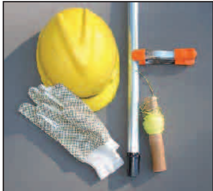
Figure 6 — The lower end of the pole, showing the string being held taut and the suggested safety equipment.
