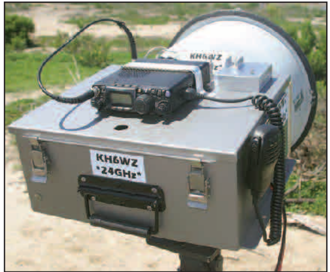
Figure 6 — The completed 24 GHz system, from the operator's point of view.
