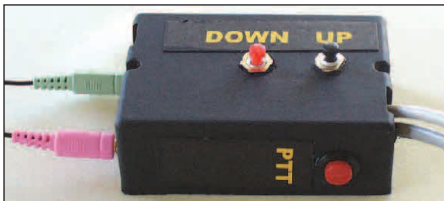
Figure 3 — View of control module of the headset adapter showing the location of the buttons.
