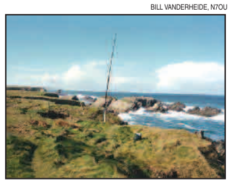
The 20 foot fiberglass fishing pole that supported my end-fed wire.
