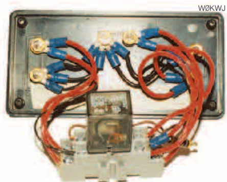
Figure 4 — This view shows how the relay is mounted on a socket, with wiring between the socket and the binding posts. Notice that the no. 16 AWG wiring is doubled for all wiring runs, to increase the ampacity of the wiring.
