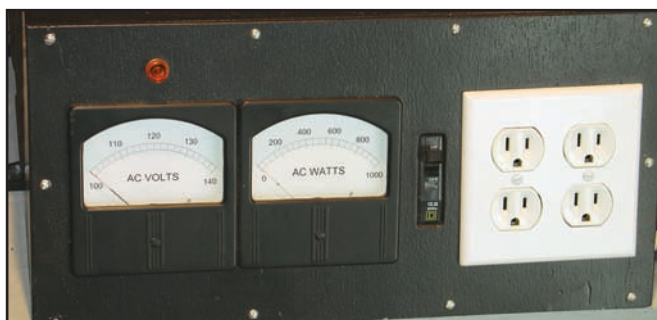
Figure 3 — Control box showing voltage meter, “wattmeter,” circuit breaker and ac outlets.
