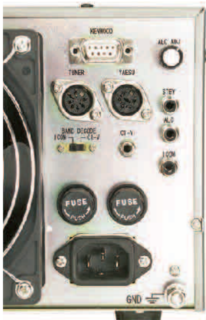
Figure 2 — The rear panel includes connections for the amplifier to receive band information from ICOM, Yaesu and some Kenwood transceivers. Supplied cables make for a no-fuss installation if you have a compatible radio.
