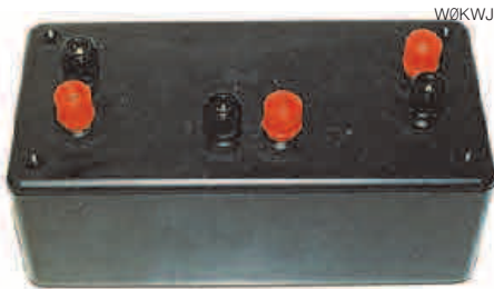
Figure 3 — This photo shows how W0KWJ installed binding posts on a project box cover to connect his radio to an ac power supply or a battery.
