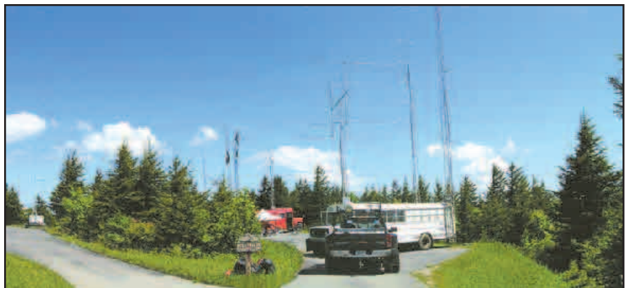
Figure 2 — A panoramic view of the K8GP operation. The generator trailer is to the left with the third 6 m beam stack. Three buses to the right: three 2 meter arrays on the white bus, 222, 903/1296 MHz and two microwave dishes on separate towers on the first red bus and two 6 m arrays and the 432 antenna on the second red bus (antennas only visible over the trees in the center).
