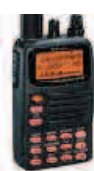
VR-500 100 kHz to 1300 MHz (1.3 GHz) less cellular, in AM, FM-N, FM-W, LSB, USB and CW
