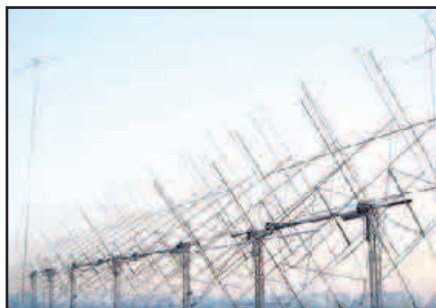
Figure 2 — The ARRL EME Contest is under way and even small stations have a chance to do moonbounce. Here is currently the largest 2 meter EME array, used by Sam, RN6BN (KN95) — 64 15-element cross-polarized Yagis stacked 4 high and 16 wide.
