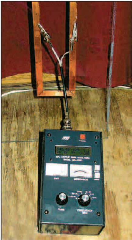
Figure 5 — A short length of coaxial cable with alligator clips on one end makes a convenient test fixture for finding the feed point on the copper tape J-pole antenna.
