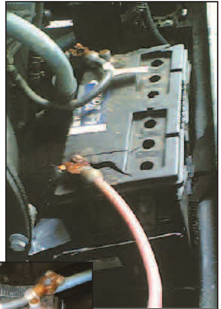
Figure 2 — Another view of the remains of the exploded battery.
