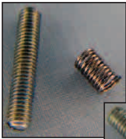
Figure 2 — Steel wire wrapped around #6 screw and ready to be installed on a slug.
