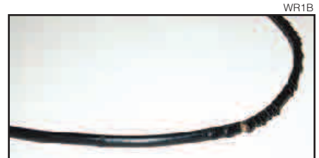
Figure 7 — Thomas Lally, W1NSS, says deer destroyed his coaxial cable. Whether they sliced it with their antlers or tried chewing on the cable, this was the result.
