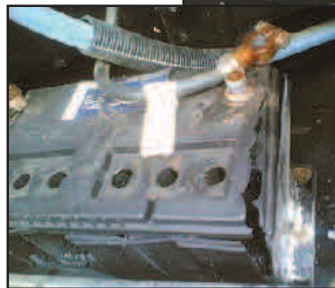
Figure 1 — This is a view of what's left of the battery that caused the author to lose part of his hearing.
