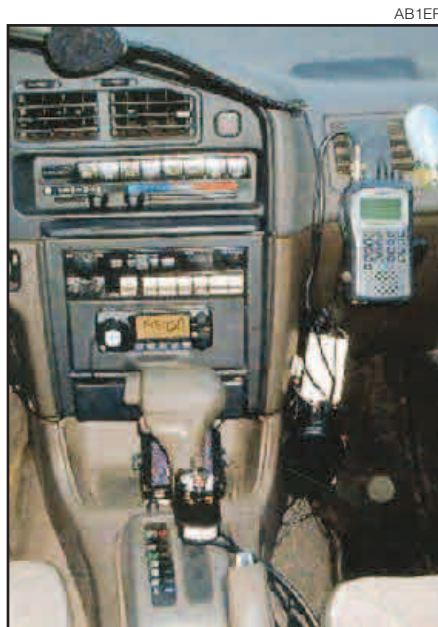
Figure 6 — The boom microphone is attached near the top of the dash, where the microphone clip had been attached previously. The PTT switch is attached to the shift lever.
