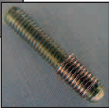
Figure 3 — Wire in place on end of a slug and ready to be inserted into coil.
