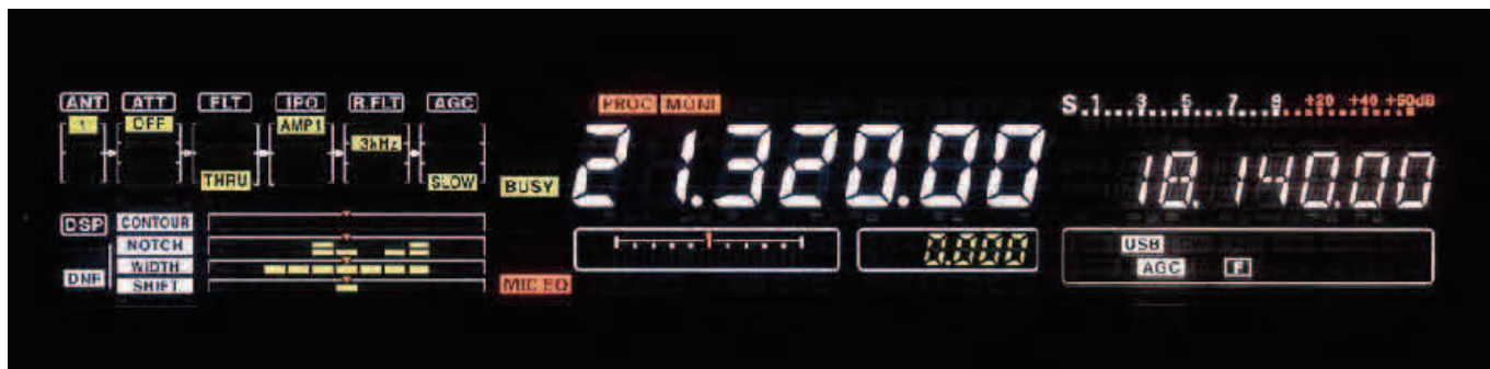
Figure 3 — The Yaesu FT-2000 graphically indicates which roofing filter (15, 6 or 3 kHz), R.FLT , is selected.
