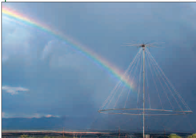
The Discage antenna at the Titan II Missile Museum, Green Valley, Arizona, is available for use by licensed ham radio operators, thanks to the Green Valley ARC.
