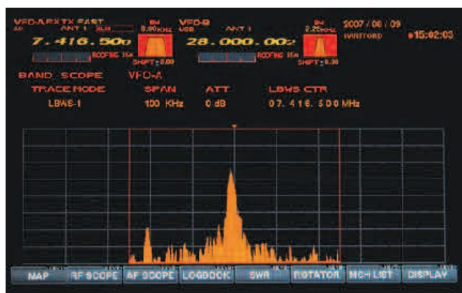
Figure 5 — Here's the DMU spectrum scope looking at a 100 kHz slice at 7 MHz. The DMU simultaneously displays frequency and other transceiver operating parameters. DMU functions are selected by the buttons at the bottom of the screen.
