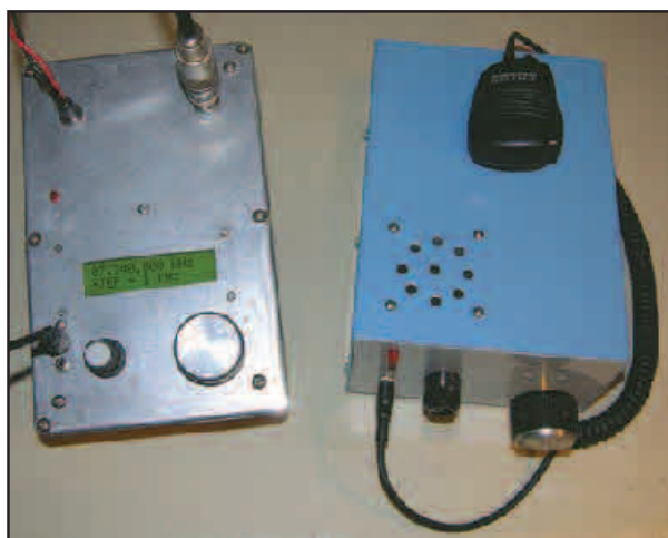
View of two versions of the SSB transceiver. The example on the left includes the FREQ-Mite frequency counter offered by Small Wonder Laboratories .
