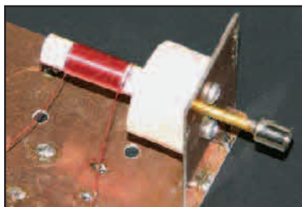
Figure 4 — View of the wooden dowel slug interfacing the brass screw and the soda-straw coil used as part of the PTO in the second version.
