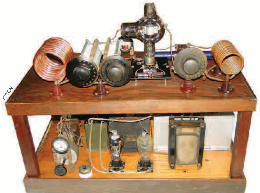
Restored transmitter with new knobs, new 52 tube, tube socket and new trim moldings.
