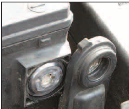
Figure 1 — Close-up of side terminal battery connector.
