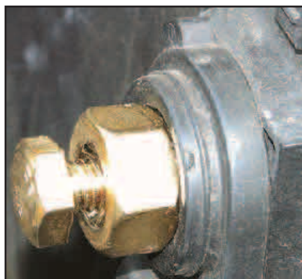
Figure 2 — Photo of the proper type of radio connection for a Delco side-terminal battery.
