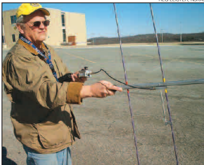
Jim Toth, K3CHJ, was the lead tracker using: a modified 3 element Arrow Yagi modified to WB2HOL "tape measure" specs; ICOM IC-W32A and homebrew 2 MHz active offset attenuator.
