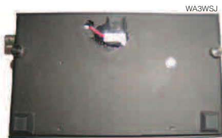
Figure 6 — This photo shows how WA3WSJ brought a set of leads from the battery pack out on the bottom of the KX1 case to connect the battery charger.
