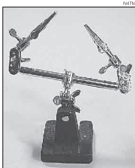
Figure 1 — A "third hand" is useful for holding small parts and small circuit boards while soldering.
