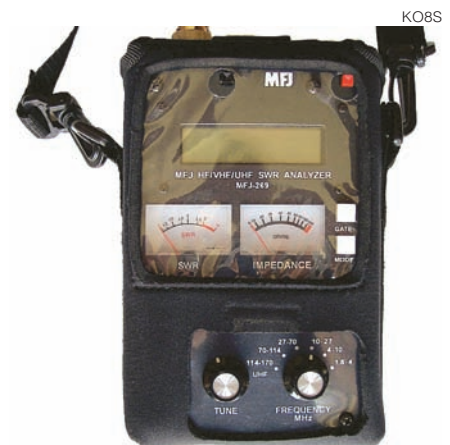
Figure 3 — KO8S modified the carrying case by cutting an opening to show the FREQUENCY and TUNE labels on his MFJ-269 Antenna Analyzer.
