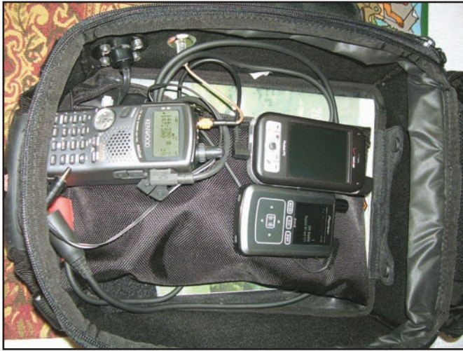
The Kenwood APRS-ready transceiver (left) shares space with a cell phone and satellite radio. The communicator, which provides voice communications via push-to-talk or VOX to the rider and passenger, is below.
