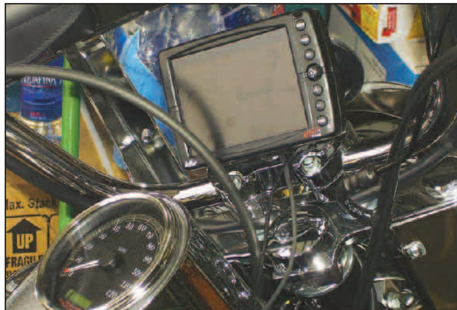
The AvMap G4T GPS unit mounted atop the handlebars.
