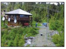
The KL7FF QTH: The 2 meter 12 element Yagi can be seen mounted on the mast on the deck to the left side of the cabin. The 6 meter 8 element Yagi can be seen in the right foreground, mounted on 3 tower sections. The 2 meter station ran 400 W output and the 6 meter station ran 600 W output.
