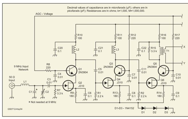
Figure 4 — Schematic diagram and parts list for complete IF amplifier and AGC system for receivers.
