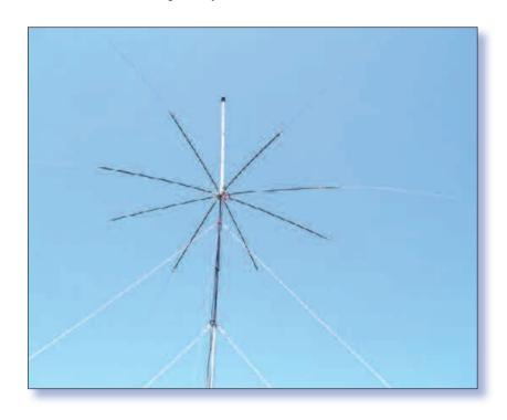
dipole taken to extremes. The basic plan was to find an attachment mechanism that could be mounted on a mast and accept up to four helical dipoles, eight helical type antennas, radially around the mount in the horizontal plane.
