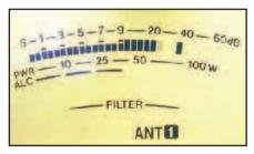
Figure 3 — Much better! I've lost a bit of RF output (top scale), but now there is no ALC activity (bottom scale).
