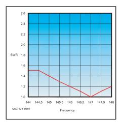
Figure 1—EE-3 2-meter SWR plot.
