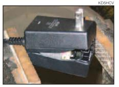
Figure 6 — The wall-wart case has started to split open under gentle pressure from the vise jaws.
