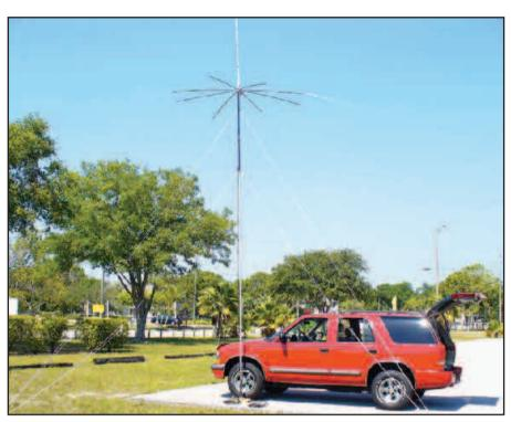
Figure 4 — Here is a view of the octopus all set up for park-side DX or disaster recovery operations. The SUV, sitting on the mast base, keeps the whole array erect. The guy lines in the picture would be used only if the vehicle was needed elsewhere.
