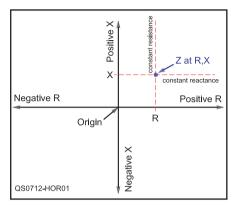
Figure 1 — This graph shows the rectangular coordinates for any impedance against the resistance (R) and reactance (X) axes.
