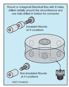
Figure 2 — A drawing of the electrical box showing the holes drilled for the stud mounts, four of which are insulated from the box and four of which are grounded to it.
