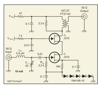
Figure 1 — Traditional JFET cascade IF amplifier. The computer simulated gain of this circuit is 23.5 dB at 9 MHz. Measurements produced similar values.
