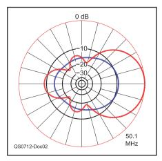
Figure 2 — Azimuth pattern of three element 6 meter Yagi in free space (red), compared to the same antenna with a 10 foot mast behind the driven element.
