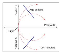
Figure 2 — Distorting or mapping the rectangular graph captures all of its righthand side impedances inside the circle formed by the bent reactance axes. This is the basis of the Smith Chart.
