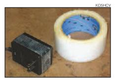
Figure 8 — You could glue the case back together, but heavy plastic tape will make the next repair easier.
