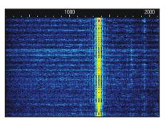
Figure 1 — A real-life stinky PSK31 signal. Notice the lines to the left and right of the signal track in the waterfall display. This is actually a mild offender; I've seen much worse with garbage throughout the display.
