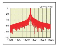
Figure 2 — Worst-case spectral display of the Yaesu FT-450 transmitter during
