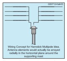
Figure 3 — This shows the schematic diagram of the wiring of the antenna elements.
