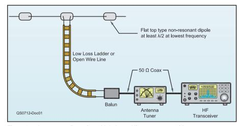
Figure 1 — Antenna configuration with balanced line to coax transition.
