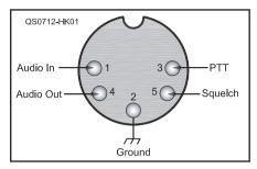
Figure 1 — Connections at 5-pin DIN plug to fit FT-221 accessory socket. (Note that this is a mirror image of the socket's pins.)
