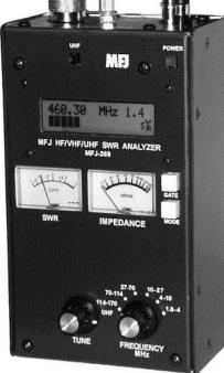
yagis, quads and others and determine their SWR, resonant frequency and bandwidth.
