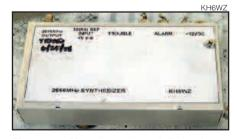
Figure 2 — Many "store-bought" aluminum chassis boxes these days are made of flimsy material. In the case of my 2556 MHz synthesizer, some frequency wobble was attributed to the wobbly box.
