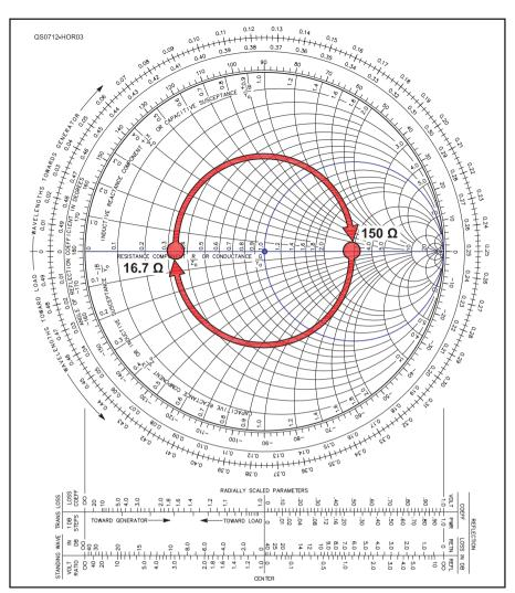
Figure 3 — Plotting the impedances measured on an SWR analyzer forms a circle as the electrical length of a line of fixed length increases with increasing frequency.
