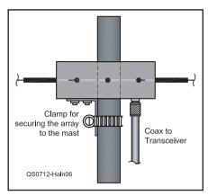
Figure 6 — This diagram shows clearly how the hub is secured to the mast to allow "armstrong" rotation of the array, if needed.
