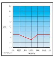
Figure 2—EE-3 1.25-meter SWR plot.
