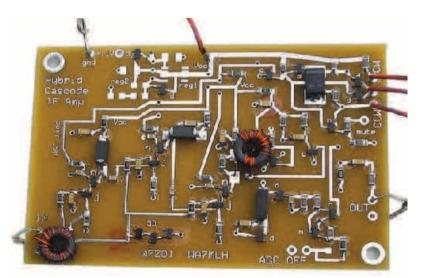
Figure 5 — A printed circuit board version of the IF amplifier using surface mount (SMT) components. The regulator was not installed when the circuit was built and tested with V<sub>cc</sub> of 9 V.
