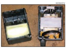
Figure 7 — With the case carefully cracked open, you can repair a broken wire or replace a diode or capacitor.
