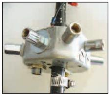
Figure 1 — The hub of the array is a standard octagonal electrical box available at your local home improvement store. Stud mounts available from your local ham radio or CB shop are used to mount the mobile antenna pairs.
