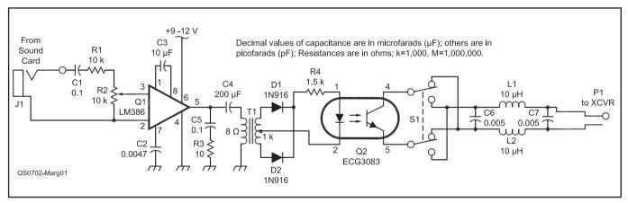
Figure 1 — Schematic diagram and parts list for the CW interface. See www.mouser.com.
