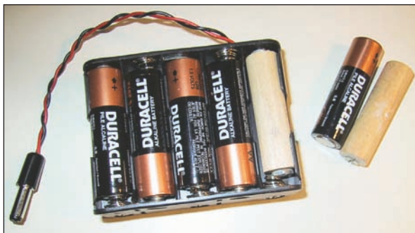
Figure 3 — A dummy cell voltage reducer at work.
