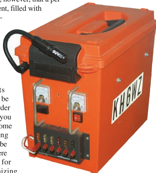
Figure 2 — A sportsman's "dry box," found at sporting good shops, is used to house this emergency power source.
