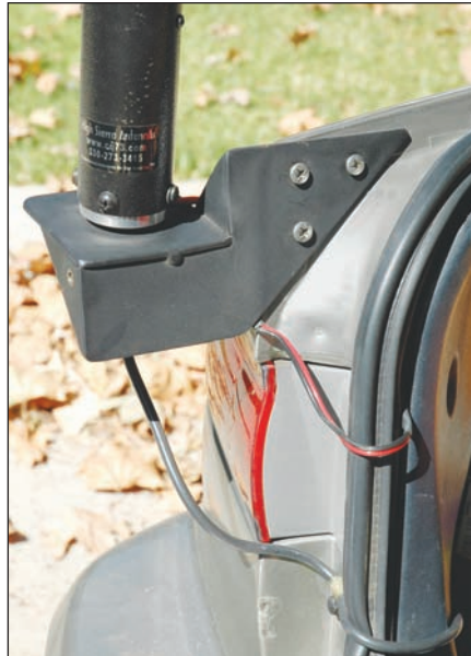
Figure 5 — View of the completed mount.
