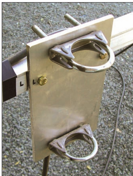
Figure 6 — Plate installed on square boom.
