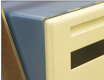
Figure 5 — This instrument cabinet has a front panel with a “lip” around the perimeter. This would be very difficult to duplicate, so I decided to recycle the original front panel, and customize it for a new project.
