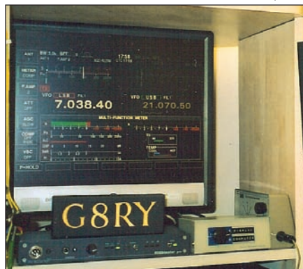
Figure 1 — Using a data switch to interface a flat-screen monitor to the ICOM IC-7800.
