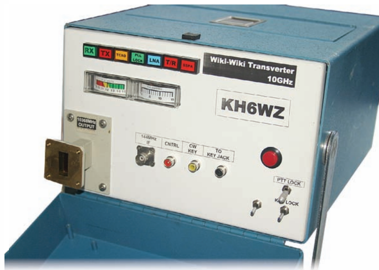
Figure 9 — The refinished front panel looks almost brand-new. Labels are made with Microsoft Word and Avery labels. My call sign on the upper right will be backlit with LEDs: green for transmit and red for receive.
