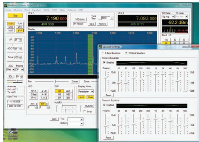
Figure 6 — PowerSDR offers 3 or 10 band graphic equalizers for both receive and transmit.
