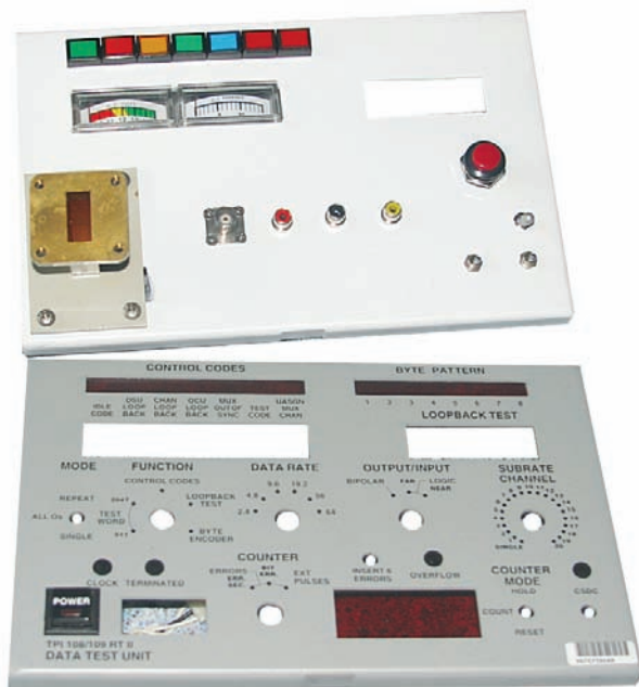
Figure 8 — This is what the patched and refinished front panel looks like. Even some of the holes were “recycled.”
