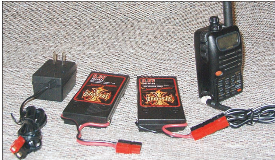
Figure 4 — The complete system: charger, battery packs and FT-50.
