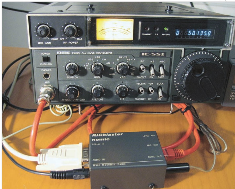
The author's 6 meter radio, connected to a popular sound card interface, is used for SSB/EchoLink operation.
