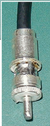
Figure 11 — Tighten up the adapter until there is no gap between it and the connector body.
