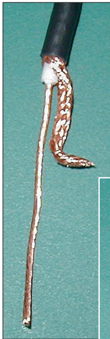
Figure 8 — Trim and bend the shield to get it ready for insertion into the connector.
