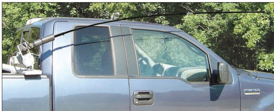
Figure 5 — Antenna shown in stowed position (leaving enough room to open passenger door).
