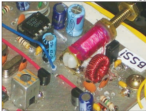
Figure 2 — Details of the permeability tuned oscillator (PTO) tuning inductor. The PTO has about a 130 kHz tuning range, so a jumper is provided to move between CW and voice band segments.
