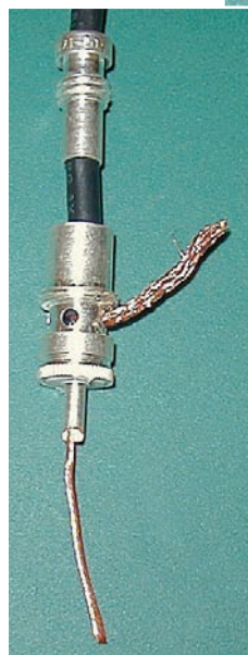
Figure 10 — Pull shield out through the prepared hole.
