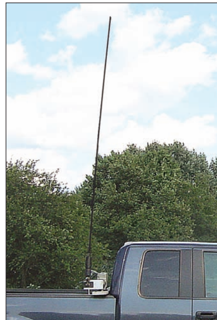
Figure 1 — The problem — 12 foot high antenna, 7 foot high door!
