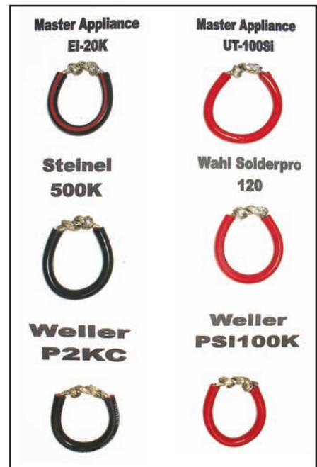
Figure 11 — A sample test setup, this one for 10 gauge wire connections for the six units tested.
