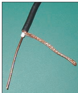
Figure 7 — Strip center conductor down to within \frac{1}{8} inch of the braid.
