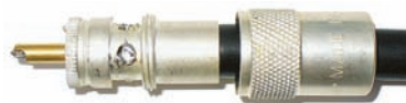
Figure 14 — A typical example of the very neat soldering possible with a butane powered iron on a PL-259 attached to RG-8 coaxial cable. The braid shield was tinned using the same iron before the final connection.
