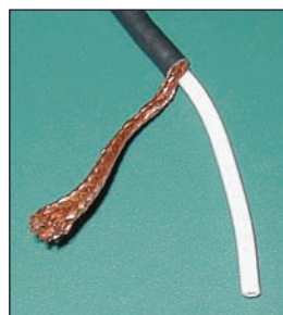
Figure 5 — Pull center conductor out of the shield braid.
