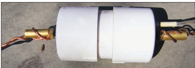
Figure 6 — Completed and sealed pneumatic switch housing with 80 meter extension wire (left), 40 meter wire (right) and attached pneumatic tubing (right).
