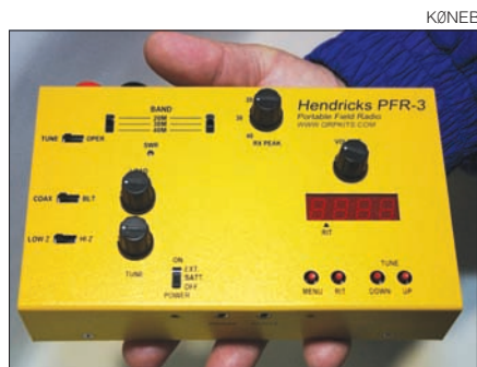
Figure 2 — Advanced kit builders can take on projects such as this 40-30-20 meter, 5 W, QRP CW rig from Hendricks QRP Kits.
