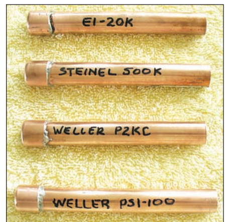
Figure 12 — Those units that included blowtorch tips worked acceptably for soldering ½ inch copper tubing that might be used to build a J-pole antenna.
