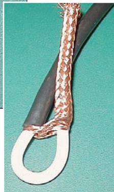
Figure 5 — Pull center conductor out of the shield braid.
