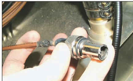
Figure 1 — Oops! This type N connector had its ratings exceeded.
