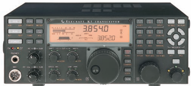
Figure 5 — The Elecraft K3. It looks like a traditional amateur transceiver, but is actually an SDR.
