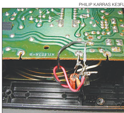
Figure 2 — The dead-bug installation of the power regulator directly onto the receiver's circuit board.
