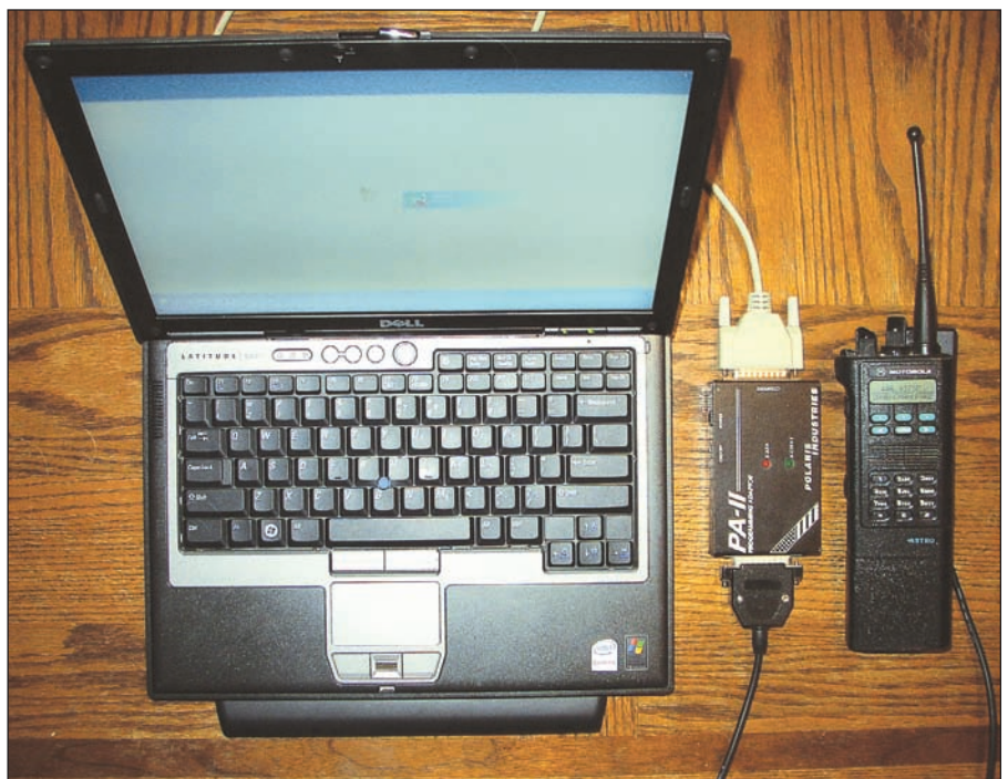
To reprogram a Motorola Astro Saber, you need Motorola’s programming software, a Radio Interface Box (RIB) and the appropriate cables. You can find the RIB and cables on eBay and other sites.
