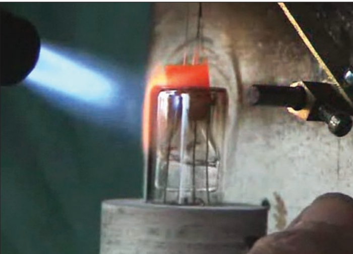
6 Welding the glass parts together.
