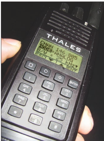
The Thales 25 (formerly Racal 25) is a P25 digital radio covering the 136-174 MHz band. Notice that this one has been reprogrammed for use on the 2-meter ham band. It features a very intuitive user interface, which allows channel parameters to be quickly programmed or changed from the front panel.
