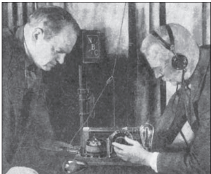
Left, Dr Orestes H. Caldwell, and Dr Clayton H. Sharp tuning the simple receiver with the 50 year old Edison tube.
