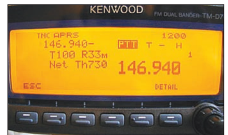
Figure 8 — Typical flashed display of a new local packet. We like to concentrate information into the first 20 or 28 bytes of a packet so that it displays well on the 10x10 display of the 'D7 and the 10x10x8 display of the 'D700 shown here. This packet shows the local repeater, its tone, its typical range and its weekly net time.
