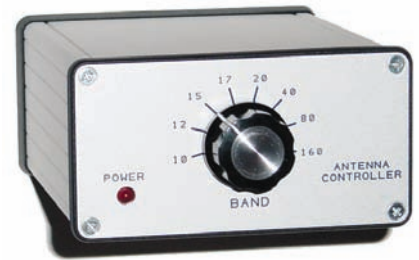
Figure 8 — Completed antenna controller. This one is set up to cover all HF bands except 30 and 60 meters.
