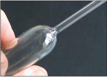
4 Attaching the air evacuation tube to the envelope
