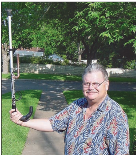
Charlie Schlieper, N5TD, of Temple, Texas built this unique adaptation of a 70 cm J-Pole antenna into a walking cane for Mike, WB5PBS. He says the coax tap was higher than expected, but it achieved an SWR of 1.1:1 at the UHF D-STAR frequency of 440.525 MHz.
