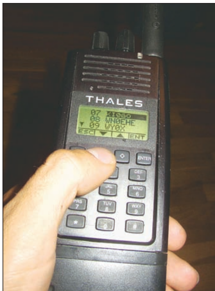
On the Thales/Racal25, accessing the unit ID list to make an individual call is as simple as pressing and holding the pound (#) key.
