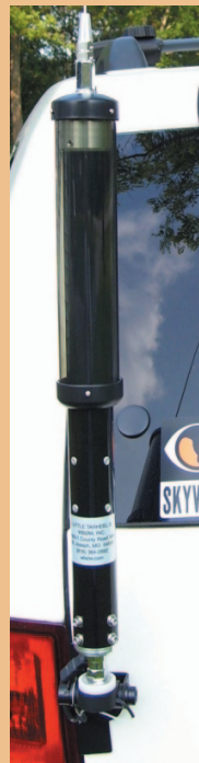
Little Tarheel II Shown Mounted on Diamond K400-3/8C
