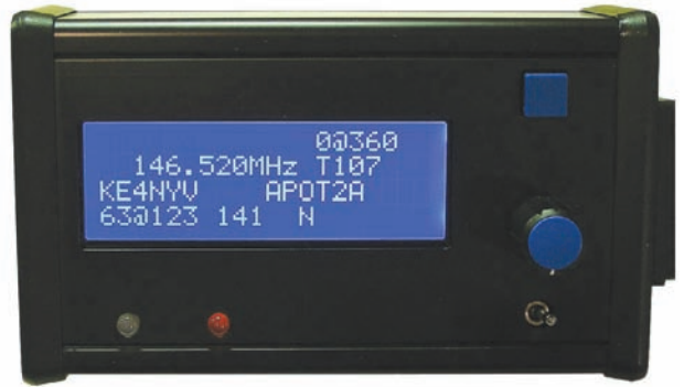
Figure 6 — This HamHUD display shows that station KE4NYV is 141 miles north and is doing 63 mi/h on a heading of 123°. His device is identified as an OpenTracker2 (APOT2A). His position report includes his voice operating frequency as 146.52 with a tone of 107 Hz for voice contact. His position is translated to a waypoint and displayed on the map of the attached GPS.
