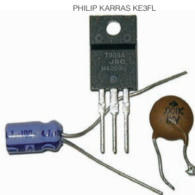
Figure 1 — All that's needed to adapt a 9 V radio to a 12 V battery.
