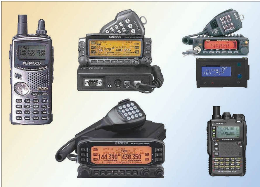
Figure 2 — For over 10 years, there have been a variety of fully integrated APRS radios as shown here. Shown left to right (top row), first was Kenwood's 'D7 and then 'D700. Then the Alinco DR-135 with add-on HamHUD to give it an APRS display capability. Then (bottom) in 2007 the fully capable 'D710 and recently the VX-8R was announced by Yaesu.
