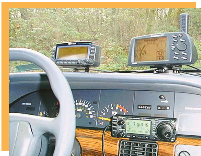
Figure 1 — W4HFZ's typical mobile setup includes VHF, UHF, HF, a GPS and APRS.
