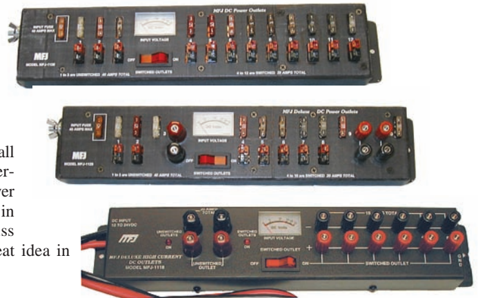
Figure 2 — Selection of dc power strips available from MFJ.
