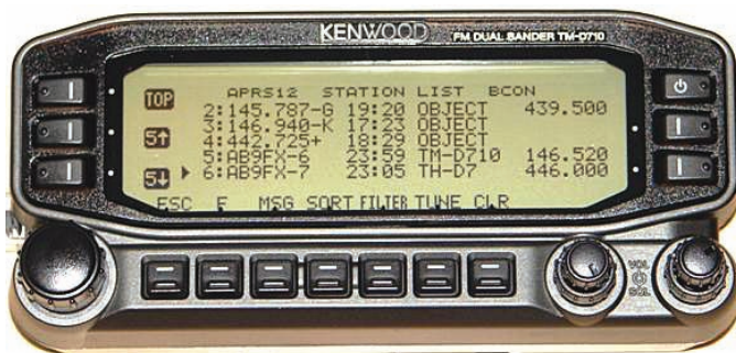
Figure 3 — The new 'D710 mobile radio includes an added column for frequency information and also has a TUNE button for instant QSY to contact one of those stations. The first three objects are nearby voice repeaters, and AB9FX has two stations nearby, another 'D710 monitoring 52 and his 'D7 handheld monitoring 446.000.
