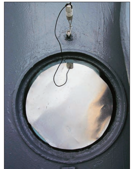
Figure 3 — Outer capacitor plate and end support of antenna wire.
