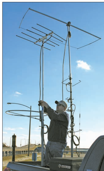
Figure 2 — To raise the antennas in a new location, Steve attaches the beams at the top of the telescoping painter poles and then pushes them up. The loops are always attached. The poles reach 19 feet above the ground when fully extended.
