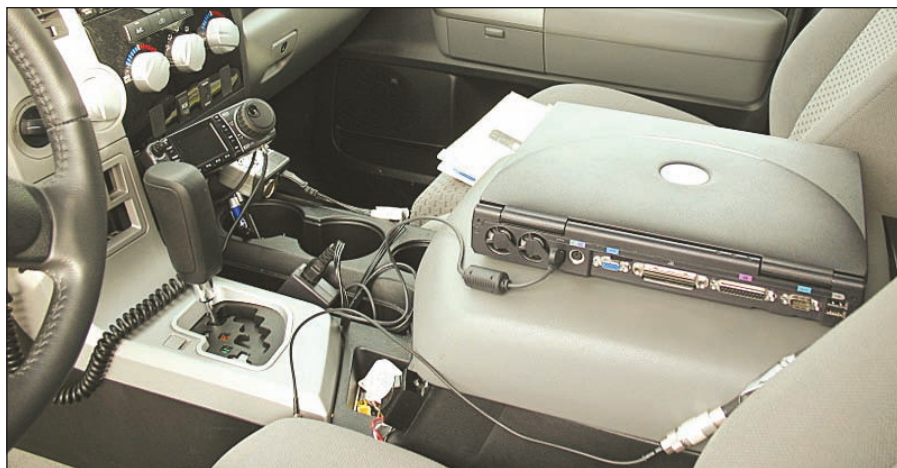
Figure 1 — Effective operation while mobile or portable is made a lot easier if the radios and logging gear are neat and secure. Today's all-band, all-mode radios put out a great signal on 6 meters, 2 meters and 70 cm.
