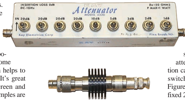
Figure 6 — Various attenuators used in the project. Step attenuator shown at top and 10 W power attenuator at the bottom.
