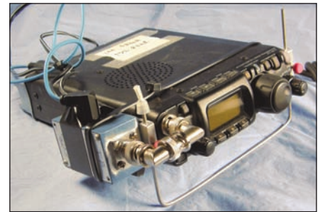
Figure 4 — The complete Bias-tee mounted on the FT-817 ready for action.
