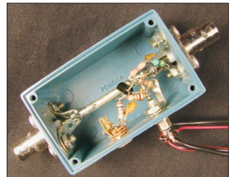
Figure 5 — A view of the dead-bug construction techniques used to build the Bias-tee.
