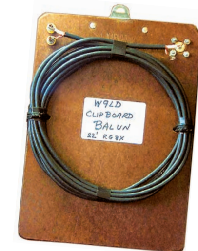
Figure 2 — The author's current balun fits on a clipboard. An SO-239 connector provides coax cable input on upper right while two banana jacks connect to window line at upper left.
