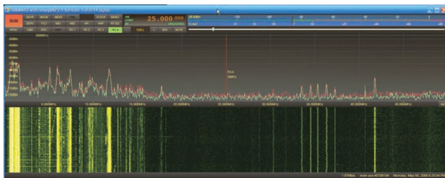
Figure 1 — You're looking at the entire RF spectrum from virtually zero all the way to 50 MHz, courtesy of a QS1R Software Defined Radio board and SDRMAXII panadaptor software.
