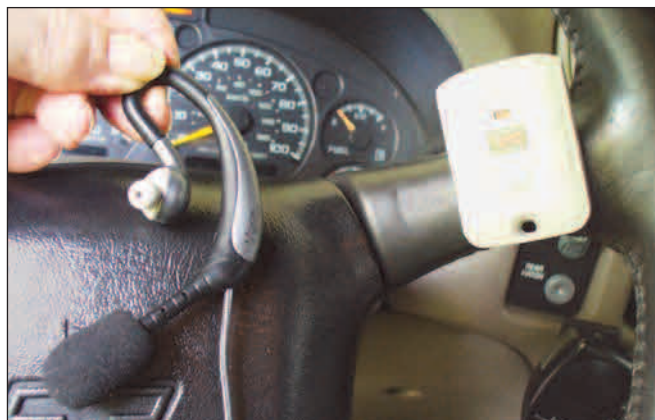
Figure 1 — Key ring size remote transmitter Velcro attached to the steering wheel.
