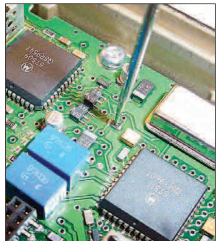
Figure 5 — Close-up of the needle keeping an SMD component in place.
