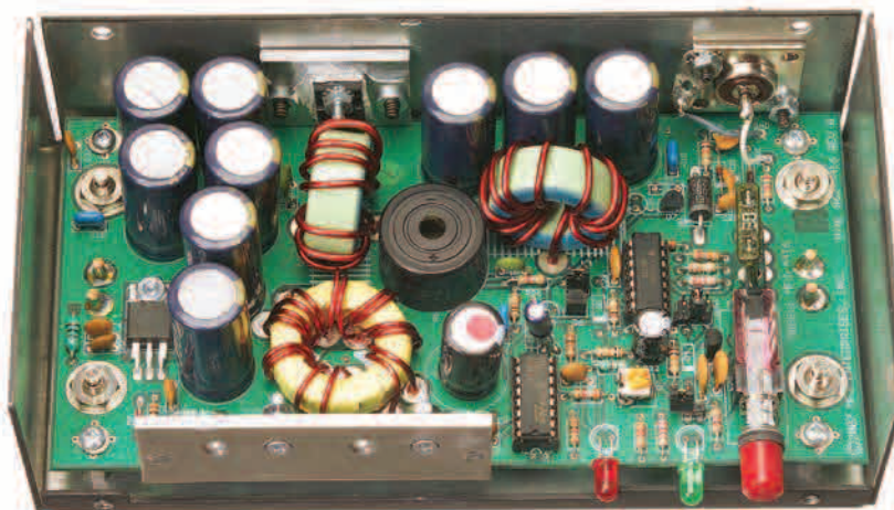
Figure 7 — Inside the MFJ-4416 Super Booster. Internal jumpers allow selection of the low voltage cutoff point and audible alarm enable/disable. The output voltage adjustment is also on the PC board.
