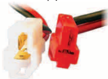
Figure 1 — Typical power connectors used on many V/UHF mobile radios. The larger housing with the spade pins is generally used on the equipment side, while the socket on the right goes to the power source.
