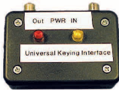
Figure 5 — Keying module installed inside a small plastic box. Two LEDs provide status of power and keying output.
