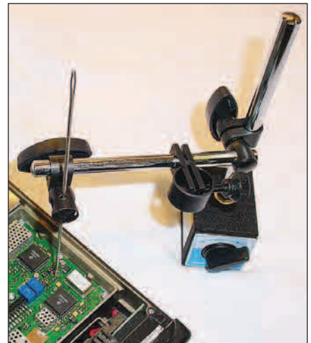
Figure 4 — The holder assembly in use on an SMD component.
