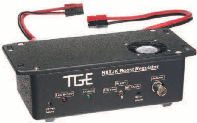
Figure 1 — The TGE N8XJK Super Booster has a small cooling fan on top, and all external controls are on the front panel. The author added Anderson Powerpole connectors to match his equipment.
