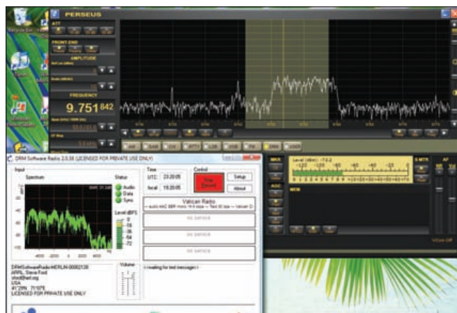
Figure 4 — Listening to a Vatican Radio DRM broadcast with commercial DRM decoding software running alongside the Perseus application.
