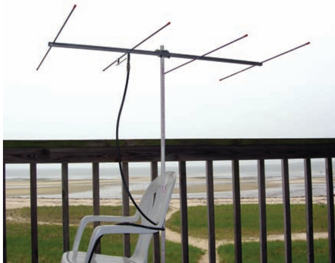
The Arrow 146-4BP Yagi perched on the author's balcony at Cape Cod, Massachusetts.
