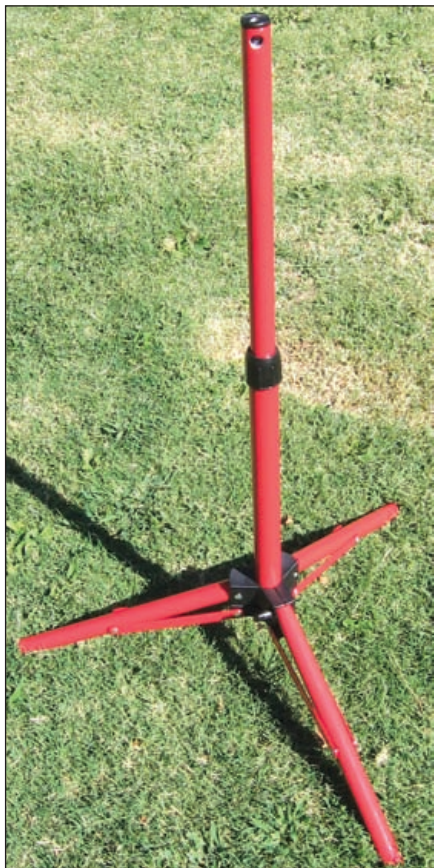
Figure 1 — The worklight tripod before the addition of the PVC leg extensions.
