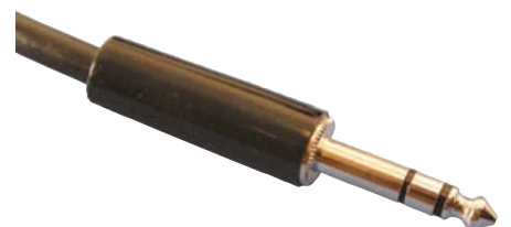
Figure 1 — Two-circuit or stereo phone plug. The connections are referred to as sleeve , ring and tip from left to right.
