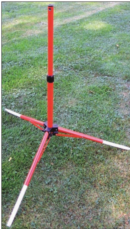
Figure 2 — The worklight tripod with the PVC legs attached.
