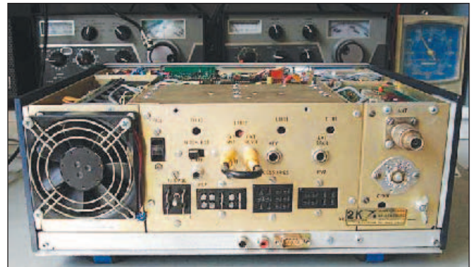
Figure 8 — TR-7 with rear extension installed.
