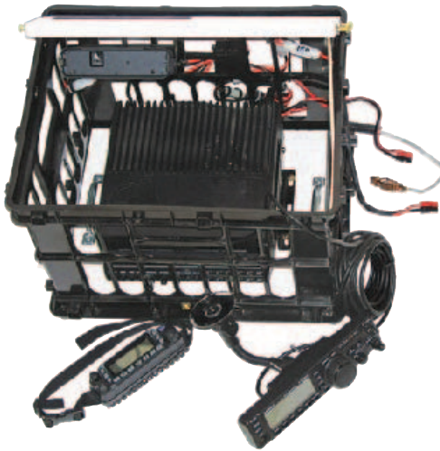
Figure 2 — Front view of crate with FT-7800 VHF/UHF chassis tilted up to show the interior. The mounted FT-900 HF transceiver chassis can be lifted out by grasping the cabinet handles.
