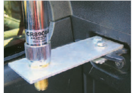
Figure 6 — Antenna mount installed on tie down.
