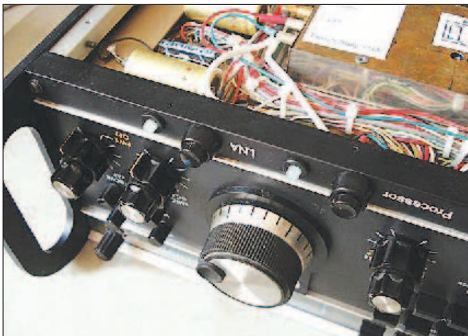
Figure 7 — Installed front panel extension, as seen from the bottom.
