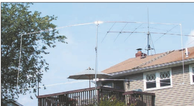
Figure 9 — Moxon pointing straight up on my test stand for initial testing. My HF roof tower with the five element 10 meter beam can be seen waiting for the antenna to be mounted.
