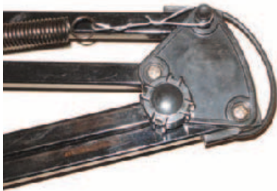
Figure 3 — The paper clips reduce the spring force by extending the springs.
