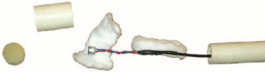
Figure 1 — Cotton padding is used to hold the mic in the tube and attenuate extraneous sounds.
