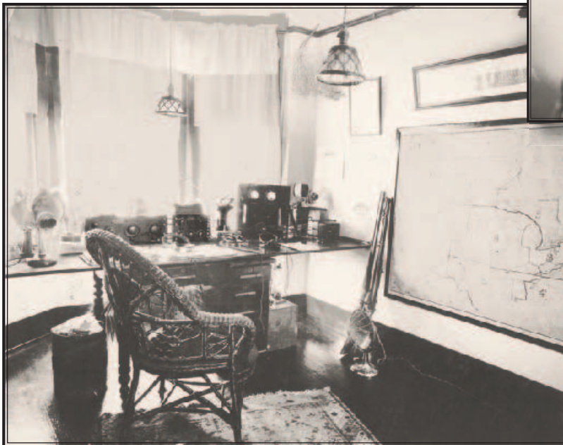
Barnsley's Station 9BP; on his desk from the left, telephone, Adams-Morgan Paragon type RA-10 receiver, Paragon type DA-2 detector-amplifier, antenna switch with hand key in front, transmitter, ear phones, open high voltage power supply with antenna tuner just above. His transmitter was the same as 6ZAC's in the May, 1922, issue of Radio magazine. Two 50 W tubes were used in a full-wave rectification circuit with 1500 V on the plates.
