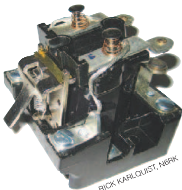
Figure 4 — The modified Potter-Brumfield PRD7AYO-24 relay showing the rear area with the tail bent to permit an increased gap between the relay contacts.
