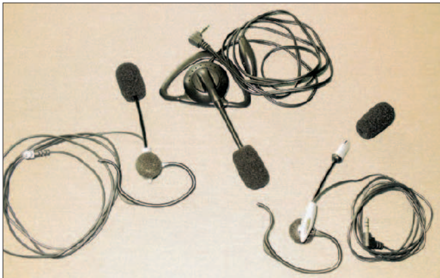
Figure 6 — Three different universal cellular headsets are shown here. One has the foam sock removed to show what it looked like when purchased. The foam sock is from Tower Electronics at www.pl-259.com . RadioShack lists this headset on their Web site for less than $20 but I have purchased them at discount stores for as little as $4.90.
