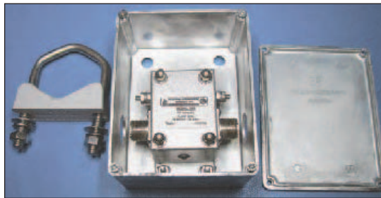
Figure 1 — The U-bolt alongside the arrestor mounted in the enclosure.
