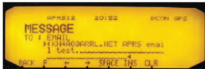
Figure 5 — I've composed a message that I want to be sent via Internet e-mail. It's very tedious to select each letter using the dial.
