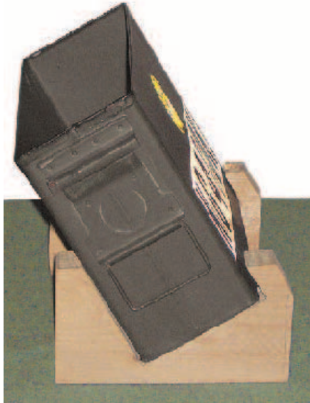
Figure 4 — Framing lumber 2 x 4 scraps were cut to make legs for the box so that it tips back around 30°.
