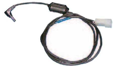
Figure 8 — Power cord for handheld was liberated from an ac supply and a Molex connector was installed to mate with 12 V battery wiring harness.
