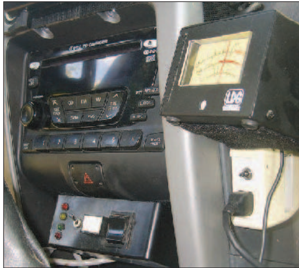
Figure 2 — The control box for part of the APRS equipment and the HF antenna control switches.
