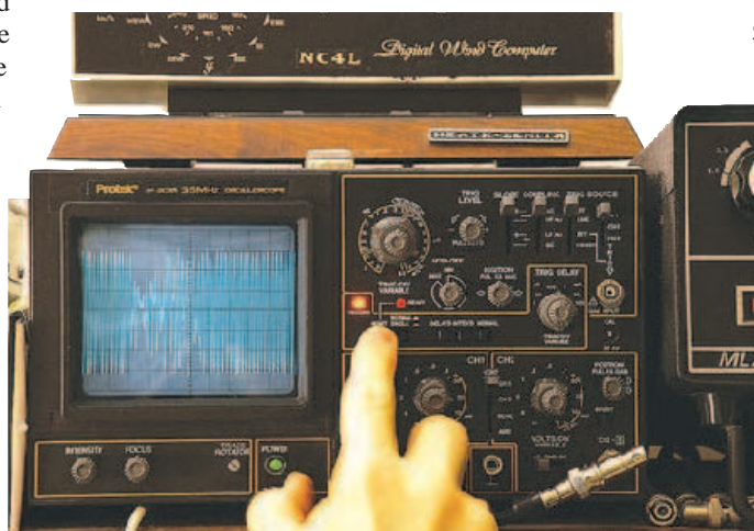
Figure 3 — Response to a brisk tap. Note that the sweep is at 5 ms per division. The disturbance persists 4 divisions and then resettles to the same level it was before the strike(s).
