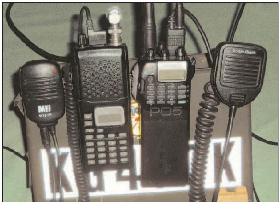
Figure 2 — Close-up of two handhelds held in place on the ammo box by belt clips.
