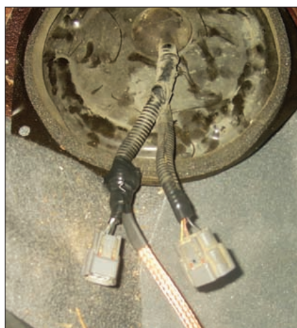
Figure 8 — Ground strap and bypass connection for the fuel pump. The strap must be long enough to attach to the passenger body.
