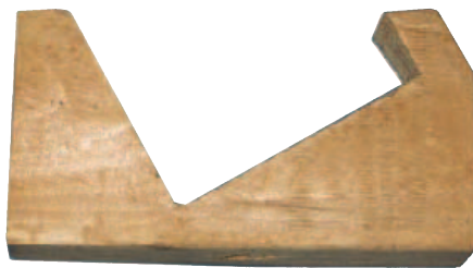
Figure 5 — Close-up of one leg cut from a piece of 2 x 4. Both legs fit inside the ammo box when not in use.
