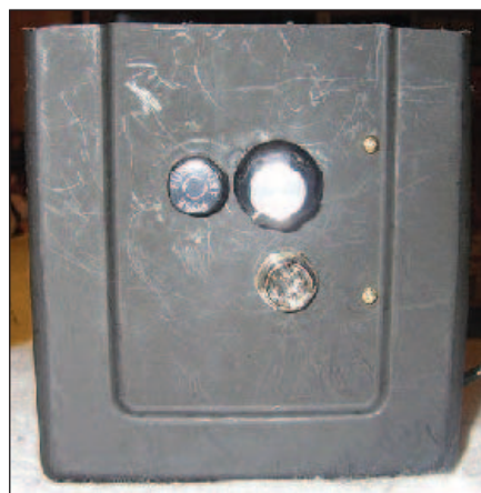
Figure 4 — “Front panel” of APRS module with external control, connector and fuse.
