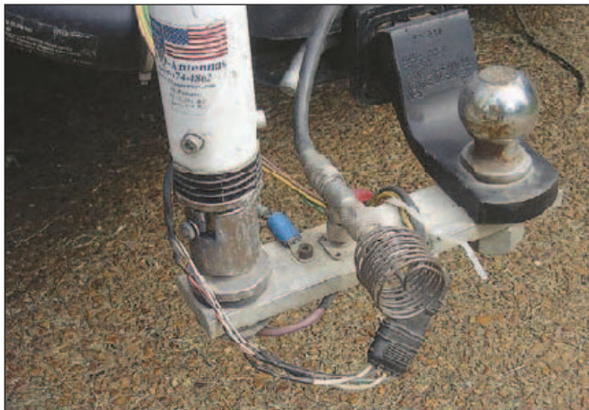
Figure 5 — The HF antenna mounted on the trailer hitch with mounting hardware from Hi Q Antennas. There is a toroid core with the motor wiring lines wrapped around it behind the mounting bar. The added shunt matching coil can be easily seen.
