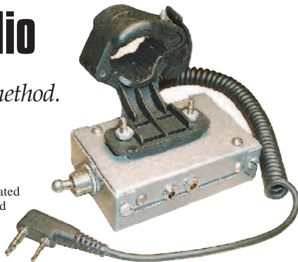
Figure 1 — Handlebar mounted transmit/receive switchbox. Two input jacks for the boom headsets are shown to accommodate different wiring schemes of the different aftermarket headsets I use.
