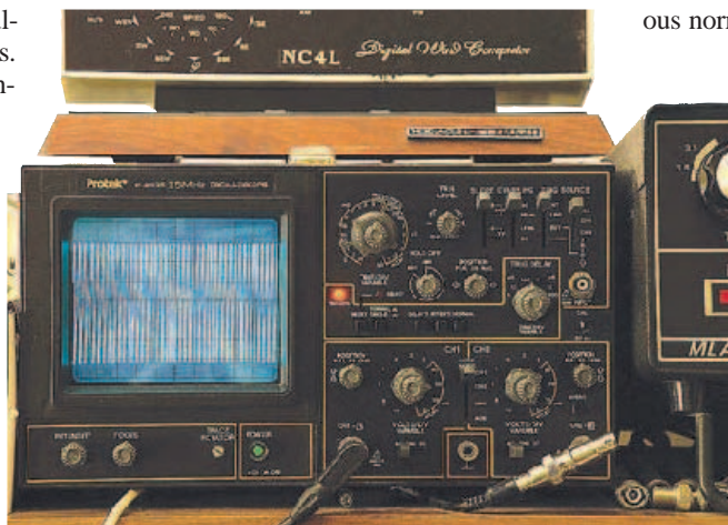
Figure 1 — An oscilloscope that is typical of those that can be purchased from eBay or at hamfests for $50 to $100. It is a dual channel 'scope with 35 MHz bandwidth — more than is usually needed.
