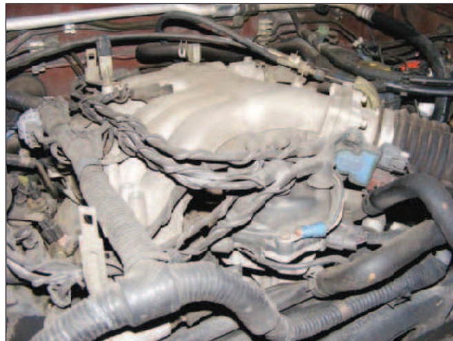
Figure 6 — Shielding wires wrapped around ignition wires to help suppress ignition noise.
