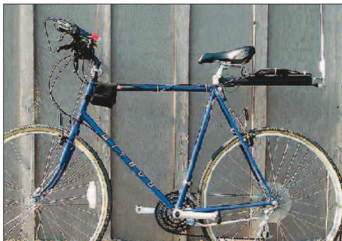
Figure 5 — The completed setup ready for action. The bottom portion of the CG-144 antenna is shown. The pouch hanging from the top tube holds a battery pack for night time riding.
