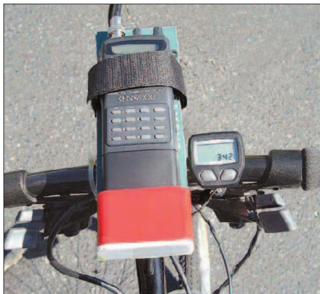
Figure 3 — The transceiver in its cradle mounted on the bicycle handlebars. (The bicycle computer to the right is unrelated to ham radio.)
