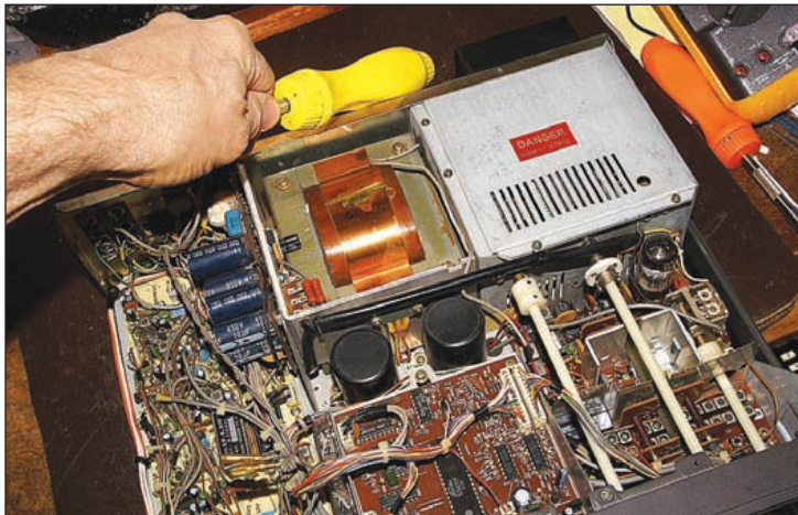
Figure 2 — Only hit the chassis hard enough to get the bounce effect (see text) on the scope pattern. In all testing use good common sense.
