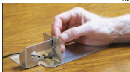
Figure 1 — This lightweight keyer paddle is held in place by the weight of the operator’s own hand. It is fabricated from two pieces of sheet metal and some snap action switches.
