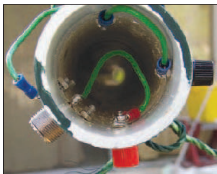
Figure 2 — Binding posts and internal wiring arrangement.
