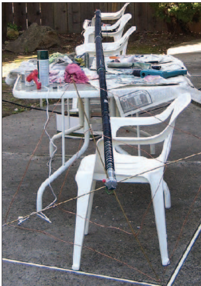
Figure 11 — Antenna fully assembled and ready to erect.
