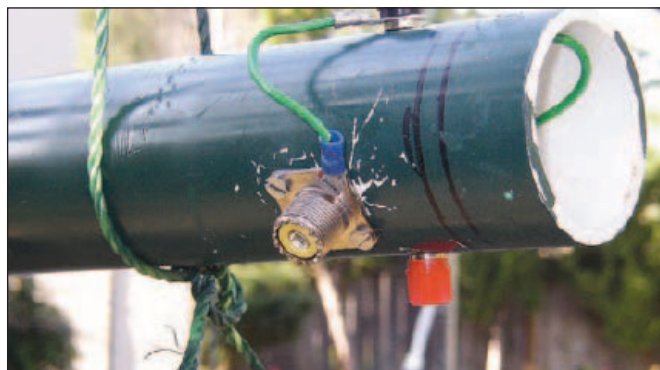
Figure 1 — Details of SO-239 UHF coax connector attachment.
