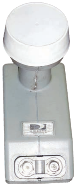
Figure 4 — Dual coax connector configured LNB. Terminate one connector with a dummy load.
