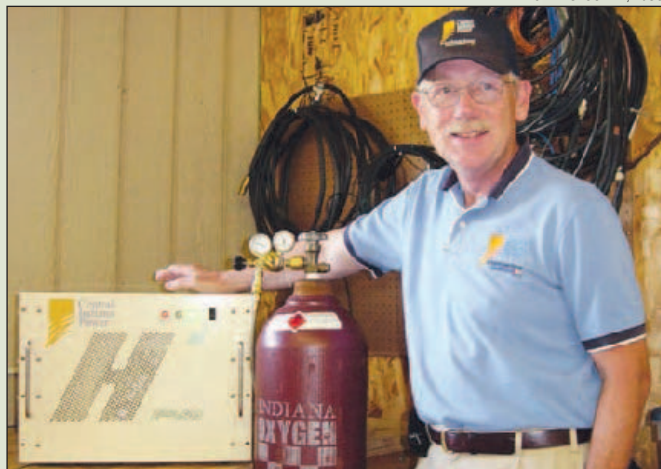
Figure 1 — Bob, W9RWP, with the H Power Epac-500 hydrogen fuel cell he won in an essay contest. The red and green LEDs indicate that it is actually running in emergency mode.
