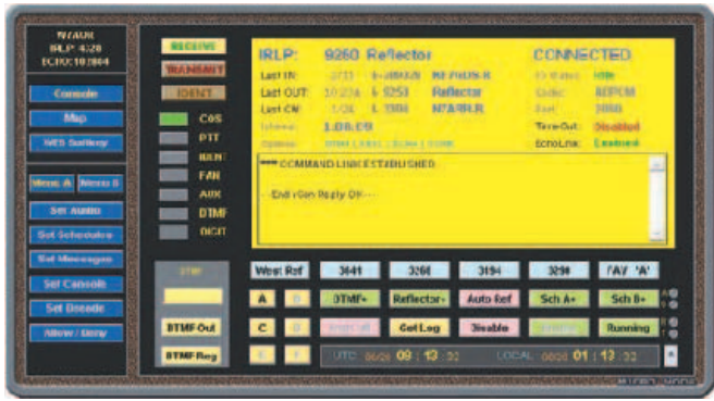
Figure 7 — The Console is the main screen for monitoring and controlling all operations.
