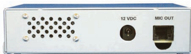
Figure 3 — Rear of cabinet showing the speaker location and the POWER and MIC OUT connectors.
