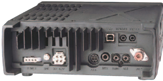
Figure 4 — The rear panel of the IC-7200 includes antenna and power connectors, ALC and TR control for a linear amplifier, provisions for digital modes and computer control.
