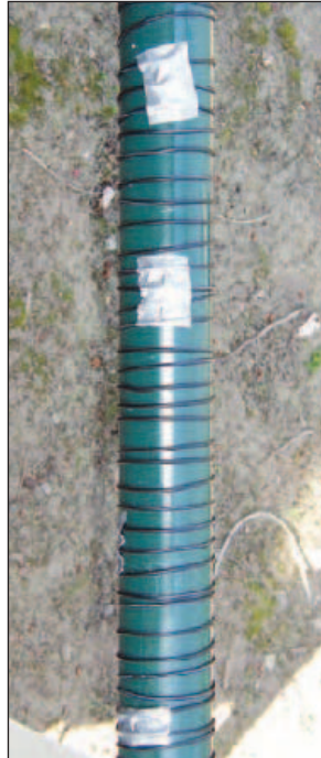
Figure 6 — Wire wrapped around pole and taped to maintain position.
