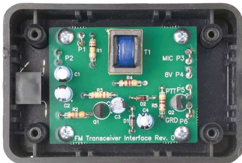
Figure 3 — A version of the VOX interface using the circuit board provided by the author.
