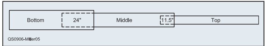
Figure 5 — Dimensions of PVC section telescoping overlap.
