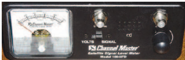
Figure 5 — CM satellite signal strength meter.
