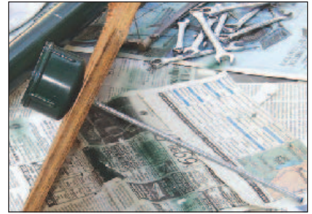
Figure 10 — View of threaded rod that will secure the antenna to the ground.
