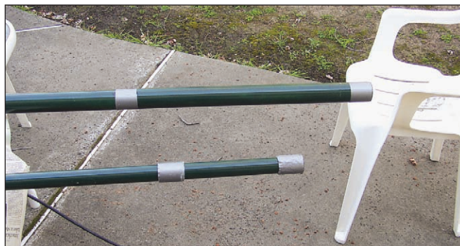
Figure 3 — PVC sections wrapped with duct tape to make a tight fit.
