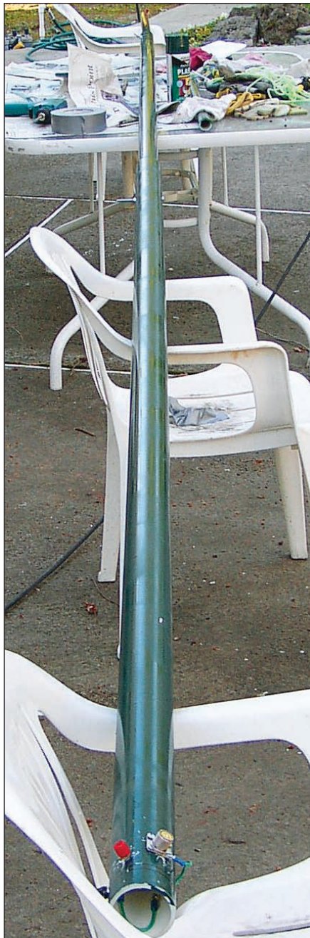
Figure 4 — PVC sections telescoped together and ready for final assembly.
