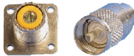
Figure 5 — UHF type connector pair; SO-239 socket on left, PL-259 plug on right. Note the four spring fingers that make the socket's inner connection.
