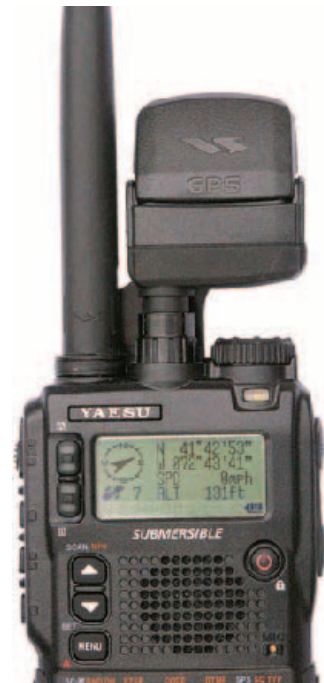
Figure 2 — The VX-8R with the FGPS-2 GPS antenna, coupled by the CT-136 antenna adapter. Note that there is ample room to turn the DIAL, thanks to its flat design. The GPS antenna can also be attached to the MH-74 speaker/mic, which then plugs into the MIC/SP jack on the transceiver.
