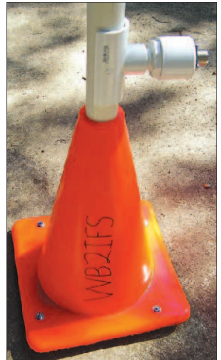
Figure 6 — The completed antenna stand.
