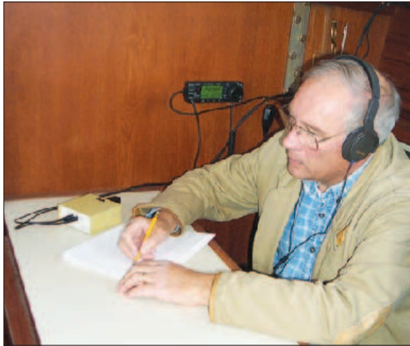
Figure 2 — Here the control head has been attached to a bracket mounted on the bulkhead adjacent to the cabin table. It makes a perfect spot for CW operation, or for contest logging.
