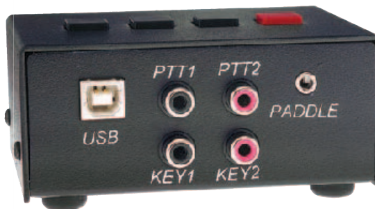
Figure 8 — The rear panel includes PTT and key connections for two radios, plus a USB jack for the computer connection and a stereo 3.5 mm jack for a paddle.
