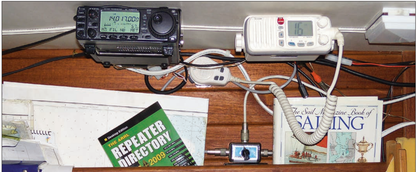
Figure 1 — The amateur transceiver is located adjacent to the VHF marine set, secured below the side deck. The small coax switch that transfers the antenna to either radio can be seen on the right.
