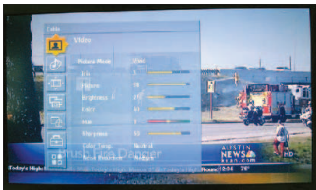
Figure 1 — The dreaded flashing menu flavor of TVI.
