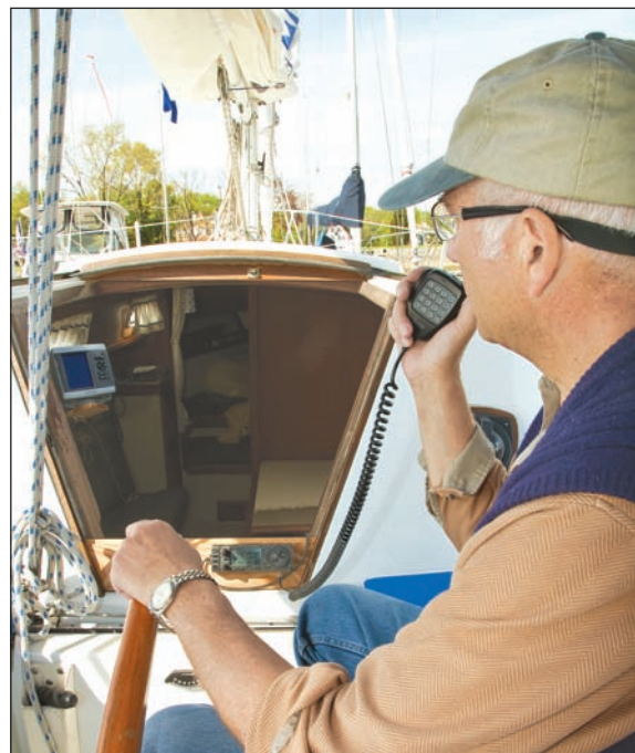
Figure 3 — A bracket is mounted to a board cut to fit in place of the lowest companionway drop board. With this arrangement, I can operate while underway. Once contact is established, hit the LOCK button or you will be sure to knock the tuning knob while you multitask!
