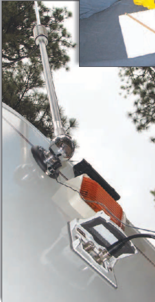
Figure 4 — The Buddistick and external antenna connections mounted on the outside of the trailer.
