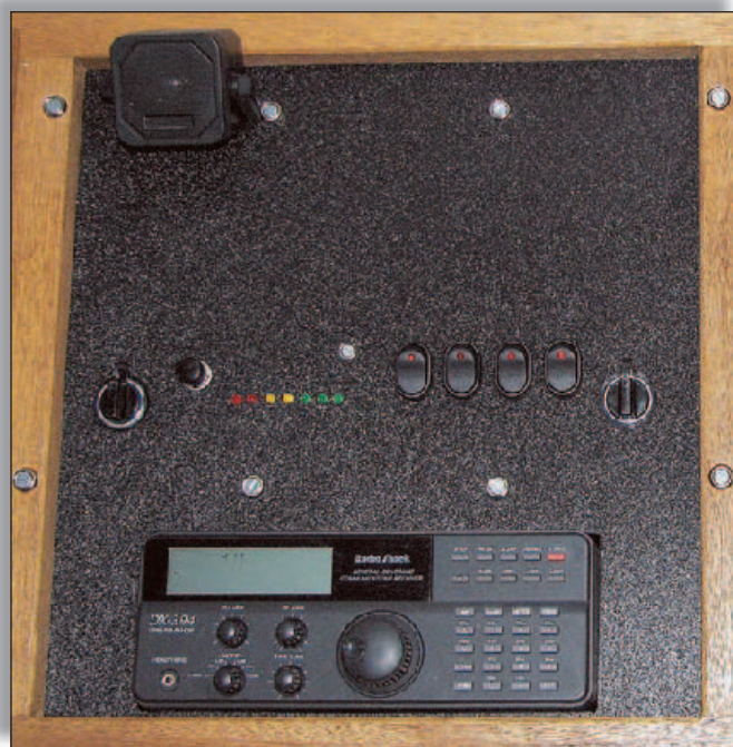
Figure 3 — The homebrewed receiver panel with various accessories and a speaker.
