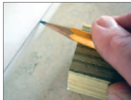
Figure 3 — Scribing a straight reference line along the mast is critical.
