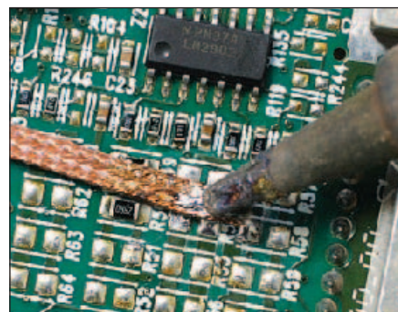
Figure 3 — Remove the excess solder and flux from the board with solder wick. Additional scrubbing with a swab and alcohol will remove the flux residue.
