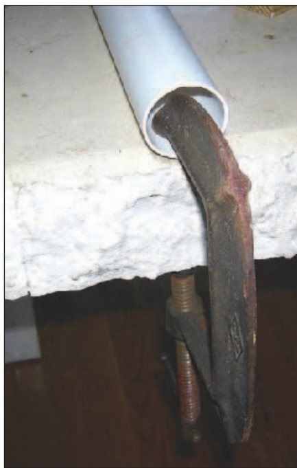
Figure 2 — Clamping the mast to a table keeps it stable as you are marking hole locations.
