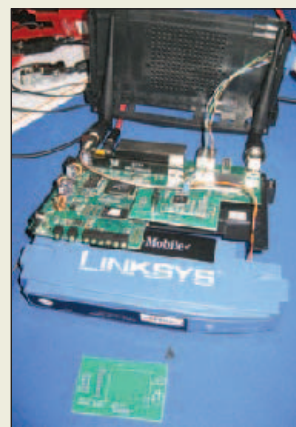
Chris Kantarjiev, K6DBG, demonstrated APRS (Automatic Position Reporting System) gear that he has collected and built. He modified this Linksys router (WRT54 series) to support a small internal TNC that exchanges data with the router using an unpopulated internal serial port. The reconfigured device connects easily to a radio to operate as an iGate digipeater. For this project, Kantarjiev selected the small “OpenTracker” kit produced by Argent Data Systems to configure the device to support APRS.
