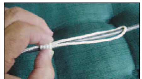
Figure 3 — Wind the end of the rope around the 5 inch loop in tight turns.
