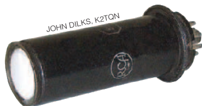
Figure 1 — RCA 913 tube, about the size of a metal 6L6 tube.
