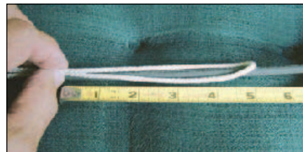
Figure 2 — First, form a 5 inch loop.
