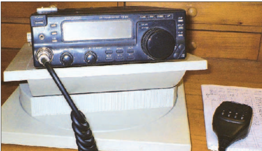
Figure 7 — The completed stand with the rig in place.
