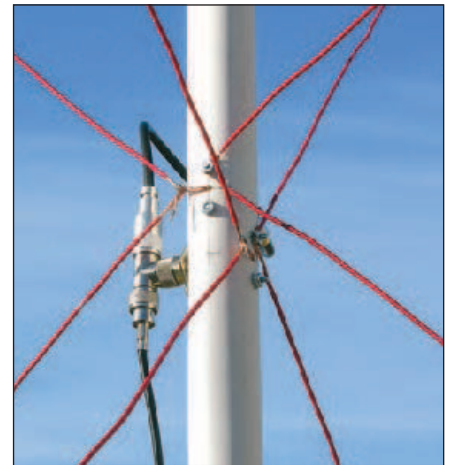
Figure 5 — A close-up view of the phasing line and wire terminations with the T adapter visible.
