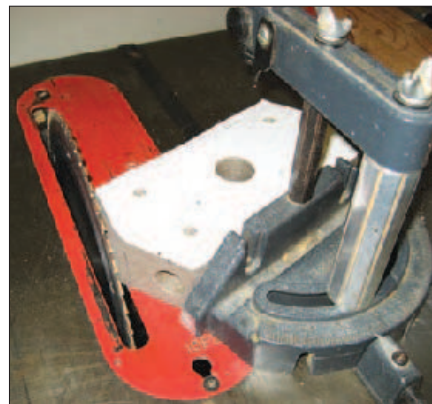
Figure 3 — Preparing a hub on a table saw using a printed template.
