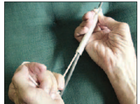
Figure 5 — Finally, pass the knot through the remaining loop and pull the end of the rope to close the loop below the knot.
