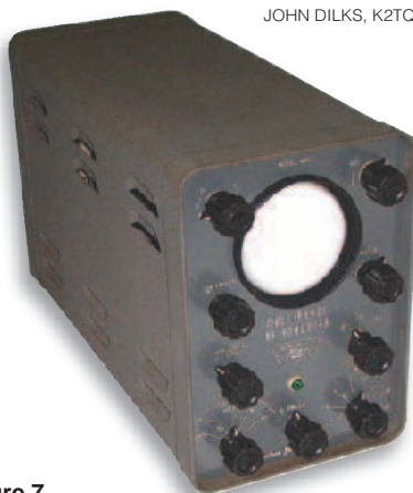
Figure 7 — Central Electronics Multiphase MM2 RF Analyzer.
