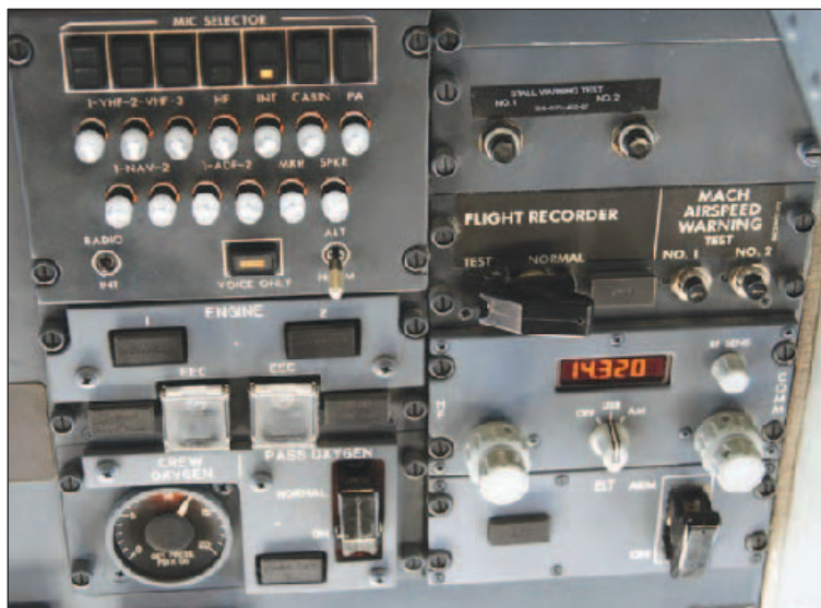
The HF station used aboard the Boeing 737-800 is a Collins HFS900D with 400 W PEP coupled to an automatic antenna tuner (bottom right).
