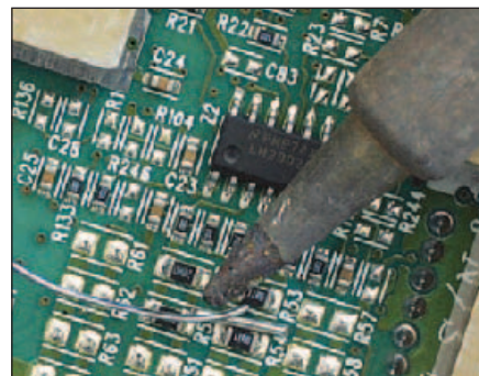
Figure 2 — As the component heats and solder begins to reflow, quickly add more solder to flood the component area. The component will float and you can flick the iron tip to push the component off of its pads.
