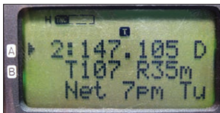
Figure 3 — For travelers, APRS radios display the locally recommended voice frequency object that includes the tone, range and net times as shown here on a TH-D7.
