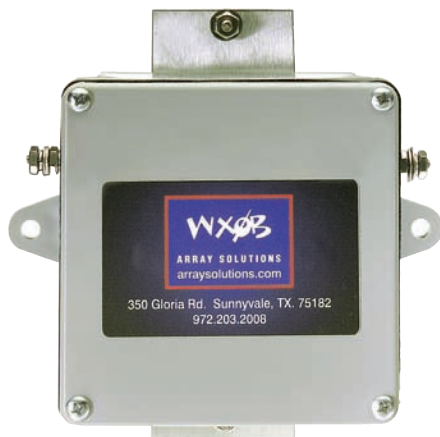
Figure 9 — The ATD-1 is also housed in a weatherproof NEMA enclosure and is slightly larger than the Bias-T units. The two screw terminals are for connection between the autotuner and antenna, and the metal plate on the back attaches to ground. There's a coaxial jack for power on the left side.
