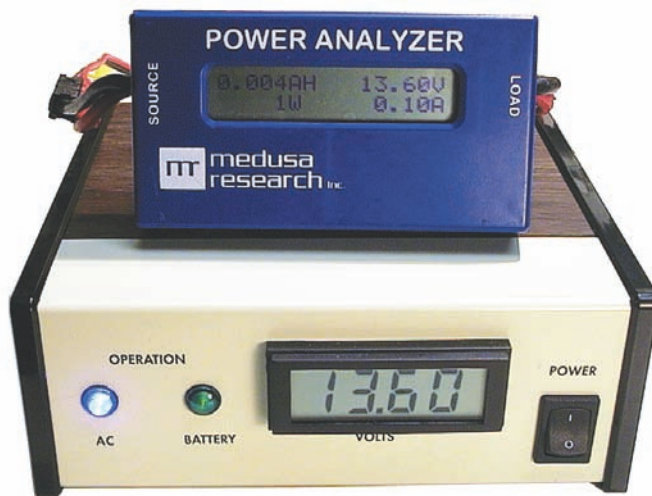
Figure 5 — Here's the charger buttoned up and put to use. The power analyzer shows the voltage to be tracking right on the money. The battery is being charged at a 100 mA rate.
