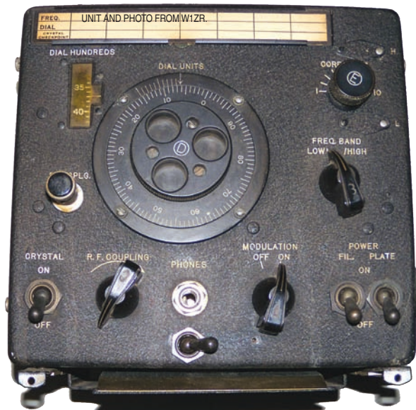
Figure 8 — An LM heterodyne frequency meter from the WW2 era. Each line represents 1 kHz at the fundamental range (2 to 4 MHz).
