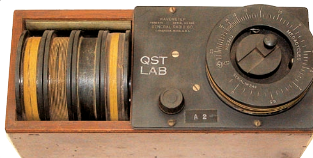
Figure 2 — General Radio 574 wavemeter, c 1930s, from the ARRL Lab collection. The left side includes inductors for different bands that are positioned on the top as shown to measure within each frequency range.
