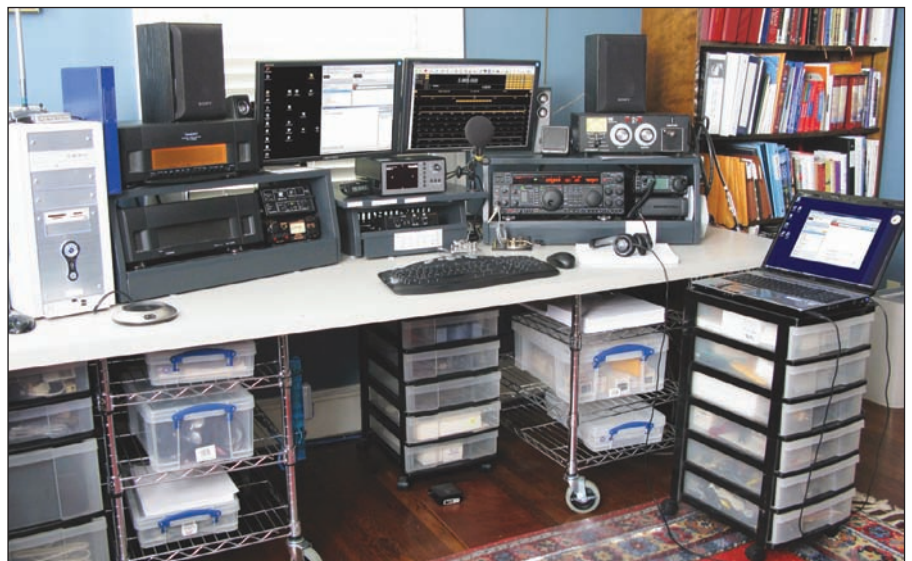
Figure 2 — The W4UOA operating position with the Skype software running. The laptop is handling the conference controller function while the base station computer is providing the interface to the transceiver
