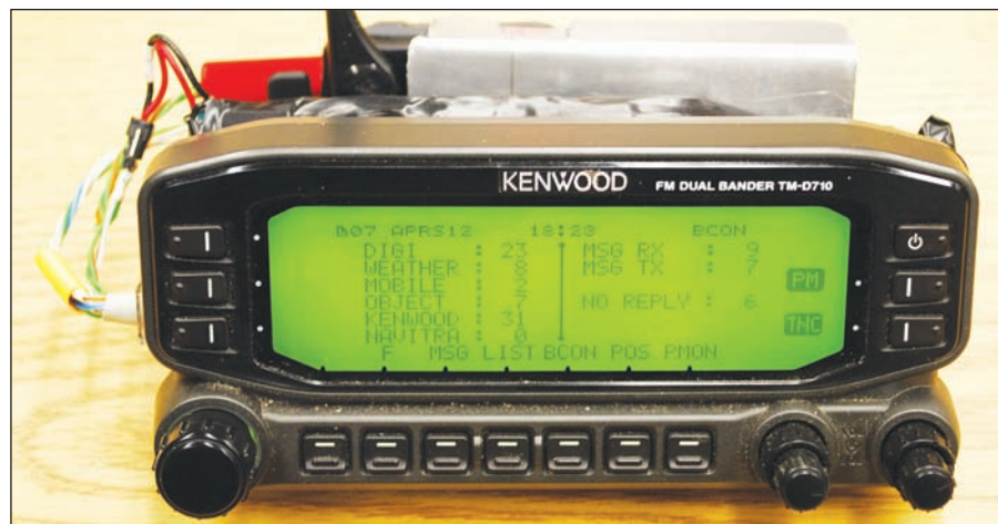
Figure 2 — The Kenwood RC-D710 APRS display head can be purchased separately from the TM-D710 radio and can be plugged into the external audio interfaces of any radio. All of the APRS hardware and functionality is in the display head itself. Here it is shown connected to an Alinco handheld transceiver to provide front panel APRS, text-messaging capabilities and e-mail to the operator.
