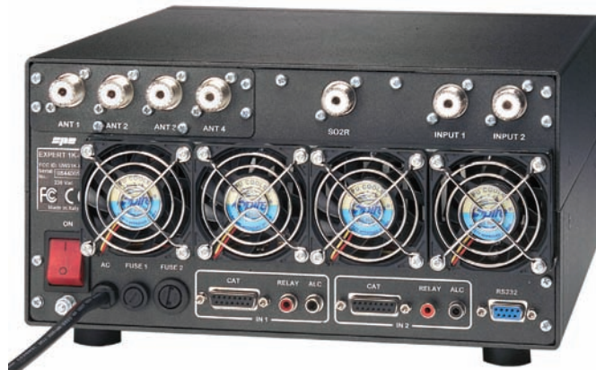
Figure 2 — The rear panel includes connections for two radios and up to four antennas. The four cooling fans, plus three more inside the case, remove heat effectively.
