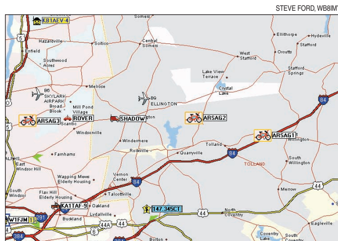
Figure 2 — A glimpse of Angel Ride APRS activity with UIView software. Notice the three bike mobiles designated ARSAG, along with the ROVER and SHADOW mobiles.
