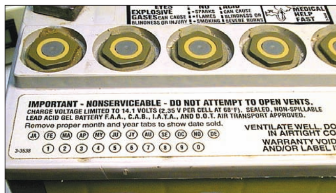
Figure 1 — An example of the labeling of a gel cell battery. Sometimes the battery itself will have the necessary information on how it should be charged. In this example, they state a maximum of 14.1 V. Notice the "fill caps" are actually vents and not removable caps. This DeKa from East Penn Manufacturing is a true gel cell battery.
