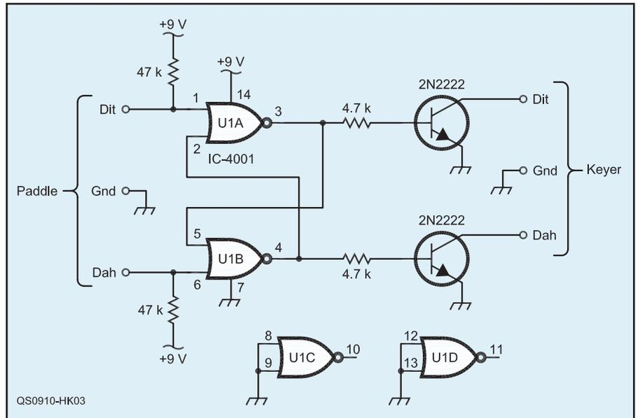
Figure 3 — The multivibrator circuit to make an iambic paddle act like a single paddle key.
