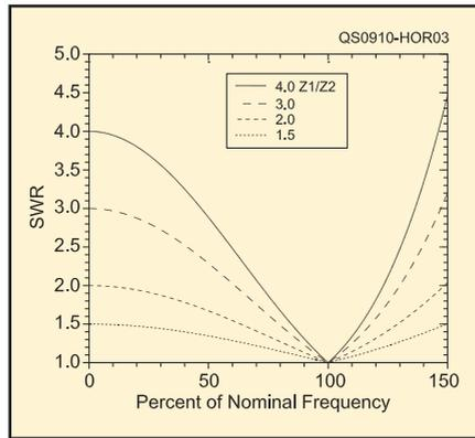
**Figure 3 — The bandwidth of the  $\frac{1}{2}$  wavelength transformer. The resulting SWR for frequencies from dc to 1.5 times the design frequency and resistive impedance mismatches up to 4:1 (from Note 3).**
