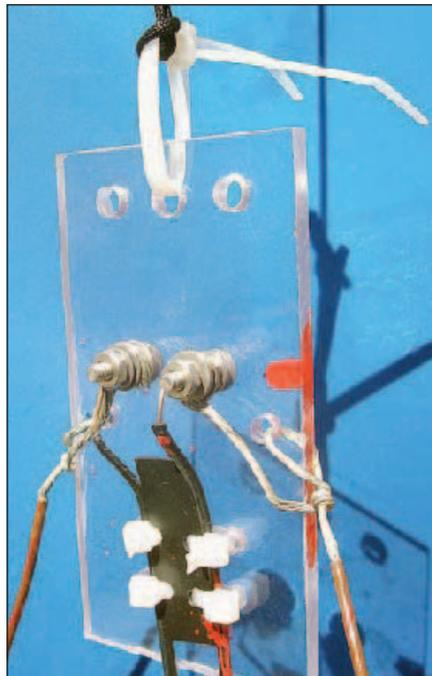
Figure 4 — Antenna center insulator ready to be hoisted up.
