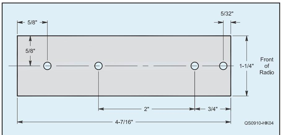
Figure 4 — Mechanical layout of the adapter bracket.
