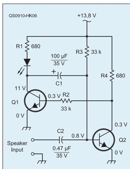
**Figure 6 — The circuit for the receive indicator.**
