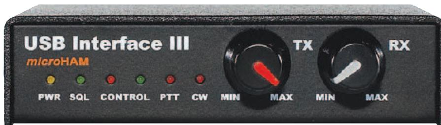
The microHAM Interface III includes its own sound device and provides radio control capability.
