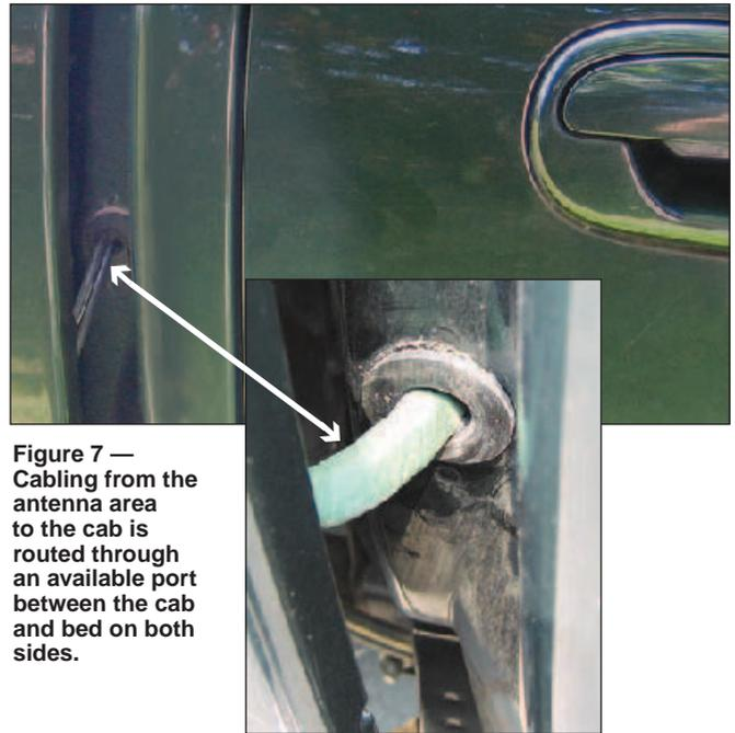
**Figure 7 — Cabling from the antenna area to the cab is routed through an available port between the cab and bed on both sides.**
