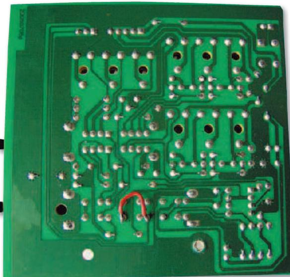
**Figure 1** — By adding a short jumper wire across the 4th and 6th bottom pins of the AVG/PEP switch, M0BOL modified his Daiwa CN-801 HP HF/VHF wattmeter to display average reflected power while reading forward PEP.
