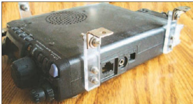
Figure 5 — Mobile radio mounting bracket made from 0.188 inch thick material. The upper angle brackets swivel to accommodate possible mounting surface curvatures, such as found on a vehicle dashboard.
