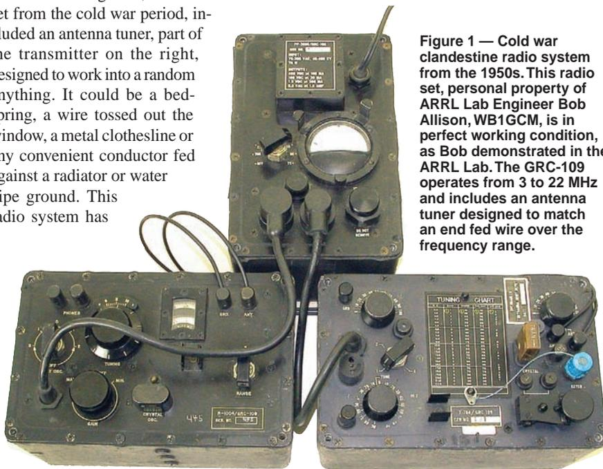
**Figure 1 — Cold war clandestine radio system from the 1950s. This radio set, personal property of ARRL Lab Engineer Bob Allison, WB1GCM, is in perfect working condition, as Bob demonstrated in the ARRL Lab. The GRC-109 operates from 3 to 22 MHz and includes an antenna tuner designed to match an end fed wire over the frequency range.**
