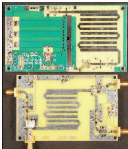
Figure 5 — Transverter board for 1296 MHz with 1152 MHz local oscillator board above it.
