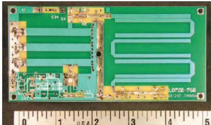
Figure 2 — Local oscillator board for multi-band transverters. Oscillator and dc wiring on reverse side.
