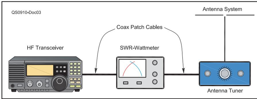
Figure 3 — KG4UDL configuration of transceiver and external wattmeter and antenna tuner.
