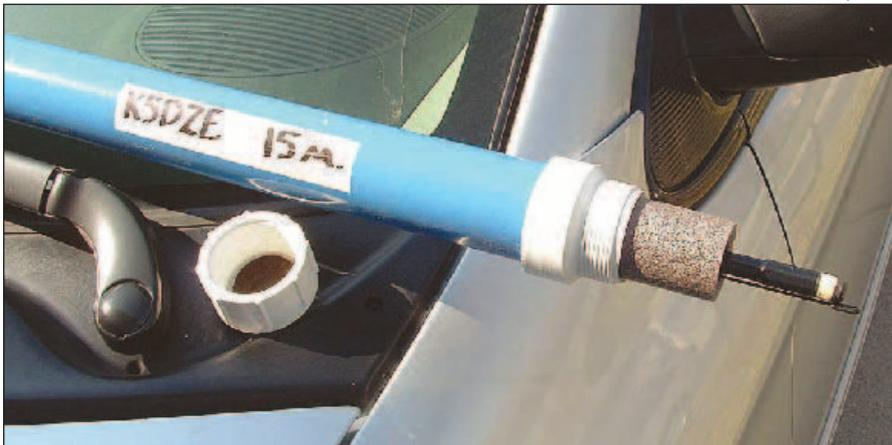
Figure 1 — A completed travel tube for a 15 meter Hamstick.
