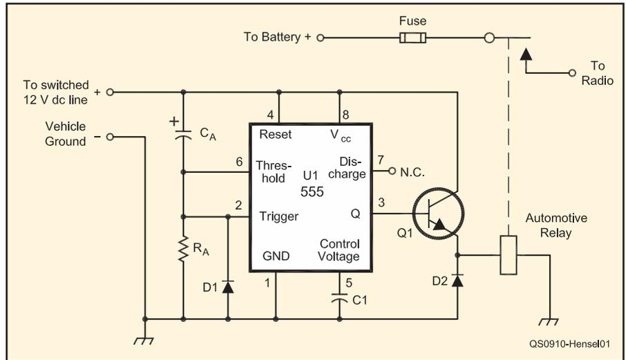
Figure 1 — Schematic diagram and parts list for transceiver protection circuit. Digikey parts are available at [www.digikey.com](http://www.digikey.com).
