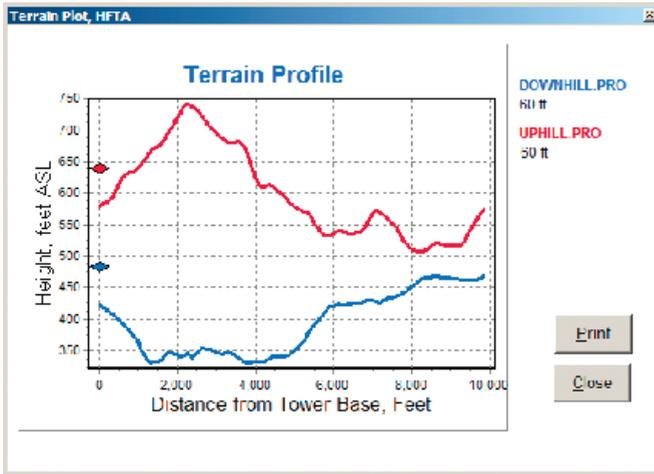
Figure 2 — Two terrain profiles towards Europe, one uphill (red) and one downhill (blue).
