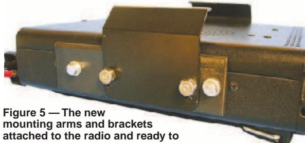
**Figure 5 — The new mounting arms and brackets attached to the radio and ready to slide into the truck's mount.**
