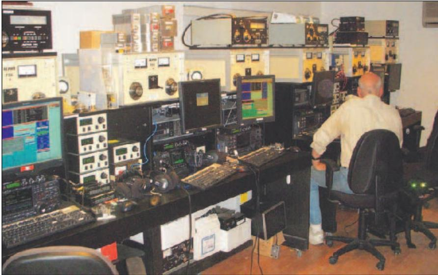
**Figure 2 — The war room at NR5M. Two of the single-band stations. Each includes a separate transceiver and amplifier for running and sweeping. All stations are networked to share log information. This is the nerve center and front line for the NR5M team's radiosport action.**
