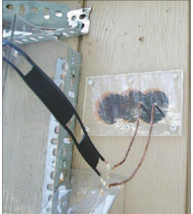
**Figure 7** — A 0.25 inch thick plastic window centers the conductors of parallel line in the feed through holes.
