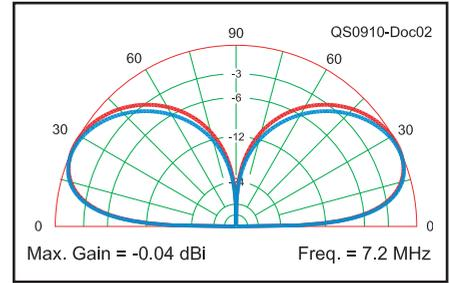
**Figure 2 — Comparison of elevation patterns of a 43 foot (blue) and 33 foot (red) vertical on 40 meters.**
