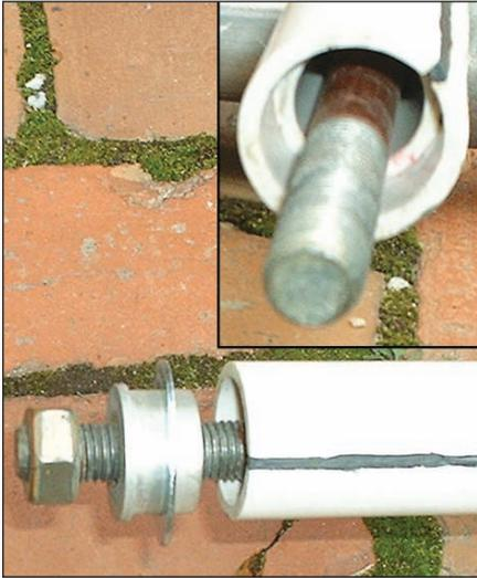
Figure 2 — The assembled components ready to be tightened onto the insulator.
