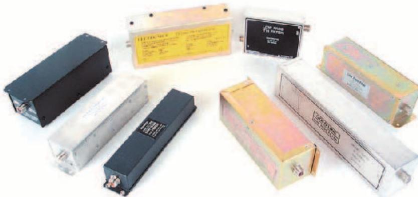
Figure 4 — Assortment of typical low pass filters — not as important as they once were.
