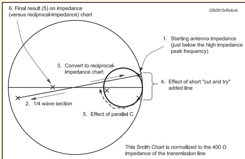
**Figure A — Simplified Smith Chart illustrating matching mechanics as the impedance is transformed through a  $\lambda/4$  section of mismatched line.**
