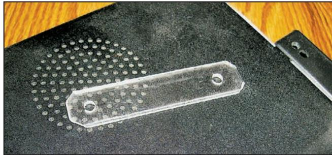
Figure 3 — Antenna end insulator made from 1 inch wide by 0.063 inch thick material. The hole edges are chamfered.
