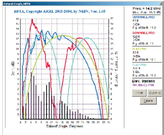
Figure 5 — Over downhill sloping ground, it is quite possible for an antenna to be too high. Here, the 120 foot high Yagi is inferior to the 60 foot high Yagi because of the effects of sloping ground. On the other hand, comparing the Figure of Merit numbers for flat ground would favor the 120 foot over the 60 foot height.
