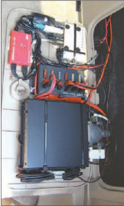
**Figure 3 — V/UHF transceiver body, RIGrunner and digital accessories all mounted on cargo door.**
