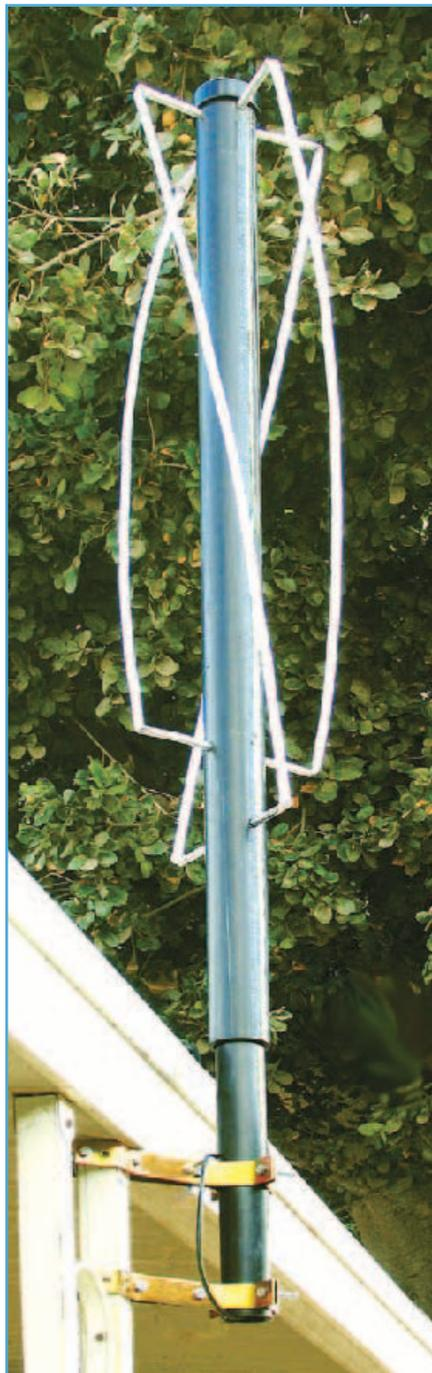
loops. Next, twist both loops horizontally a quarter turn into helices. Finally connect the feed points in parallel. Voilà — you have a quadrifilar helix antenna.
