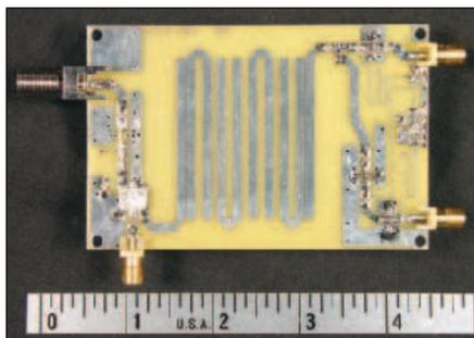
Figure 4 — Transverter board for 902 MHz with four-section printed hairpin filter.
