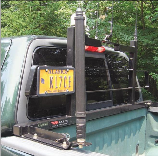
**Figure 6 — Antenna mounting details. Note the positions for an HF antenna above the side rail and VHF and UHF antennas on the upper support.**
