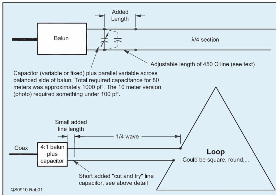
Figure 1 — Details of the matching network arrangement for the two band loop antenna.
