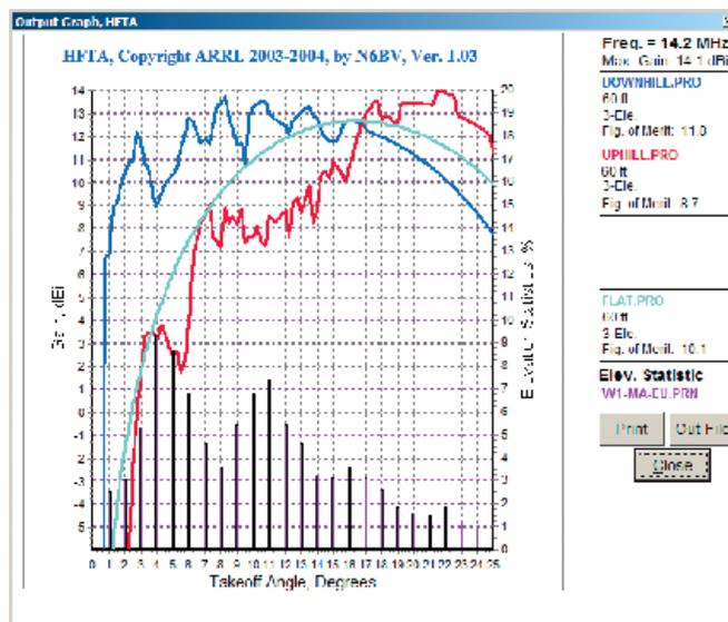
Figure 3 — Comparison of elevation-angle responses at 14.2 MHz towards Europe from New England for uphill (red) and downhill (blue) terrain profiles for 60 foot high, 3 element Yagis. For reference, the response over flat ground is also shown (cyan).
