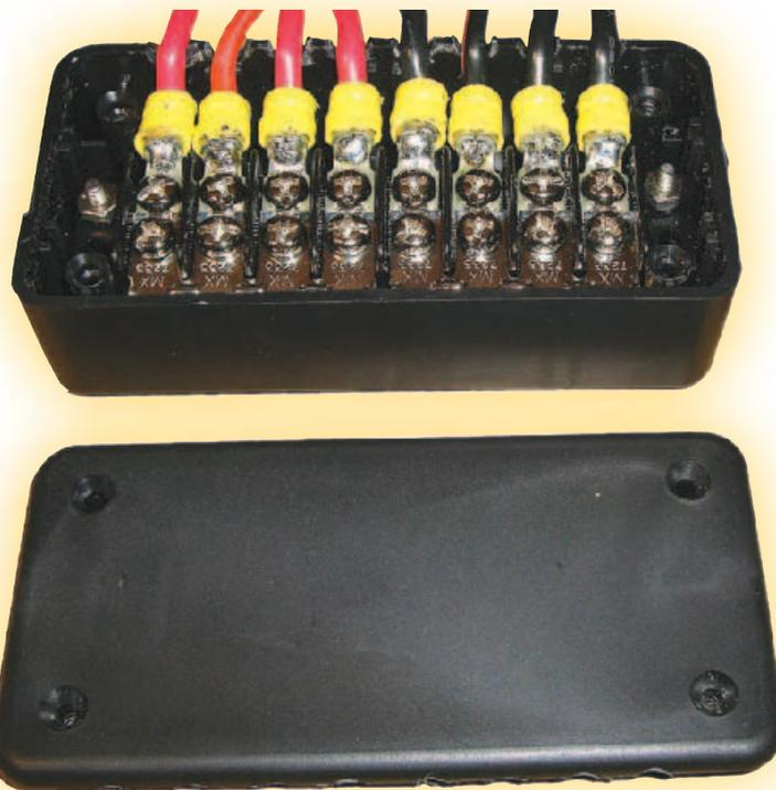
Figure 1 — The completed distribution box. Note that the terminals are secured by the edge of the (covered) box as well as by the screw.
