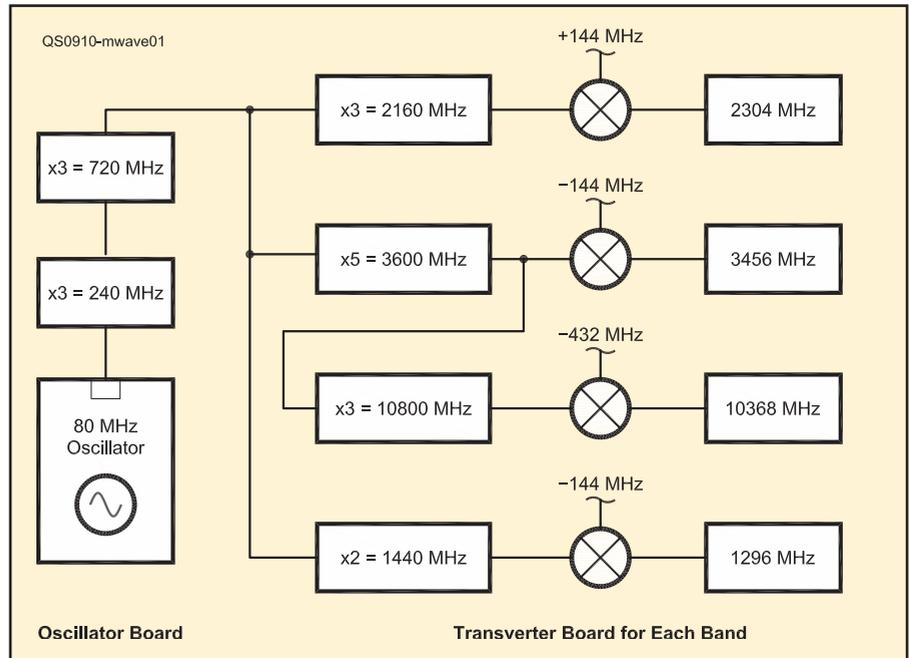
Figure 1 — Multi-band frequency scheme.
