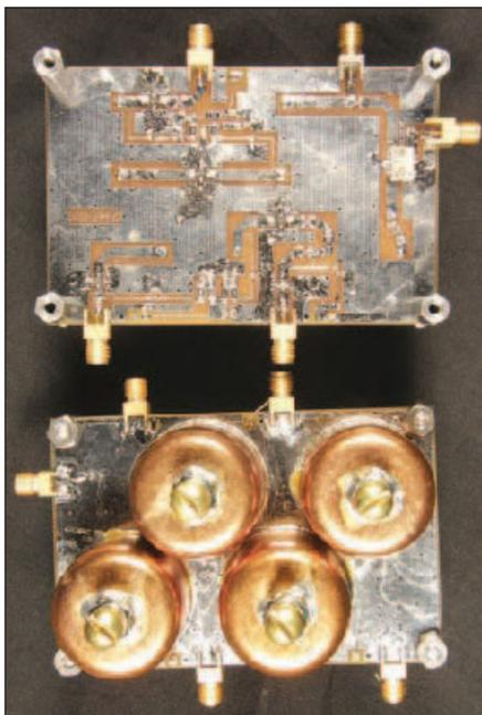
Figure 3 — Transverter board for 2304 or 3456 MHz, showing pipe-cap filters on reverse side.
