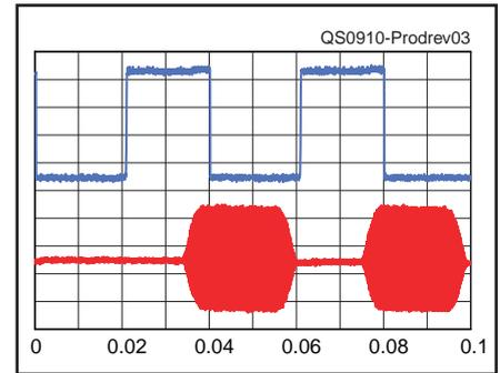
**Figure 3 — CW keying waveform for the FLEX-3000 showing the first two digits in full-break-in (QSK) mode using external keying. Equivalent keying speed is 60 WPM. The upper trace is the actual key closure; the lower trace is the RF envelope. (Note that the first key closure starts at the left edge of the figure.) Horizontal divisions are 10 ms. The transceiver was being operated at 100 W output on the 14 MHz band.**
