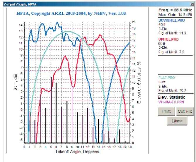
Figure 4 — Comparison of elevation-angle responses at 28.5 MHz towards Europe for 60 foot high, 3 element Yagis.
