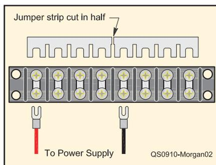
Figure 2 — Details of cutting jumper strip making the left four sets of terminals interconnected for positive connections, and the right four for negative.
