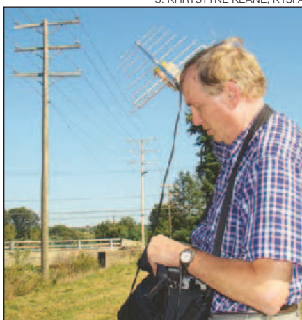
ARRL Lab Engineer Mike Gruber, W1MG, locates some harmful interference radiating from a power line.
