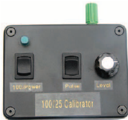
Figure 4 — The handy signal source and test generator. I installed a solid state version of the calibrator inside a small plastic box. I wire the jumpers to switches so I could control the calibrator without opening up the box. A green flashing LED keeps me mindful when the power is on. The whole shebang runs on four AA batteries.
