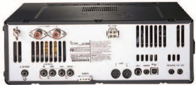
Figure 2 — The rear panel of the IC-7600 includes all the usual connectivity as well as the new USB jack for control and audio signals.
