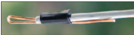
Figure 9 — An example of the temporary method to lengthen the elements is shown. A piece of #14 AWG wire is taped to the element to make a cross section approximating the diameter of the element.
