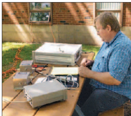
Figure 4 — ARRL Laboratory Engineer Bob Allison, WB1GCM, recording baseline data with test instruments and back-to-back baluns.
