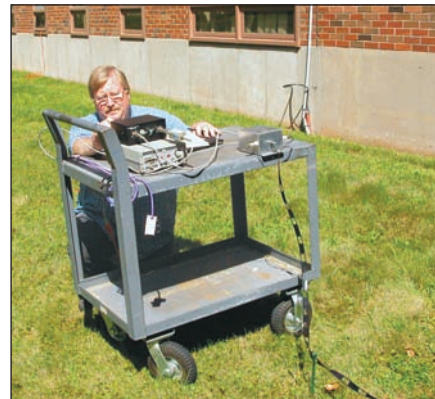
Figure 5 — WB1GCM adjusts the tuner for maximum signal into the microvoltmeter. Results were also taken with the tuner out of the circuit.
