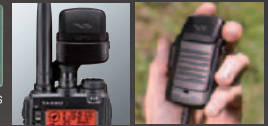
*Attached to the radio (microphone input) using the optional GPS Antenna Adapter CT-136 *The optional GPS Antenna Unit FGPS-2 attached to the optional Speaker/Microphone Adapter MH-74A
