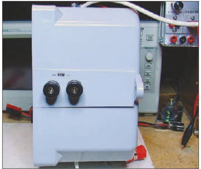
Figure 4 — 80 meter coil shorting jacks.
