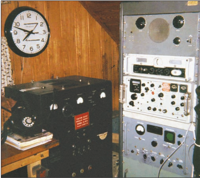
K2TQN's RTTY station in his Hampton, Virginia home. From left: BC-610-I, FRR23 receiver, CV-89 RTTY converter and miscellaneous equipment.
