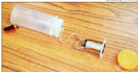
Figure 3 — An exploded view of the spice jar power adapter.
