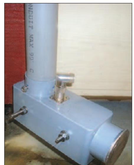
Figure 4 — View of the antenna base. Note the stud that will connect to the ground system.
