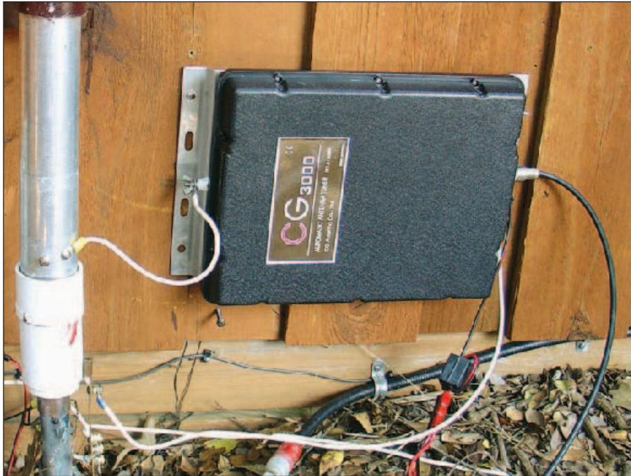
Figure 2 — Each auto tuner was tested at the base of the author's 43 foot vertical antenna.
