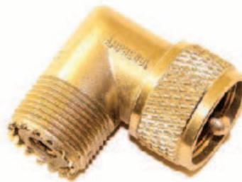
Figure 1 — Amphenol UG-646/U UHF type right angle coaxial adapter. Such an adapter can make it easy to move equipment close to walls, but use only good quality components.
