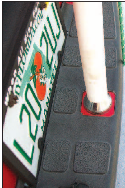
Figure 2 — The bottom end of the PVC pipe slips over my trailer hitch stud. It could easily be a regular bolt and nut through the bumper if one does not have a tow hitch on the vehicle.
