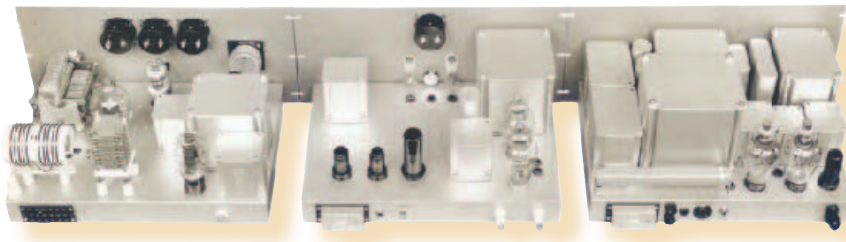
Inside the TEMCO 100-A NYA kit, from the left: RF exciter with low voltage power supply, speech amplifier-modulator unit, high voltage and C bias supply.
