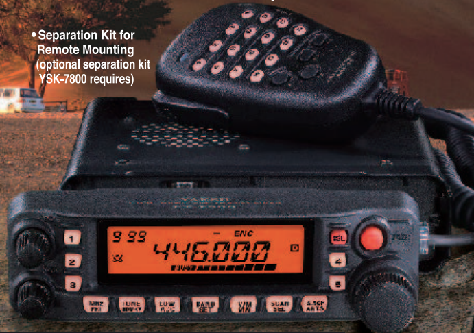
50 W 2 m/70 cm* DUAL BAND FM TRANSCEIVER *70 cm 45 W FT-7900R Size: 5.5" (W) x 1.6" (H) x 6.6" (D) / Weight: 2.2 lb
