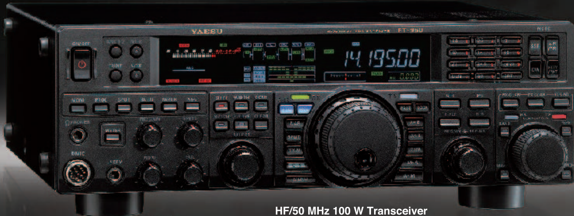
HF/50 MHz 100 W Transceiver FT-950
