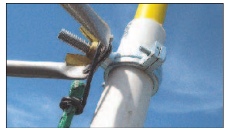
Figure 4 — The braces attached to the PVC pipe via the pipe clamp. The bungee cord connects to the rear bumper of the vehicle to exert downward force keeping the mount in place.
