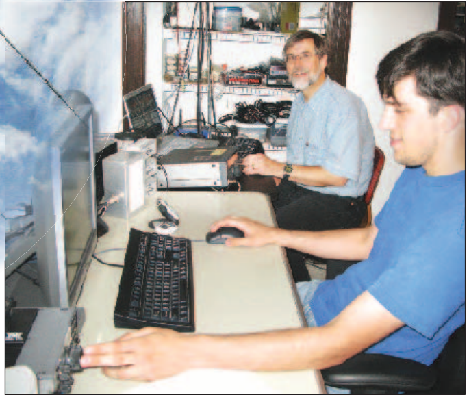
Figure 1 — Kenneth Finnegan, W6KWF, in foreground and Phil Verinsky, W6TQG, at Phil's station, competing in the July 2009 NAQP contest in the multioperator two transceiver category. Using the triplexer standing on the table between them, Kenneth and Phil operate on both 20 and 15 meters sharing Phil's triband antenna.
