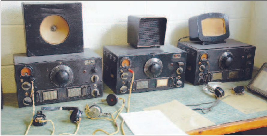
Three of the famous National HRO radio receivers whose superb selectivity made them ideally suited to intercept German wartime Morse code communications.
