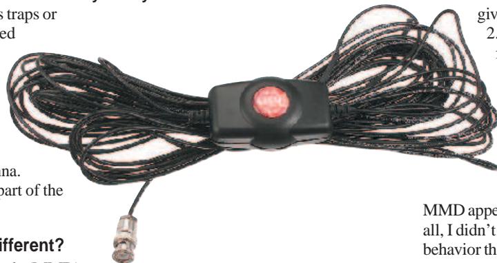
The feed point of the MMD-20 under test in my back yard.
