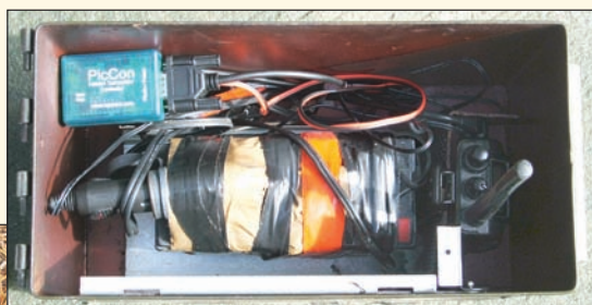
The inside of the ammo can fox box. The transceiver is clipped on the added interior support to the left. The 12 V battery and wiring harness is in the center, while the PicCon controller is in the upper left hand corner.
