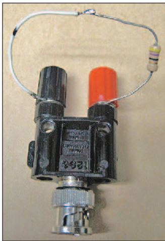
Figure 2 — Here is a close-up view of the 47 \Omega resistor in the test fixture.
