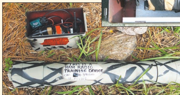
The ammo can, with lid removed, and PVC fox box containers. They are both painted to blend in to the environment, but are both marked with identification and contact number. The electronics fit in either container with room for air flow.
