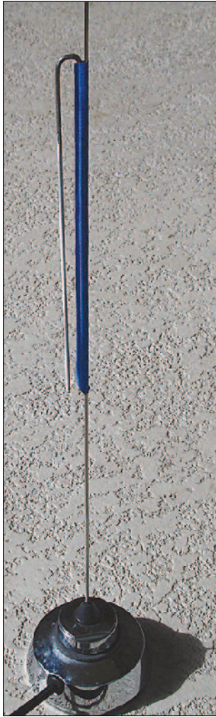
Figure 4 — The modified 2 meter whip with the hairpin taped in place on the antenna element.
