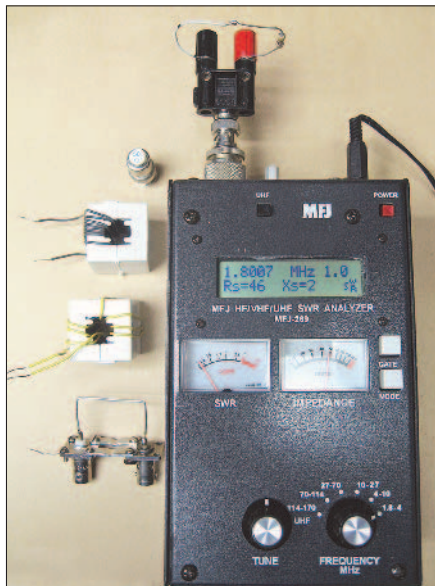
Figure 1 — This photo shows my MFJ 269 SWR analyzer measuring a 47 \Omega resistor at 1.8 MHz. The readout shows a resistance value of 46 \Omega and a reactance value of 2 \Omega . A standard 50 \Omega test load, along with two current transformer secondaries and a T-line section are shown on the side.
