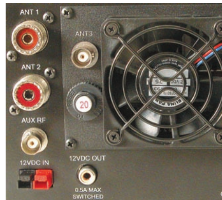
Figure 2 — Rear panel of the K3/100 showing the added dedicated 2 meter antenna connector, ANT3, on the fan panel. The K3/10, which doesn't have fans, has the connector in a similar spot on a blank panel. The ANT2 connector is provided as part of the KAT3 internal antenna tuner.
