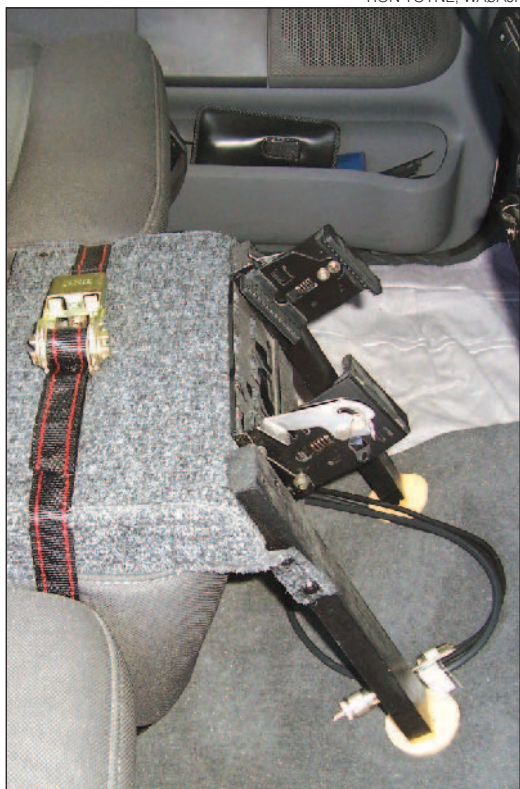
Figure 5 — The movable mount strapped in place in the author's F-150 truck. The width of the base board and length of the legs will vary according to your vehicle's interior layout.
