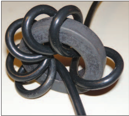
Figure 2 — A common mode choke made of coaxial cable wound on a ferrite toroid core. Note that each turn passes through the core in the same direction.
