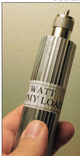
Figure 2 — My little toolbox dummy load is rated at a maximum power of 60 W for 60 seconds.
