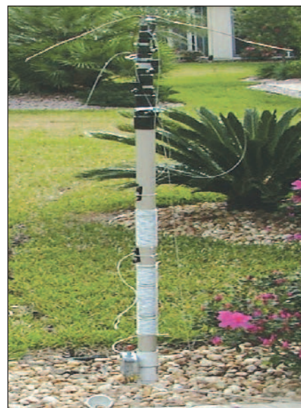
Figure 2 — Close-up view of the base construction. A standard PVC pipe is used as a socket for the mast, forming a telescoping arrangement that can be removed when not in use. The three 18 inch capacitance hat wires are connected to the top of the wire.
