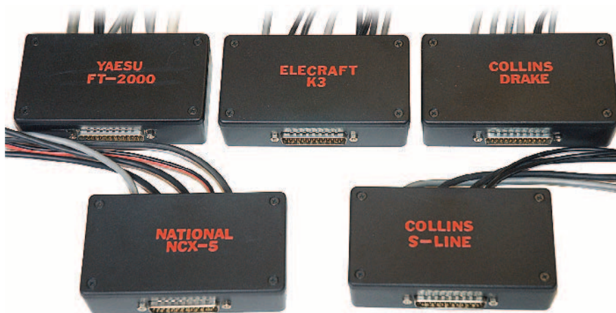
Figure 4 — Breakout pods, customized for each transceiver or exciter, interface the StationPro to the builders' rigs and minimize behind-the-desk "cable clutter."
