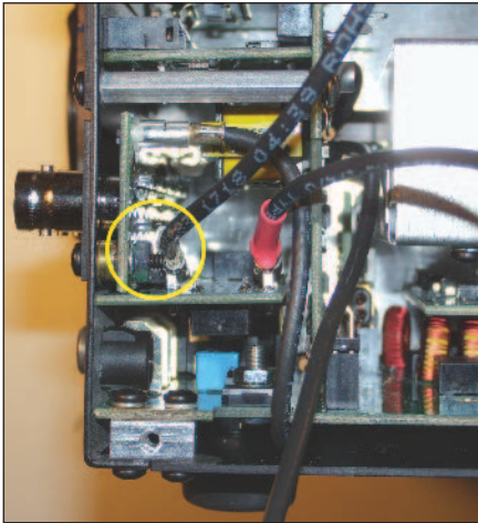
Figure 3 — Close-up of the tight quarters for the RF connector inside the KXV3A transverter interface. By temporarily removing the nut and lock washer, and backing out the screw, the connections could be made without difficulty.
