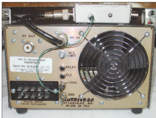
Figure 4 — Attenuator mounted on top of the ALS-600 amplifier cabinet for additional heat dissipation capacity.
