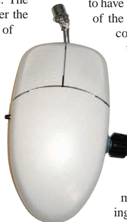
Figure 7 — Mouse based paddle with keyer, buttoned up and ready to go. For mobile use, a pair of stick-on hook and loop fastener strips can keep the paddle in place.
