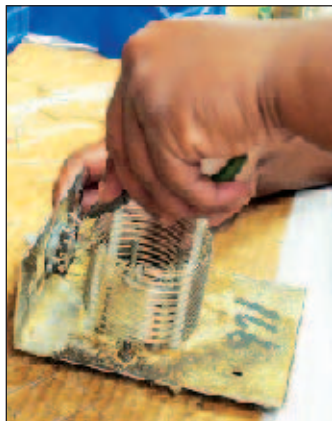
Wiring a high-Q air-wound inductor to a rotary switch for use in an antenna tuner.
