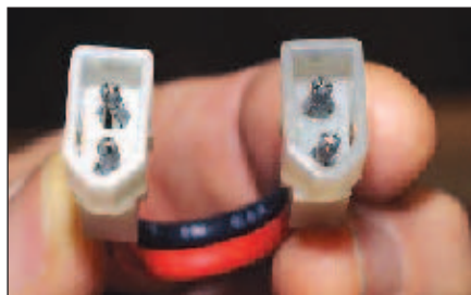
Figure 2 — Molex gender changer — typically used to connect two usual supplies as when charging a battery with a power supply.
