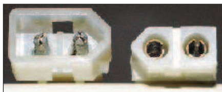
Figure 1 — Molex type connectors. On the right, female pins in a male housing; on the left, male pins in a female housing. The female pins in male housing should be used for supply side connections since they are less likely to short.
