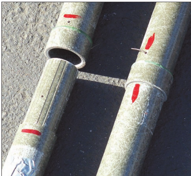
Figure 2 — View of the mating ends of the fiberglass mast sections. The marking is needed because each joint's locking wire position will be slightly different.
