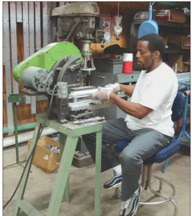
Here we have Randy Sharp dimpling two concentric aluminum tubes to form a double wall structure for a vertical antenna.
