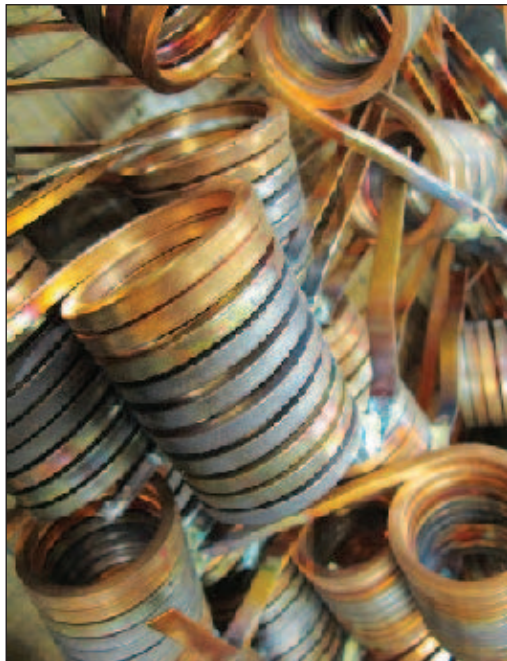
These thick-wall rectangular tank coils will end up in a full legal limit amplifier. Their considerable surface area and mass helps dissipate the extreme heat generated when the amplifier is running full power for an extended period. The taps are silver soldered and the entire inductor assembly will be glass beaded and silver plated for added efficiency.
