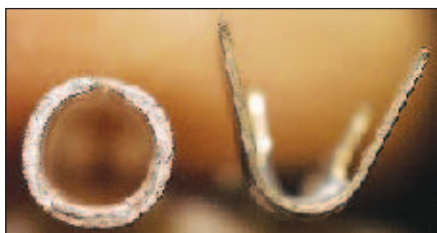
Figure 7 — End view of pin wire attachment mechanism of Powerpole (left) and Molex (right) connector pins. Note the additional thickness of the Powerpole connectors.
