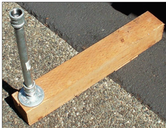
Figure 1 — The flange is screwed onto the end of a 24 inch 4 × 4, as shown.
