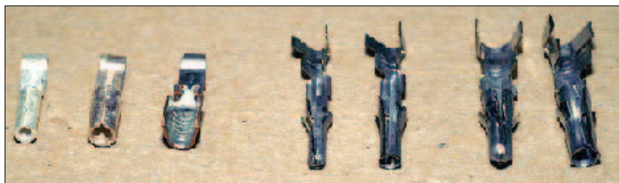
Figure 8 — Comparison of the three sizes of Powerpole pins (left) with the 20 and 7 A Molex pins. Note that all three sizes of Powerpole pins fit in the same size housing and that they can be interconnected.
