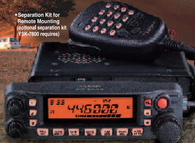
50 W 2 m/70 cm* DUAL BAND FM TRANSCEIVER FT-7900R *70 cm 45 W Size: 5.5" (W) x 1.6" (H) x 6.6" (D) / Weight: 2.2 lb
