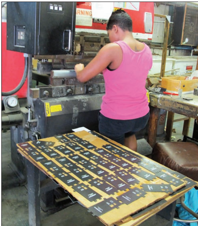
Celletta Tate is using a computer controlled bending machine to form a wattmeter cabinet.
