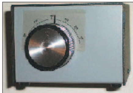
Figure 1 — Front panel view of VHF signal generator. This version is for the 1.25 meter band. It can also be made for 2 meters or 70 cm.
