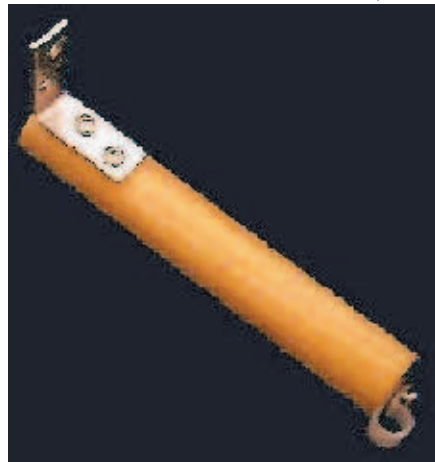
Figure 3 — The homebrewed standoff made from a wooden dowel, angle bracket and cable clamp.
