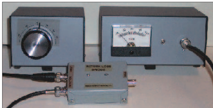
Figure 6 — Typical setup for measuring SWR using the generator and a return loss bridge.
