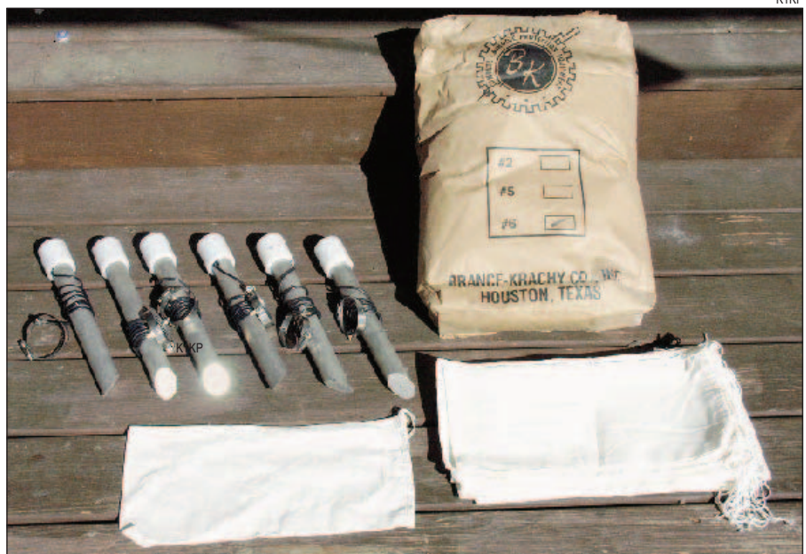
Figure 4 — All the materials required to build six sacrificial anodes.
