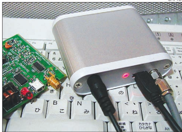
The Soft66AD software-defined receiver by Kazunori Miura, JA7TDO.
