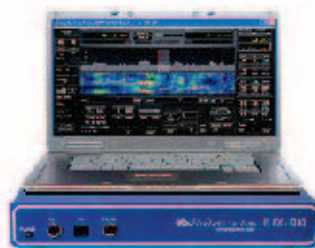
FLEX-3000™ HF-6m 100W Transceiver
