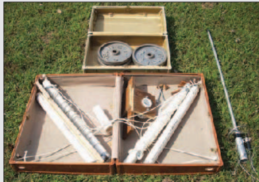
All 14 feet of the suitcase mast stowed and ready to travel.
