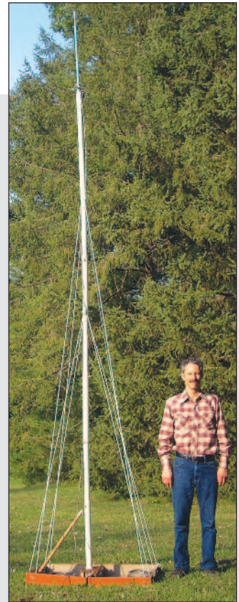
The author and his 14 foot tall suitcase antenna topped with a Cushcraft Ringo AR 2.
