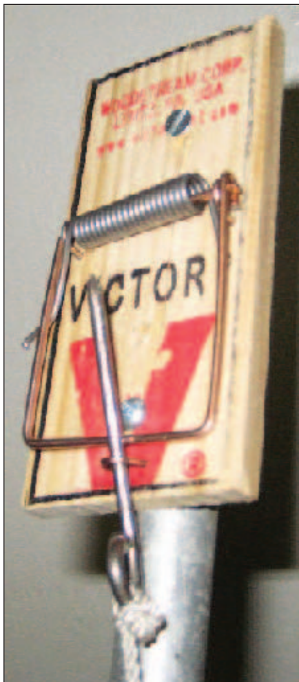
Figure 2 — A mousetrap gimmick to catch the “tail” of a rope hanging out of reach.
