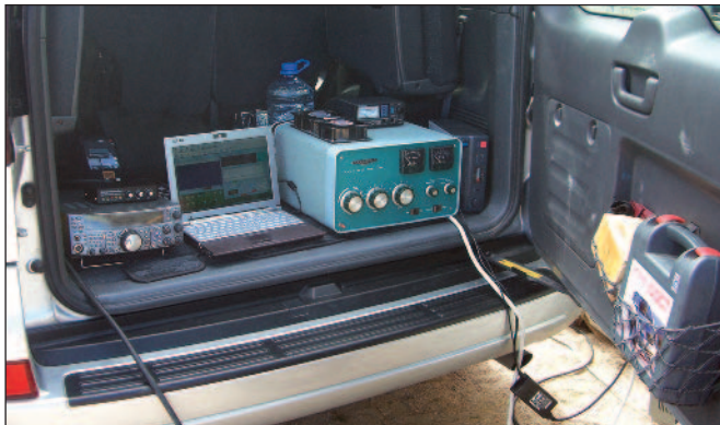
The “shack in the back.” The EME station setup in the rear of Mike’s SUV.
