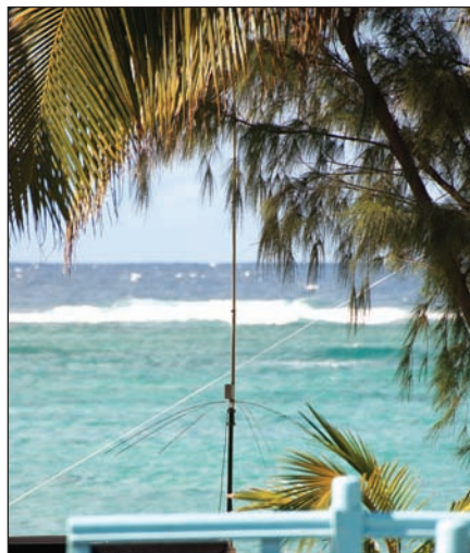
The multiband I1UJX homebrew vertical antenna weighs just 3.5 kg and was used on 7-28 MHz.
