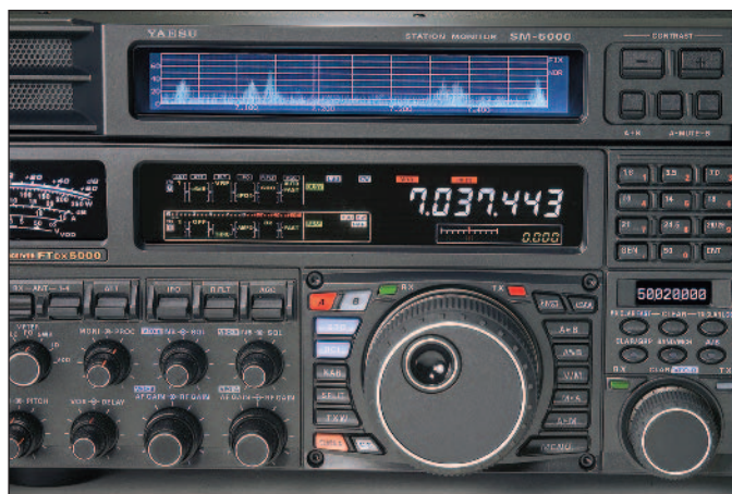
Figure 4 — Close-up of the main display and SM-5000 station monitor screen. To the left of the frequency display is information about the status of antenna, filter, attenuator, filter, preamp, roofing filter and AGC settings for each receiver.
