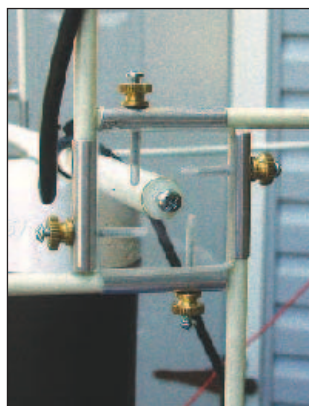
The PortaQuad booms are held in place by knurled brass nuts, as shown in the center of this image. Thanks to its no-tools-required-design, the antenna assembles in minutes.
