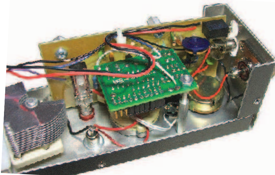
Figure 3 — This shows a more detailed view of the switch and circuit board. The annunciator is stuck to the MFJ-204B panel with double sided tape between the BAND SELECTOR and the RESISTANCE potentiometer. Also notice that the red power wire is connected to the center pin on the right side of the MFJ-204B power switch. Ground can be picked up at any convenient location. The RF input for the Freq-Mite is taken from the back of the FREQ OUT connector on the end of the MFJ-204B.
