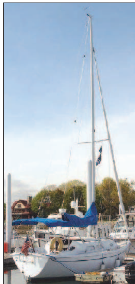
Rear view of the auxiliary sloop Windfall . The HF antenna is the stainless steel wire from the stern of the craft to the top of the mast. In addition to helping hold up the mast, it also puts out a good signal if fed against and reflected from a seawater ground.
