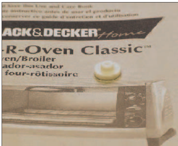
Figure 5 — Teflon bushing ready to be inserted in hole in rear of oven.
