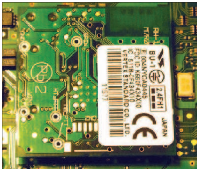
Figure 3 — The BU-1 Bluetooth adapter is a small PC board that piggybacks on the control head. Accessory installation required attention to detail but wasn't difficult.
