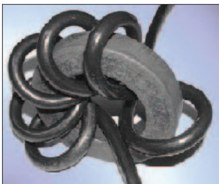
Figure 2 — Common mode choke made by winding the antenna feed coax through a ferrite toroid. The coax can be neatly secured with nylon tie wraps.
