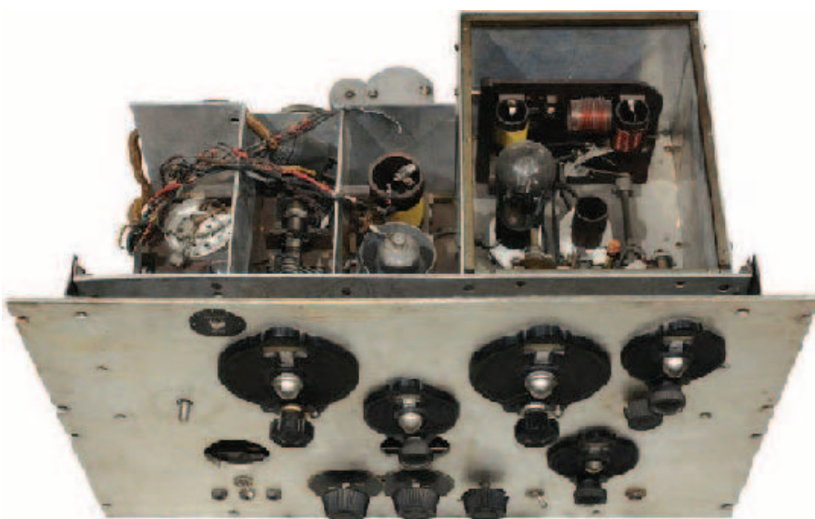
Lamb’s prototype in the collection of ARRL HQ in Newington. As built, it used an ordinary broadcast receiver for the second IF and audio stages.
