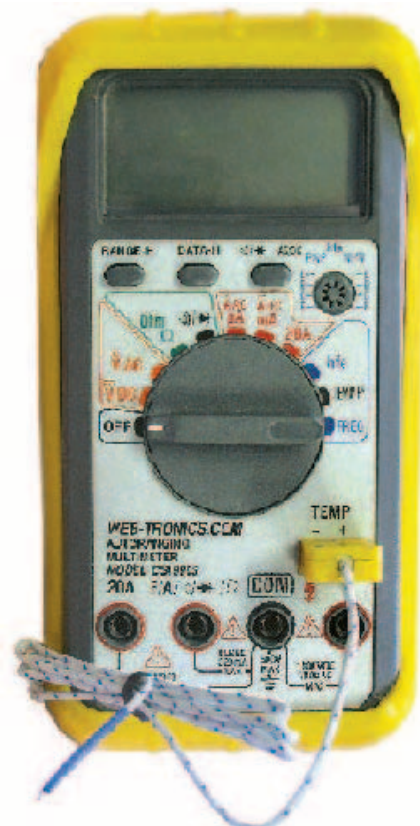
Figure 2 — Inexpensive multimeter with type-K thermocouple probe.
