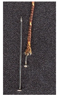
Figure 4 — Tip of type K thermocouple from Keithley instrument with a pin for comparison.
