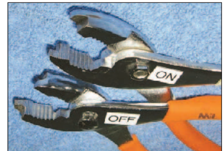
Figure 4 — Joining and separating PowerPole connectors requires that two pliers be modified in a mirror image of each other.
