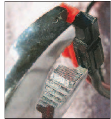
Figure 3 — Using the modified pliers simplifies the task of joining a pair of PowerPole connectors.
