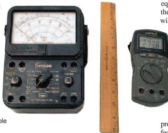
Figure 2 — A modern digital voltmeter next to the author's venerable Simpson 260 series analog VOM.
