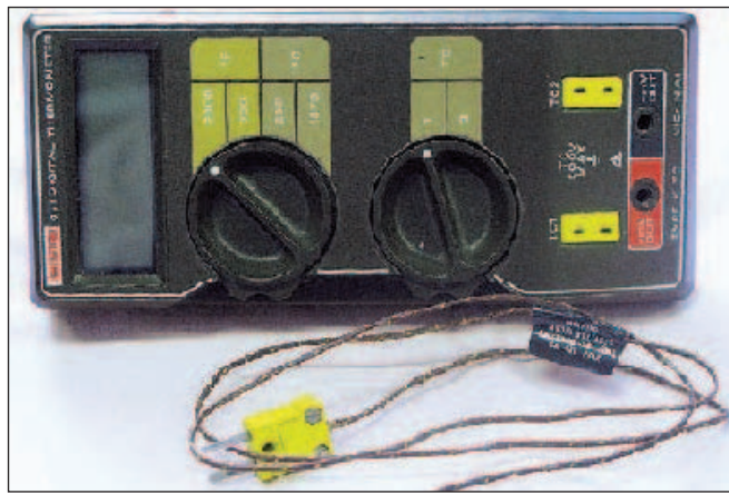
Figure 3 — Keithley electronic thermometer with type-K thermocouple probe.
