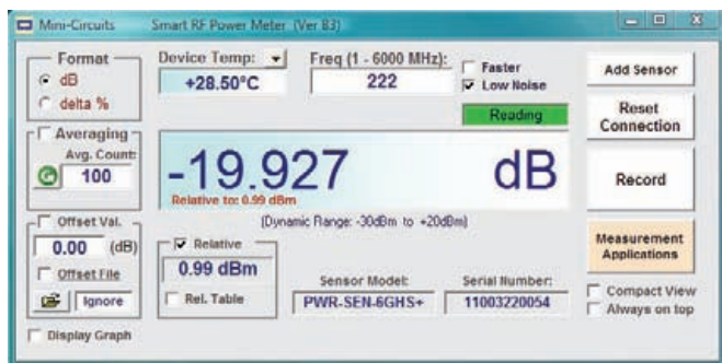
Figure 3 — PWR-6GHS+ screen showing the actual measured attenuation of the author's surplus 150 W, 20 dB attenuator.
