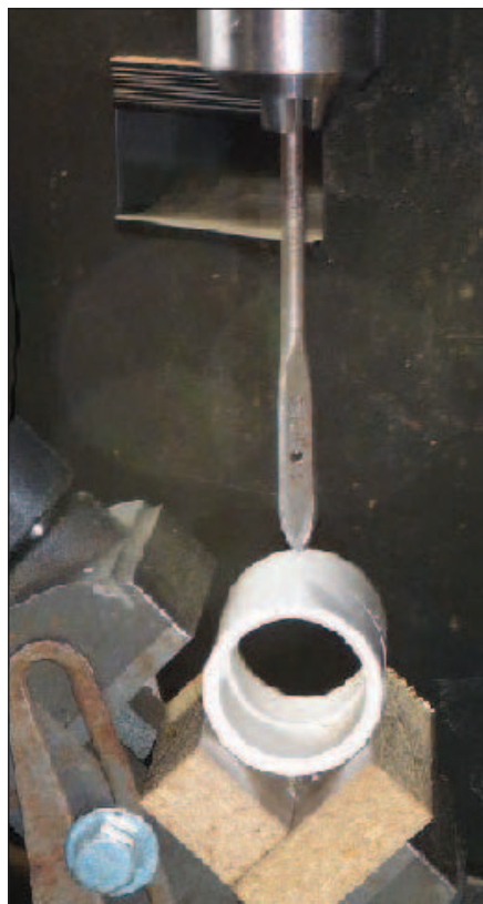
Figure 5 — Setup to drill a round boom at its center.
