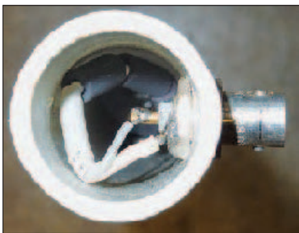
Figure 4 — Balun as attached to the BNC antenna connector.
