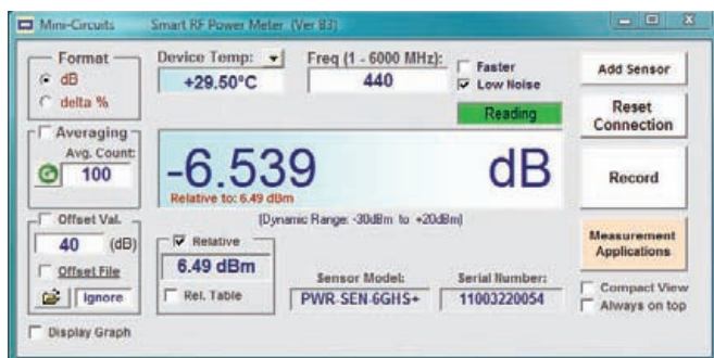
Figure 6 — Return loss of the 147 MHz antenna measured at 445 MHz.
