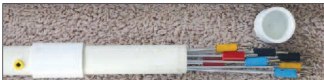
Figure 6 — The antenna elements inserted in the boom section ready to button up for travel.
