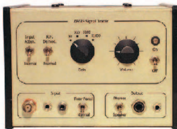
Figure 2 — Signal tracer front panel. The legend was designed using Microsoft PowerPoint.
