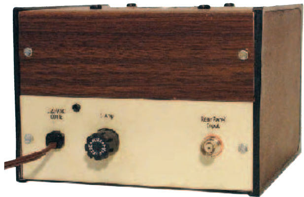
Figure 3 — Signal tracer rear panel. This legend was also prepared on clear film using Microsoft PowerPoint.
