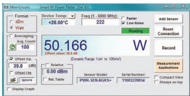
Figure 4 — Measured output power of the author's Jetstream 222 MHz transceiver.
