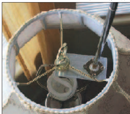
Figure 4 — The business end of the “lamptenna” connected and ready to get on the air.
