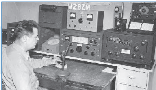
Joseph Koenig, W2BZM, in his 1950 shack. Equipment from the left: unknown, Collins 32V-2 transmitter, rotator indicator, Triplet modulation monitor (top), Collins 75A-1 receiver, field strength meters, BC-221 frequency meter (top), and an RCH CZC-46209 Scott Radio Labs receiver.
