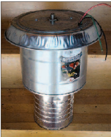
Figure 5 — The completed dummy load. Since what is now the bottom of the oil reservoir is a convex shape, a coffee can is used as a temporary pedestal mount. Two holes drilled into the top, as well as the grommet for the three temperature sensor leads, permit air to escape when placing the top on the oil reservoir bottom. For a more stable arrangement, a bucket is less precarious.
