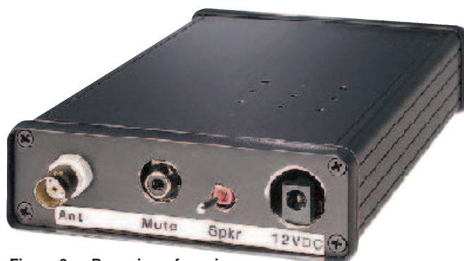
Figure 3 — Rear view of receiver. See text regarding use of the MUTE jack.
