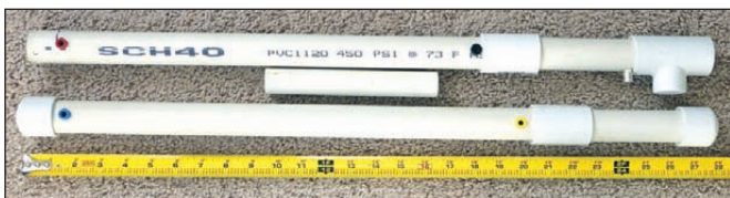
Figure 7 — Antenna ready to go. The elements are secured in the section with the end caps.
