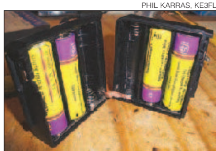
Figure 1 — The alkaline battery pack opened and with two batteries removed to show the desoldering braid jumper.
