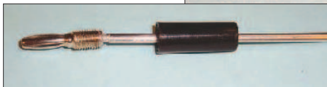
Figure 2 — Element tip with cap unscrewed. The threaded aluminum rod is shown.
