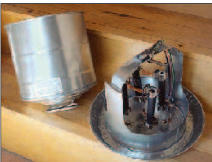
Figure 4 — The dummy load is constructed from the two parts of the fount. The inner container's side walls are cut away with a saber saw permitting oil to freely contact the outer (left) container but leaving two strips and the handle. The entire unit is then turned upside-down. The 2 gallon water container (left) is filled with oil, and the right half is now the lid, complete with the resistors, clamps and UHF female coaxial connector.
