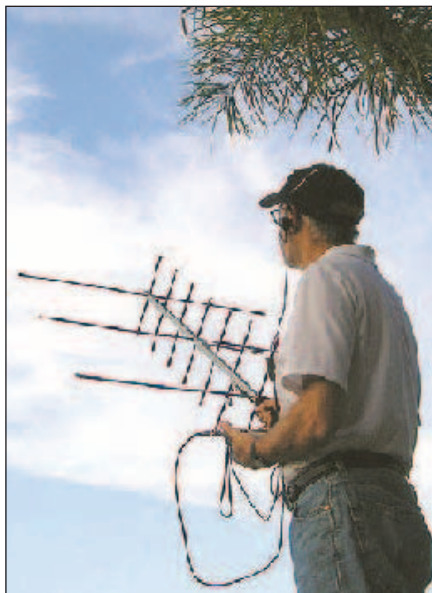
A simple handheld setup like this will be more than sufficient to receive ARISSat-1.
