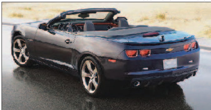
The 2011 Chevrolet Camaro convertible features its AM/FM radio antenna inside the spoiler, thanks to some ham ingenuity. The “shark fin” antenna is for satellite radio, OnStar and cellular signals.
