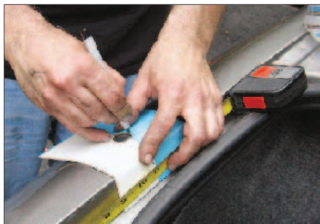
Figure 3 — Transferring the hole pattern to the right spot on the driver-side quarter panel.
