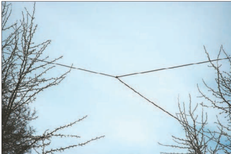
Figure 1 — A “horizontal dipole” doesn’t have to be perfectly horizontal. This commercial dipole antenna was simply installed to fit the available space.
