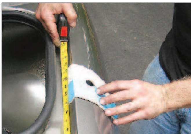
Figure 2 — Tracing the hole for the AM/FM antenna and locating it relative to the edge of the passenger-side quarter panel.
