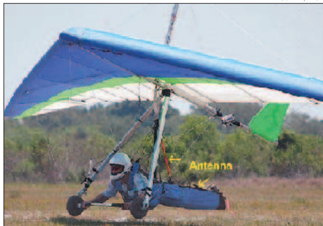
Figure 3 — This photo shows how the 2 meter dipole is integrated into the harness.
