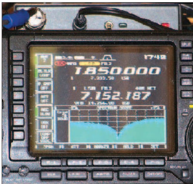
Figure 1 — Photograph of the display on the 'PROII showing the displayed spectrum with the notch in the center.
