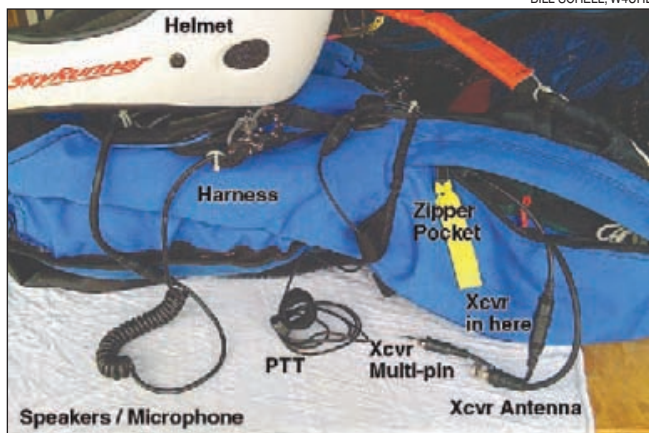
Figure 2 — The communications and gliding gear are integrated so as to provide the best communications with the least amount of weight and drag on the glider.
