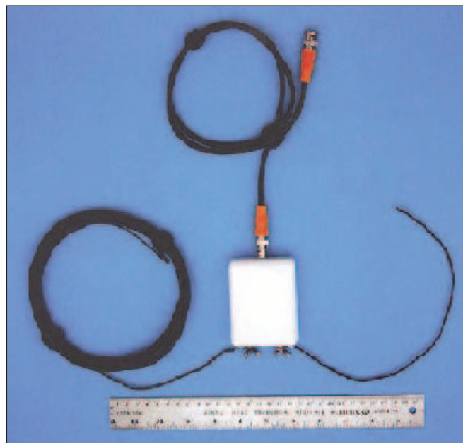
Figure 2 — Complete antenna with RF transformer, 27.5 foot radiator, 1 foot counterpoise and 3 feet of RG-58 feed line.
