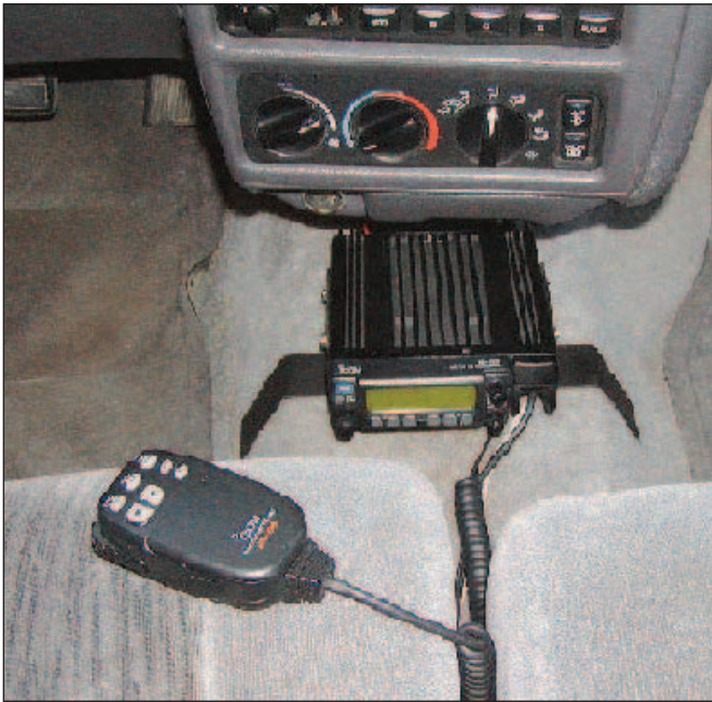
Figure 7 — The ICOM IC-207H snugly mounted on the transmission hump using an aluminum bracket and hook and loop tape.
