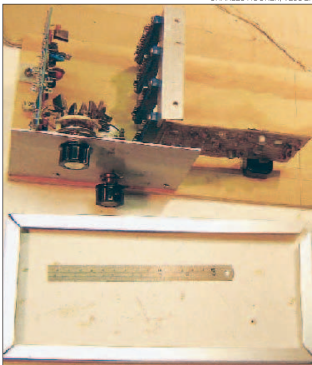
Figure 2 — A piece of aluminum L-bracket that has been cut and bent to form a rectangular frame. The transmitter breadboard is shown above.
