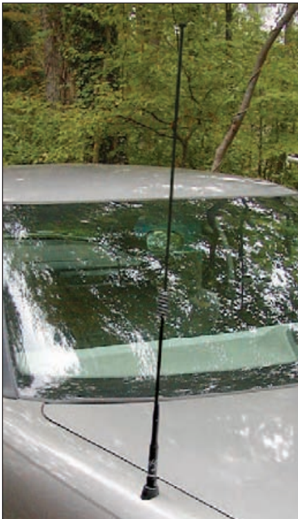
Figure 5 — The EX-107 mounted on a 4 inch UG-363 type barrel connector through the new grommet.
