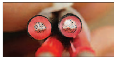
Figure 2 — Take a wire size gauge, calipers, ruler or piece of real #10 AWG wire with you for comparison when buying cable.
