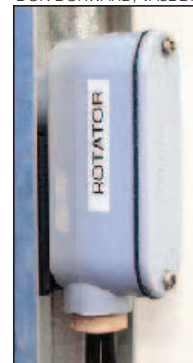
Figure 4 — The rotator break-out box mounted to the side of the tower. Note the modified wine bottle cork to seal the bottom cable entrance and the weatherproof seal between the cover and the box.
