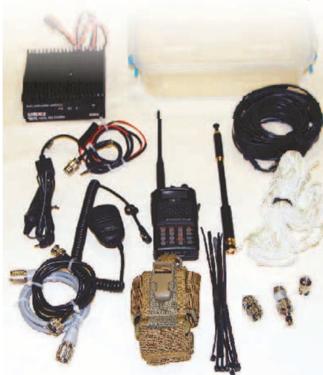
Figure 1 — This is my entire handheld radio kit. Clockwise from top left: Mirage BD-35 dual-band amplifier, plastic storage box (1 of 2 to hold everything), rolled up "Slim Jim" J-pole antenna, parachute cord for mounting of J-pole antenna, extendable whip antenna, coax adaptors for radio, zip ties for mounting of J-pole antennas, belt pouch for handheld transceiver, pigtail coax adaptors, plug in speaker-microphone, cigarette lighter recharging chord for handheld radio and extension cable for amplifier. My handheld transceiver is shown in the center.
