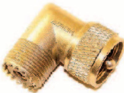
Figure 3 — Amphenol UG-646/U UHF type right angle adapter. The author found them unsatisfactory in his 800 MHz installation.
