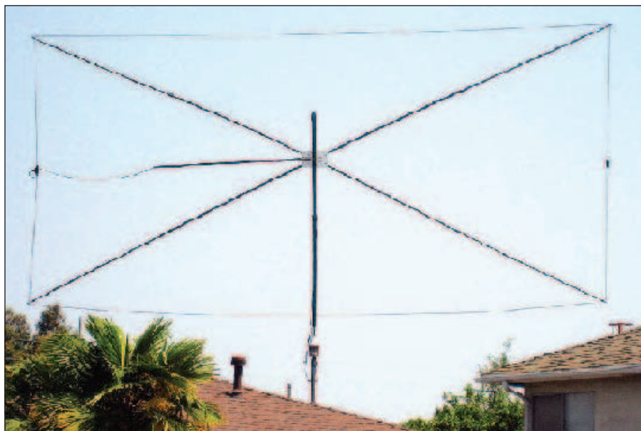
Figure 1 — The rotatable flag receiving antenna in place and ready for those rare West Coast to Europe openings.
