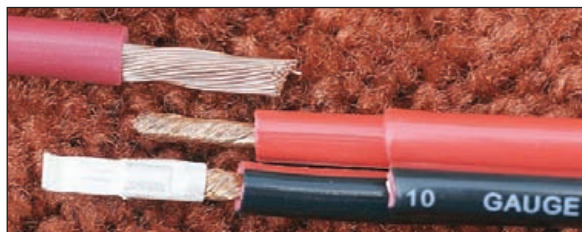
Figure 1 — All three conductors are labeled as #10 AWG. Two of the three are obviously mislabeled. It appears that the manufacturer in the lower two wires just adds insulation material to cover up its deception for the reduction in copper. Is it possible that plastic is less expensive than copper?
