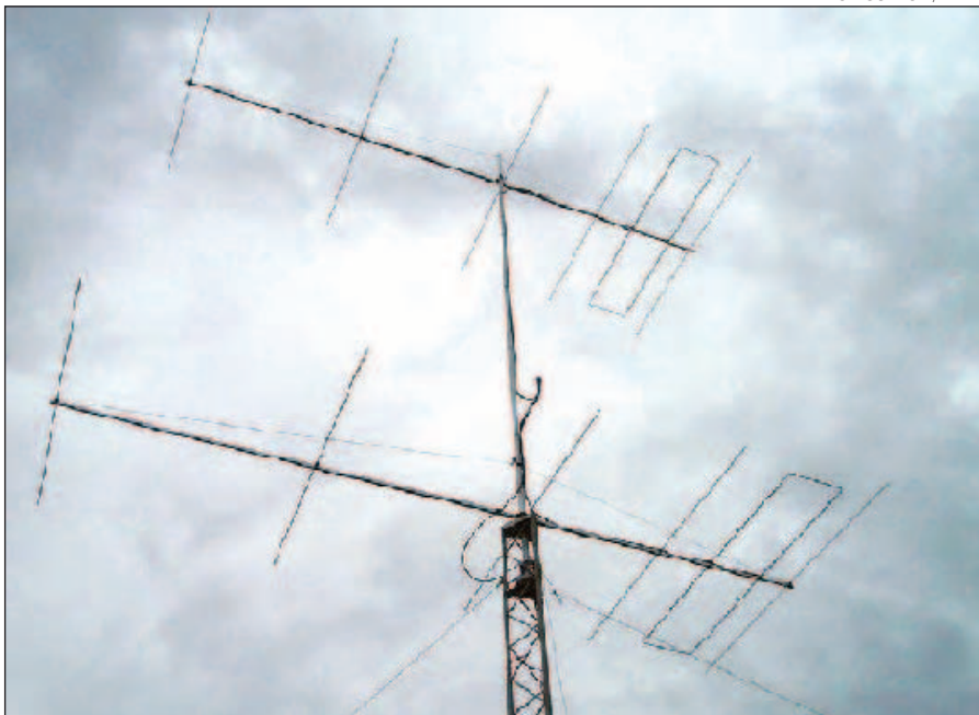
Figure 1 — The antenna system of Bob, ZL1RS, is a pair of stacked 6 element G0KSC LFA Yagis. Bob is located on New Zealand's north island and has an excellent horizon toward the Pacific Ocean.
