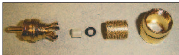
Figure 1 — There are only five components to the Shakespeare connector: The "head" of the connector with the center pin and piercing fingers, the coupling ring, a rubber O-ring, the cover ring and a small plastic guide cap for use with RG-58 A/U coax only.
