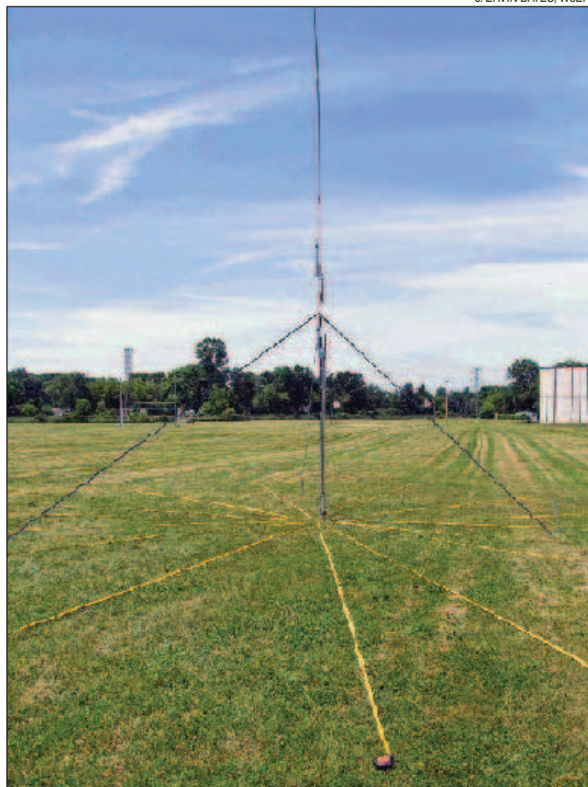
Figure 12 — Tape measure radials, fully deployed at 2009 ARRL Field Day, on the grounds of Gardner Middle School, Lansing, Michigan.
