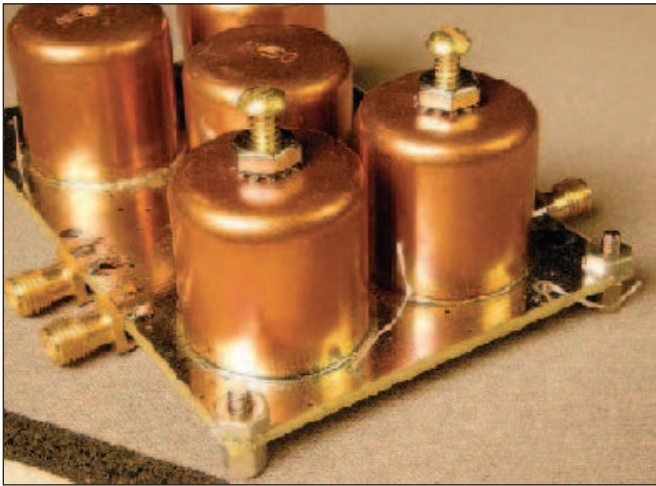
Figure 3 — Ordinary copper pipe caps can be used as filters to construct a microwave transverter.
