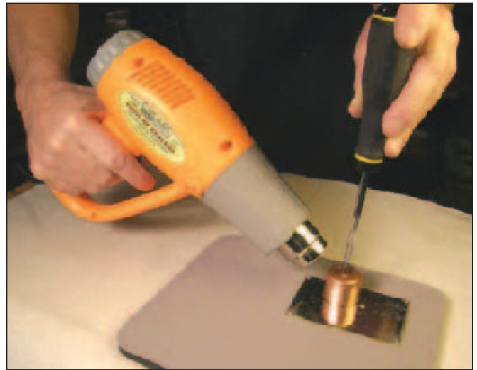
Figure 5 — Once the pipe cap is positioned, hold it down with a screwdriver and use a heat gun to melt the solder ring.
