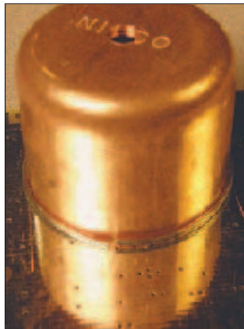
Figure 4 — Here is a pipe cap ready to solder. You can see the solder ring and the scribe lines.
