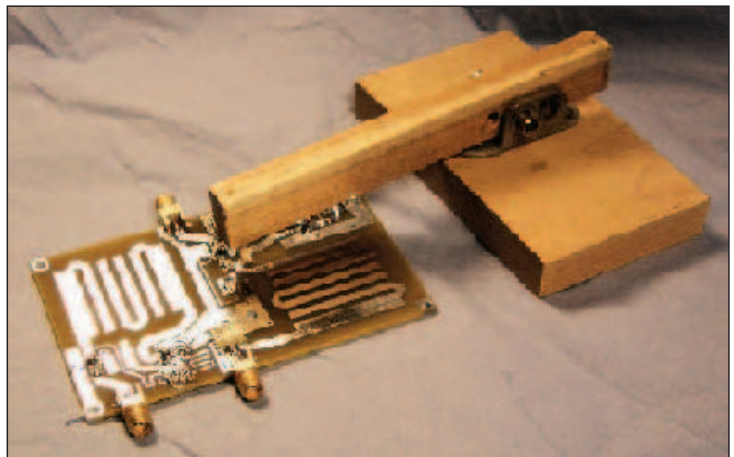
Figure 2 — A homemade fixture used to hold the surface-mount component during soldering.
