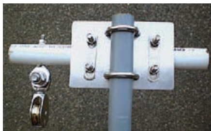
Figure 3 — Aluminum plate and pulley assembly shown bolted to the mast.
