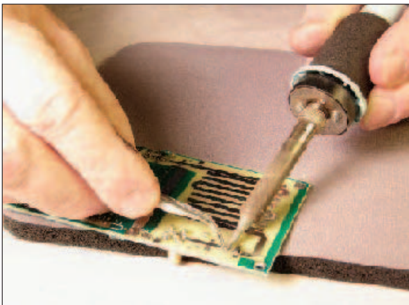
Figure 1 — This is the manual assembly technique with the tweezers, using a mouse pad as a non-slip base.
