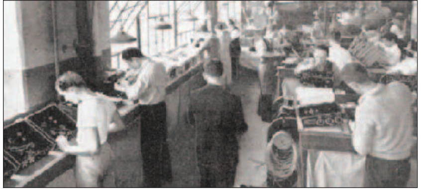
Working under clean, comfortable conditions, the wiremen in the Lafayette factory do consistently careful and accurate jobs on receivers, transmitters, transceivers and amplifiers.
