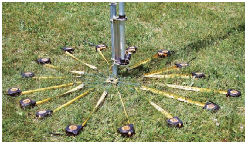
Figure 11 — Tape measure radials connected to base of trap vertical, ready for deployment.
