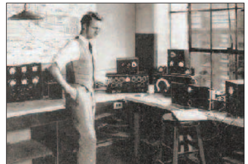
Sound Engineer Frank Dostal performs scientific measurements of audio gain, frequency response, etc, in this special audio frequency laboratory containing the latest test equipment.
