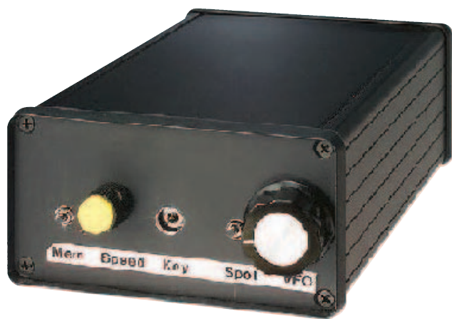
Figure 3 — Front view of the compact 7.5 W transmitter. Note that the cabinet needs to be higher than that of the lower power version.
