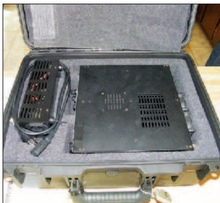
A Pelican iM2450 will house an Elecraft K3 and Astron SS25 switching power supply with no problems as a carry-on.
