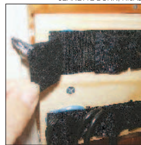
Figure 5 — A completed set of flaps all ready to hold whatever needs holding. Note the short piece of string glued to the "open" end to make it easy to open the flap.
