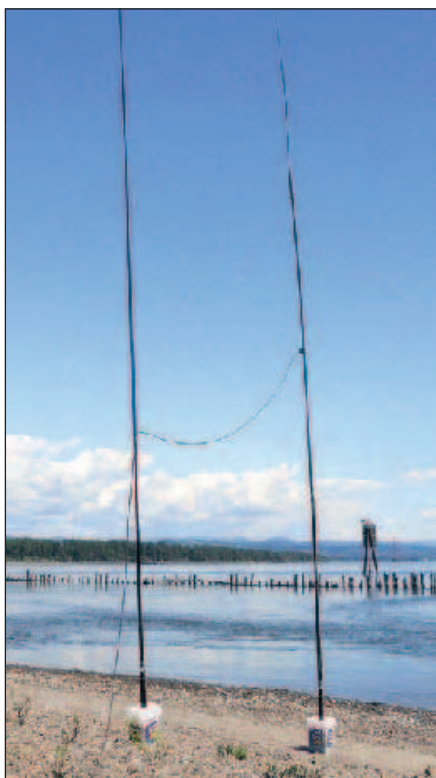
Figure 3 — The coax support vertical is built next. It gets the coax away from the driven element's bottom section. The coax support vertical is built just like the driven element. Each section is raised in three foot increments, taping each section as they are extended, until both are at full height. At this point you have an omnidirectional half wave vertical dipole. This is a good time to hook up the radio and check the band to see where you want to aim the antenna.
