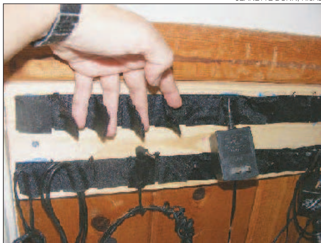
Figure 6 — Each of the short Velcro hook strips is glued to the long loop strip at one end creating a flap that can be closed over whatever small accessory you want to keep available but out of the way.
