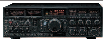
FTDX-9000C/D/MP 400 watts, dual analog meter sets, LCD display, memory card installed, main and sub receiver VRF, full dual rx, external power supply.
