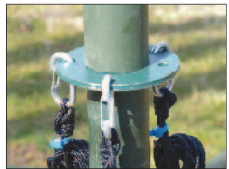
Figure 3 — Guy ring used to fasten guy ropes to the top section of the mast.
