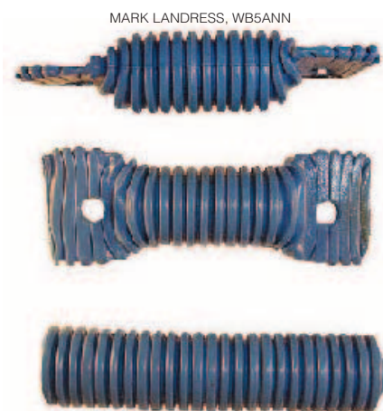
Figure 4 — Both side and top views of a finished insulator and a piece of the conduit used for their construction.
