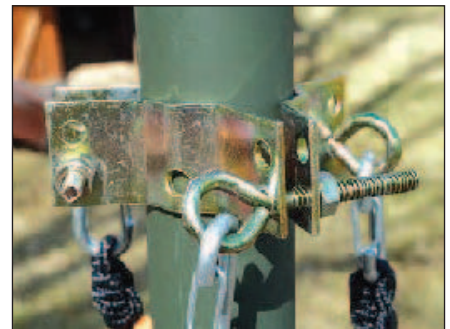
Figure 4 — Mast clamp used to fasten guy ropes at intermediate heights.
