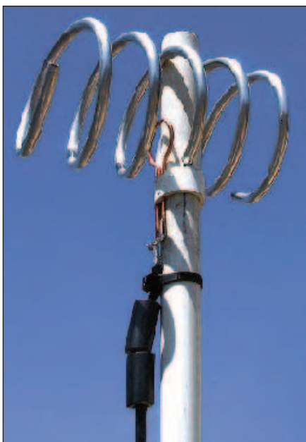
Figure 7 — My five turn 2 meter test helix, illustrating minimum turn spacing. Note also the ferrite balun.
