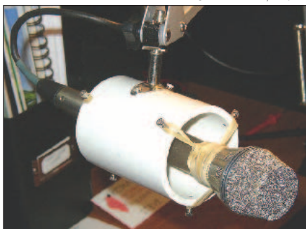
Figure 2 — The finished microphone suspended in a makeshift holder on the end of the lamp “boom.”
