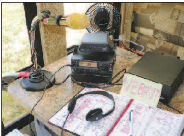
The VY1RST and VE8RST mobile shack. It consists of a TS-50 transceiver, LDG Z-100 tuner, 20 A power supply and a Heil microphone. The fan helped keep the author and his rig cool.
