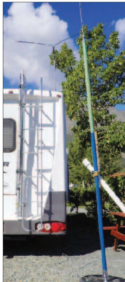
The antenna farm of VY1RST consisted of a 40 meter antenna at 20 feet and the Webster Bandspanner. The Hustler 4BTV on the ladder is a backup.
