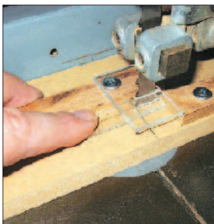
Figure 4 — Marked side of spreader is held against fence and pushed to stop. Note finger guard.
