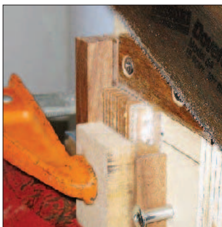
Figure 5 — Hand saw cutting jig. Top fence also serves as saw guide. Stack of spreaders is compressed by wedge.
