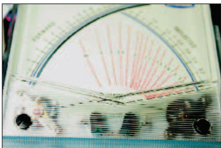
Figure 7 — You can see the LEDs behind the diffuser portion of the front meter cover here. Be sure that the LEDs do not interfere with the meter movements.
