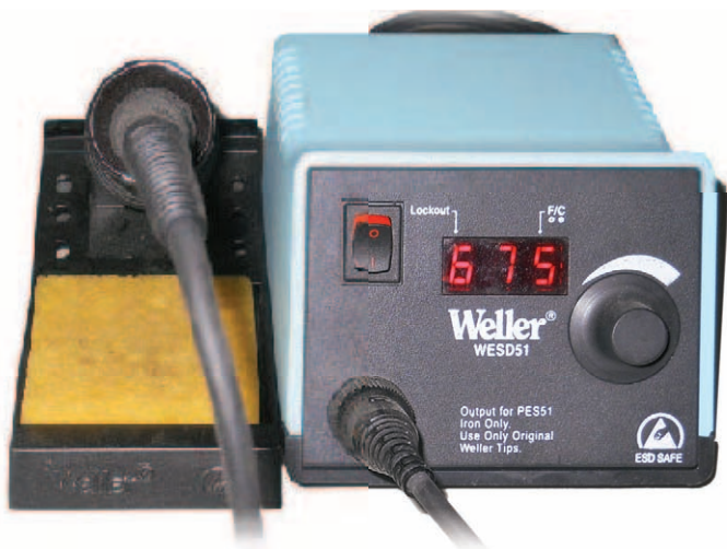
Figure 4 — A temperature controlled soldering station, such as this Weller WESD51, is highly recommended for kits that require soldering of solid state devices.
