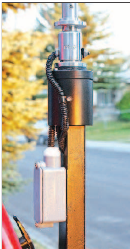
Figure 6 — Detail of base connection arrangement. The shunt matching inductor is in the gray PVC electrical box.
