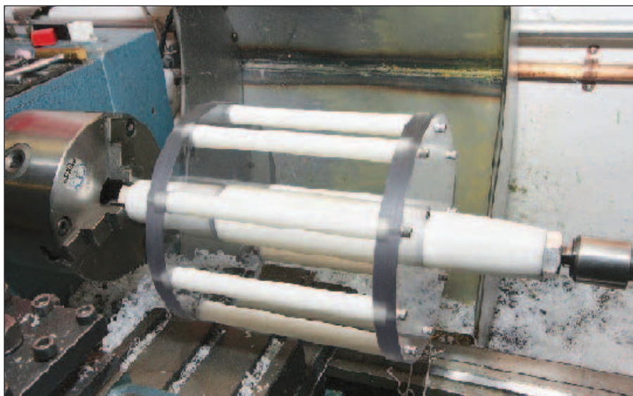
Figure 3 — Loading coil form on lathe before the wire is wound around it.
