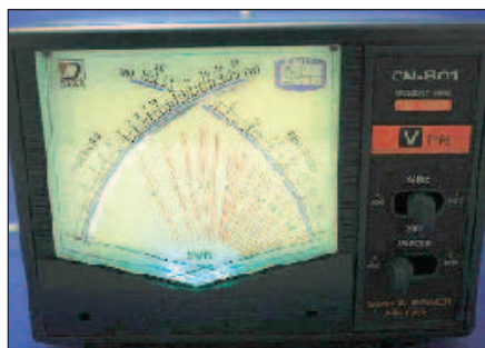
Figure 8 — With the LED replacements for the bulb, the meter now has a soft glow that makes the meter easy to read in a darkened shack, without being too bright and causing glare.
