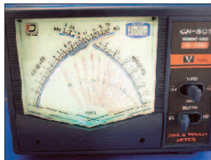
Figure 1 — The Daiwa CN-801 SWR/power meter is a versatile instrument. The meter face is illuminated by a small bulb below the bottom of the meter movement.
