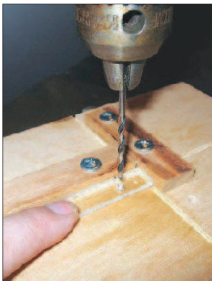
Figure 3 — Note saw kerfs serving as gutters to keep debris from getting between piece and fence.
