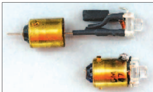
Figure 1 — The updated bayonet bulb. Above is the LED assembly ready to be mounted in the bayonet base. Below is the completed bayonet LED.
