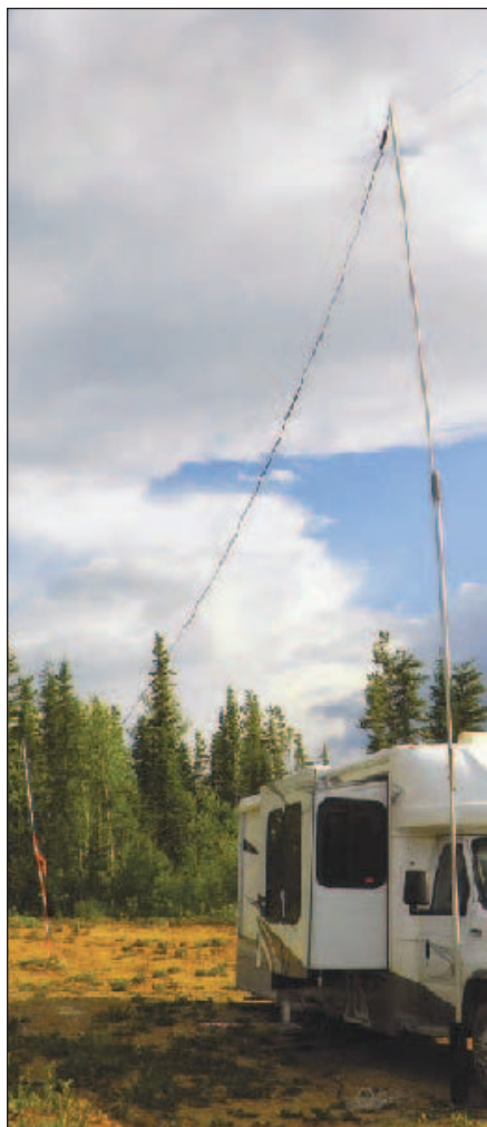
Here is the VE8RST G5RV antenna near Ft Liard, Northwest Territories.
