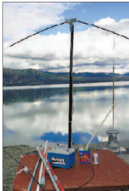
The VY1RST antenna farm, which consists of a shortened 40 meter inverted V and a Webster Bandspanner.
