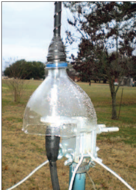
Figure 4 — The soda bottle antenna shroud over the end of the 40 meter resonator.
