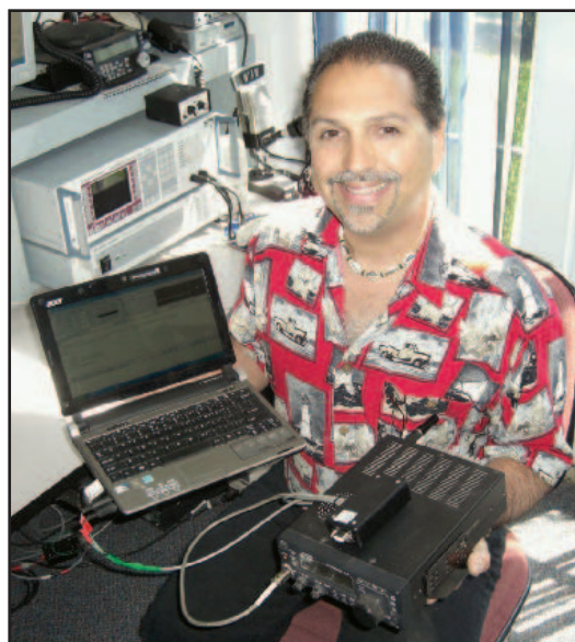
W1AW Station Manager Joe Carcia, NJ1Q, shows off a simple RTTY station: a rig, a netbook PC and a homebrew soundcard interface. Don Hill, AA5AU talks about sound card interfaces on his RTTY website at www.aa5au.com/rtty .
