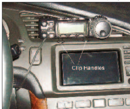
Figure 3 — Mounted radio controller head with clip handles attached.
