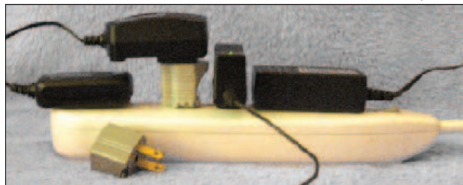
Figure 6 — Ground adapter plugs can help your wall warts rise above a congested outlet strip.
