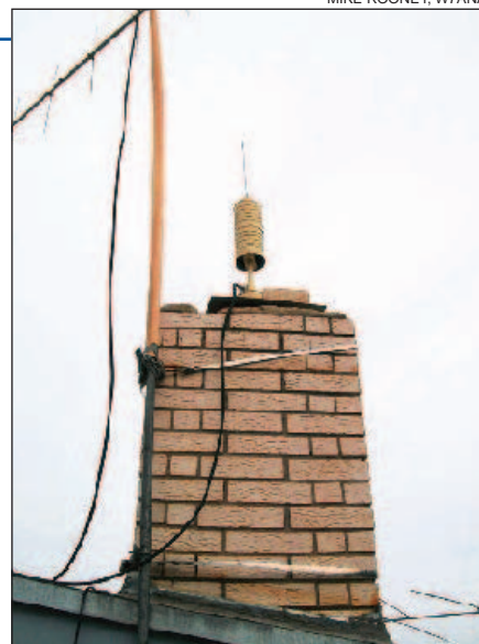
Caffeinated antenna: Mike Rooney, W7ANA, of El Paso, Texas adapted an idea he had seen in an old issue of QST to a friend's antenna farm — substituting two 3-pound coffee cans for the radial portion of his 2 meter vertical dipole. The original author used copper pipe. "One has to be aware of the winds in their specific area and mount the antenna accordingly," he cautions.
