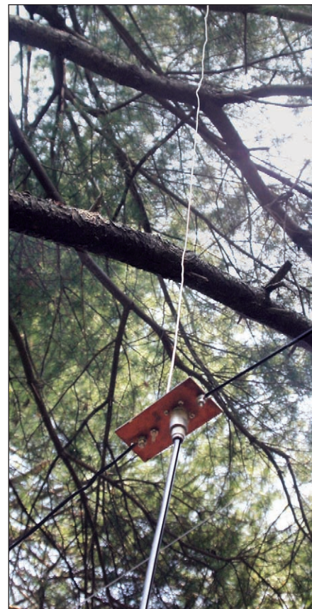
Figure 6 — The vertical monopole suspended from my pine tree at 45 feet.
