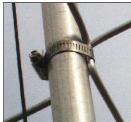
Figure 5 — A close-up of the 6 meter rods attached to the R7000 with a hose clamp.
