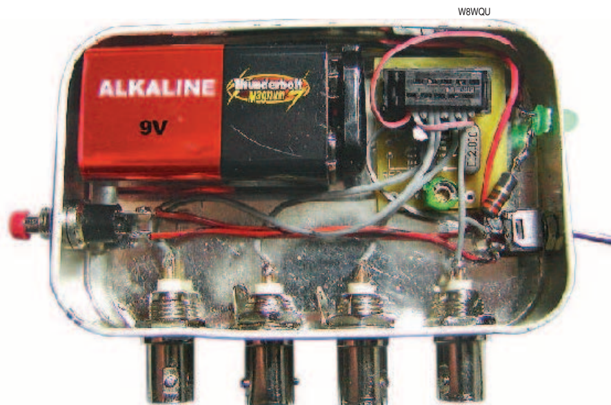
Figure 4 — Jerry, W8WQU, installed his YACC-2 in the ubiquitous Altoids tin. He named the result the Pocket YACC .
