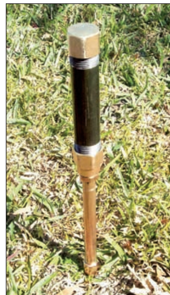
Figure 8 — The lawn dart made from surplus pipe and fittings. It can be driven into the ground with a heavy foot or a short handled sledge hammer.
