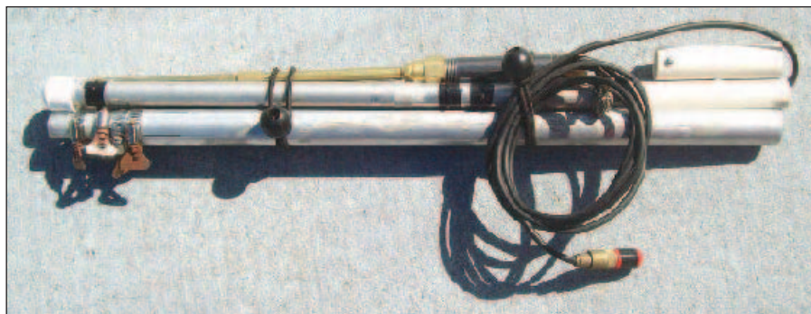
Figure 5 — The OCF sleeve dipole all packed up and ready to go. One could easily substitute most homebrew or commercial antennas.
