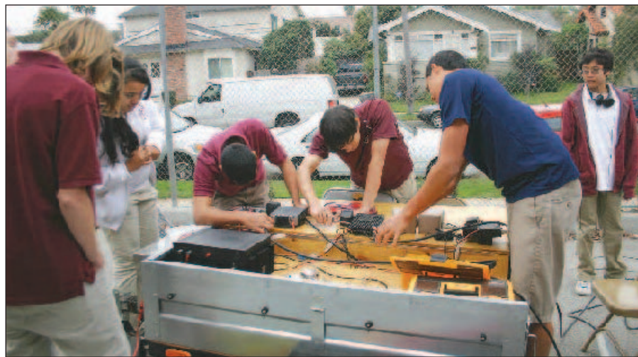
Wilson AREC team members work on the mobile radio station featuring 2 meter/1 1/4 meter and 2 meter/70 cm mobile radios. With a 50 A power supply and Powerpole connectors the radios can be easily interchanged. The station can be powered by ac, a 100 Ah gel cell, the team's generator or a car battery with jumper cables and Powerpole connectors. From the left are Corleone Ham, KJ6DXN; Philip Scholnick, KJ6MCD; Max Chang, KJ6EMB, and Kevin Keo, KJ6LNZ.
