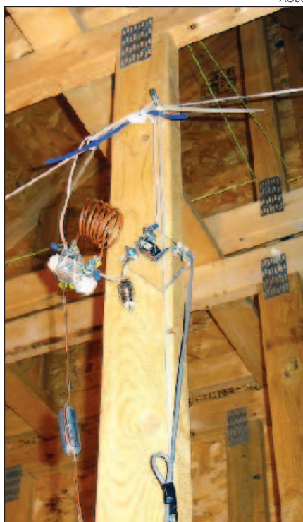
One of AC0C's earlier attic experiments — a 20 meter wire beam antenna.
