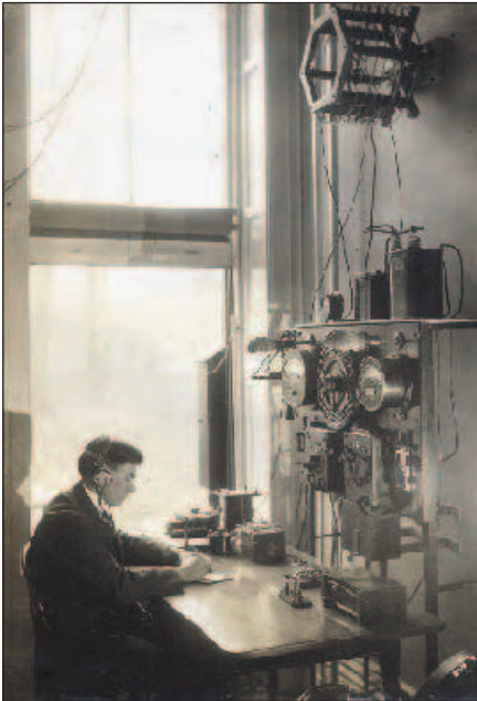
In 1916, the Museum's station was rebuilt under the direction of Ms Lee to improve its appearance and efficiency. It also operated with a new federally assigned call of "2KP." The reworked station sported a 13.2 kV, 500 W spark coil.
