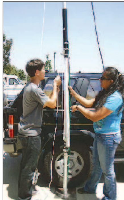
Chip Margelli, K7JA, designed a mast launcher for military masts like the one the Wilson AREC team uses. Margelli demonstrated it and we built one the next day. Here Philip Scholnick, KJ6MCD, and Carina Ochoa, KJ6MCB, are using the Margelli mast launcher for Field Day 2011.
