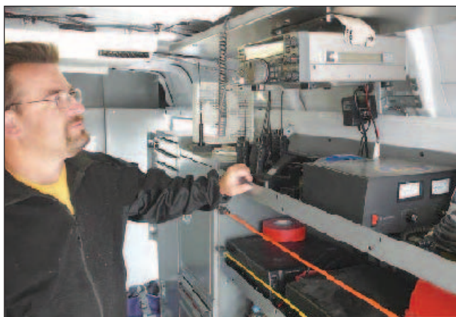
Ed Winchester admiring the TS-570D HF radio installed on EMMCOMM-1. The unit also has a Kenwood TS-480 for Pactor/WL2K coupled to an SCS Pactor controller. Below the radio is storage space for a wide range of supplies such as handheld transceivers, a spare power supply and cables together with several shelves and storage lockers for other spares and tools.
