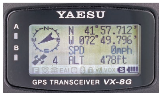
Figure 3 — The GPS screen shows position (latitude and longitude), altitude and number of GPS satellites received (in this case, four). You can scroll down to see the current time. If you are moving, it also displays speed and direction.
