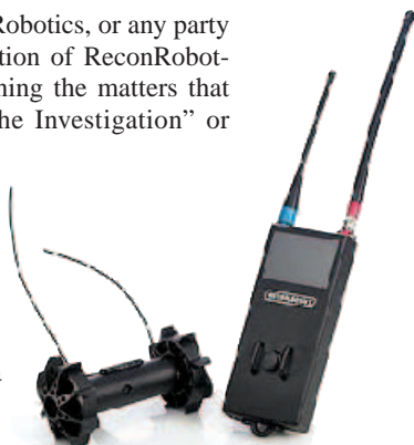
The Recon Scout — manufactured and marketed by ReconRobotics — is a remote-controlled, maneuverable surveillance robot designed for use in areas that may be too hazardous for human entry. In 2010, ReconRobotics was granted a waiver by the FCC for the device to operate between 430-448 MHz, a portion of spectrum available to the Amateur Radio Service on a secondary basis.
