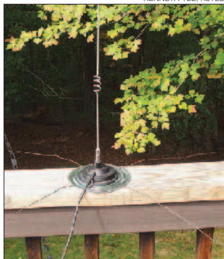
Figure 3 — With the radial adapter attached the mag-mount is freed from your car’s roof and can be placed on any convenient surface or hung from a tree.
