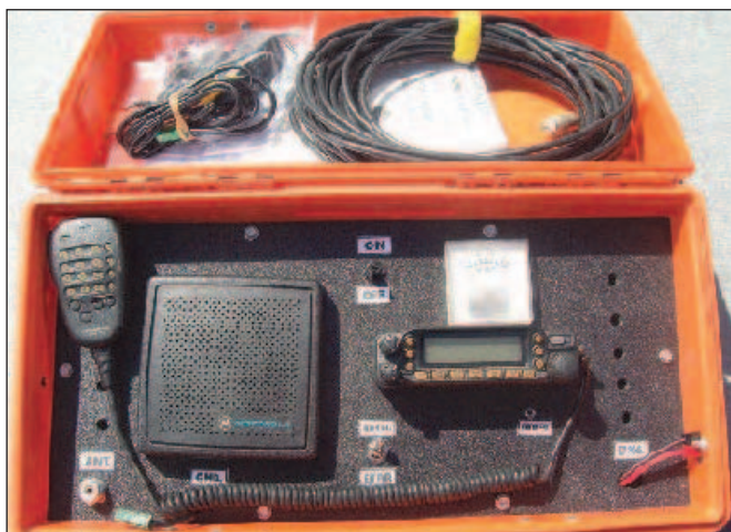
Figure 2 — View of the front (top) panel made from ABS plastic along with some of the ancillary components that are carried in the container. Under the cable in the lid are frequency lists, message forms and equipment manuals.
