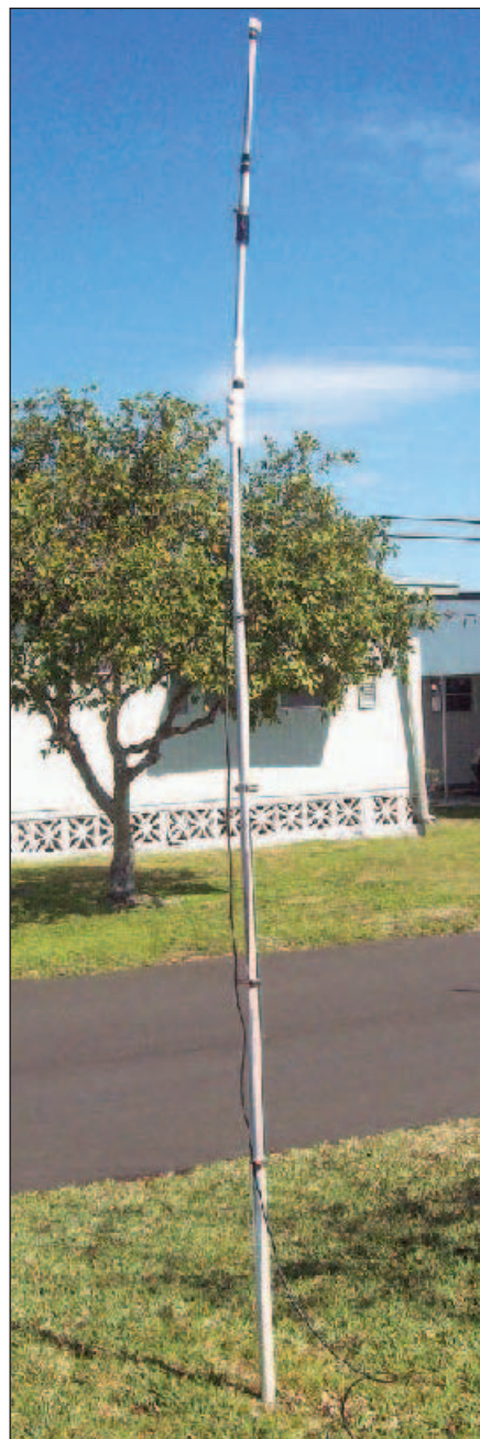
Figure 6 — The antenna and supporting mast set up on unpaved ground. The mast is simply slipped over the lawn dart mentioned in the text and shown in Figure 8.
