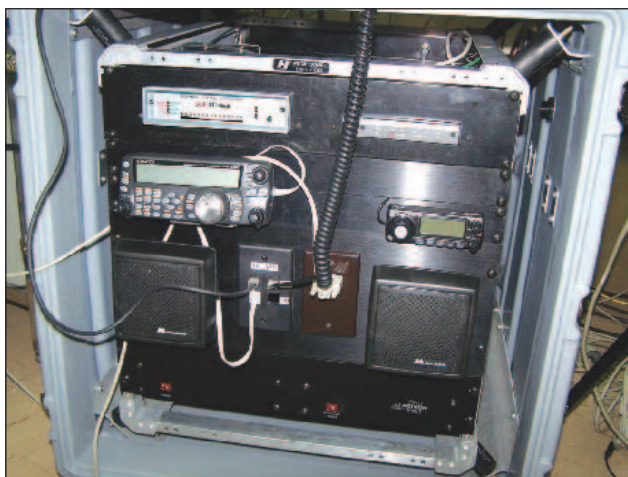
Figure 4 — Front of the BMERS portable station. The HF rig (a Kenwood TS-480SAT) and PACTOR modem (SCS PTCII) are on the left. A UHF/VHF rig (IC-208H) and packet modem (Kantronics KP3-C+) are on the right.
