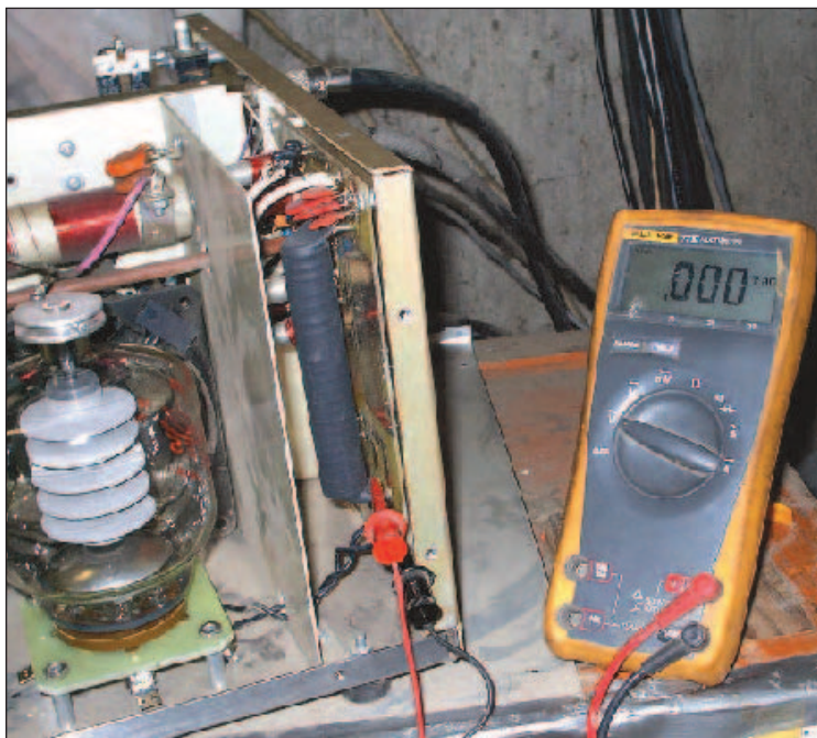
Figure 2 — Measuring the filament voltage at the output of the filament choke.
