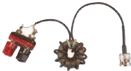
Figure 1 — A coaxial common mode choke, a 1:1 balun. This example is made by winding the coax around a ferrite toroid core.
