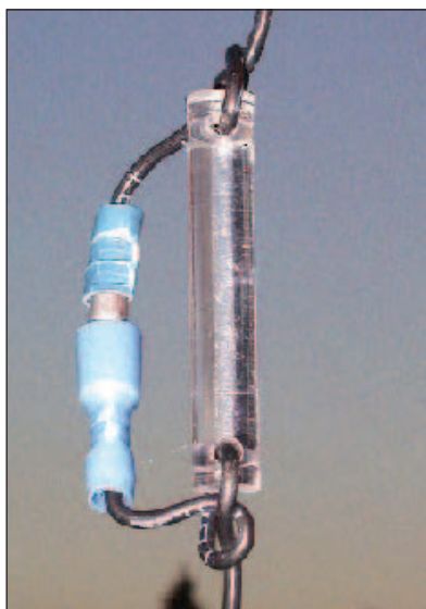
Figure 1 — Detail of the jumper connection. The connector is an automotive push-on type. The plastic insulator position is adjusted to keep the weight off the connection.
