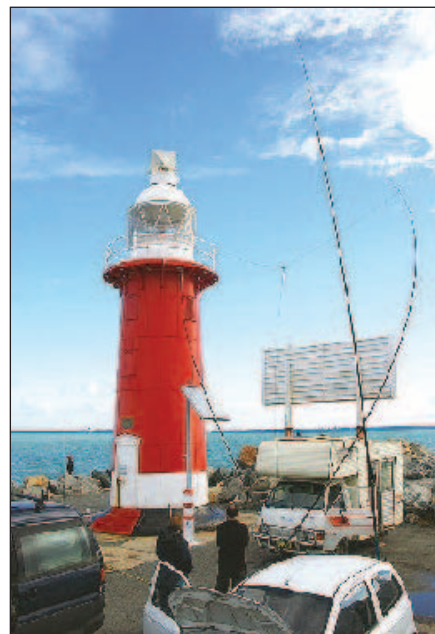
Two "Squidpoles" were used to support a dipole on the North Mole attached to the recreational vehicle. Also note the rather tall Squidpole attached to the bumper of Martin's auto; this supported a vertical wire with the counterpoise thrown in the salt water of the Indian Ocean.
