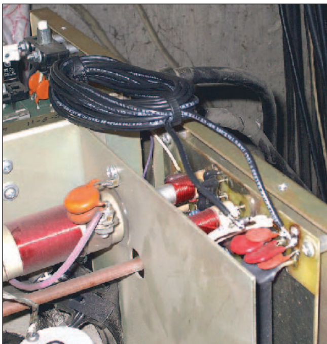
Figure 3 — Low value filament resistor made from THHN house wire installed at input of filament choke to reduce filament voltage.
