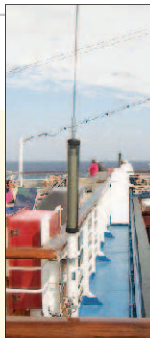
The ship's engineering department mounted the Tarheel screwdriver antenna on Deck 10 above the Lido deck.
