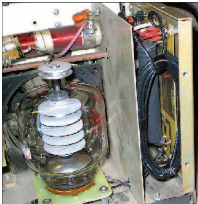
Figure 4 — Final position of the filament resistance wire, connected in series with the transformer side of the filament choke.
