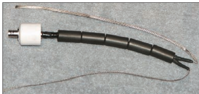
Figure 2 — Common mode choke made by sliding ferrite beads over the coax. This type has the edge at higher frequencies.
