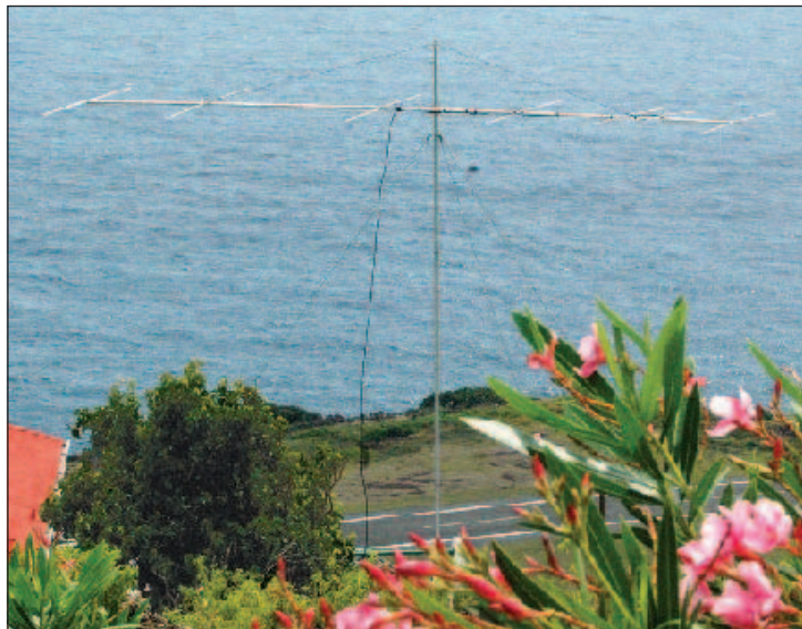
What a beautiful picture of the 7 element OWA designed 6 meter Yagi some 450 feet above sea level, with the Saba International Airport runway down below.
