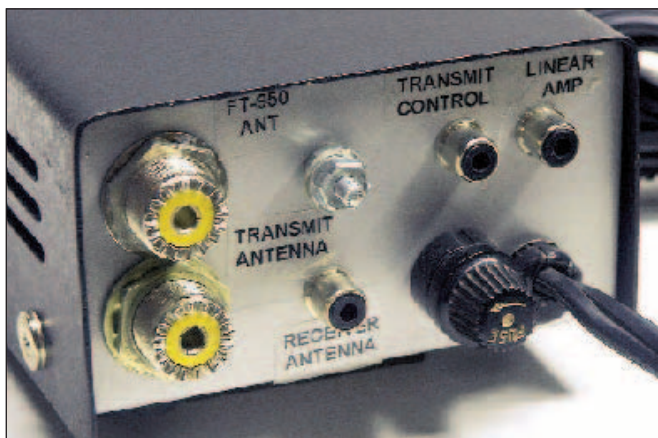
Figure 3 — Rear view of the adapter showing inter- face connector locations.
