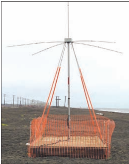
CODAR is used to measure the surface currents of the coastal ocean. A transmitter sends out a radio frequency that scatters off the ocean surface and back to a receive antenna. Using this information and the principles of the Doppler shift, CODAR is able to calculate the speed and direction of the surface current.
