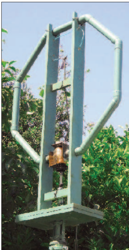
Figure 8 — The 3 foot diameter single turn loop for 14-30 MHz. Note the coupling loop used for excitation in both loop designs.
