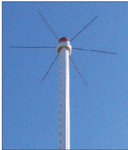
Figure 4 — The top section of the assembled antenna with the capacitance hat attached.
