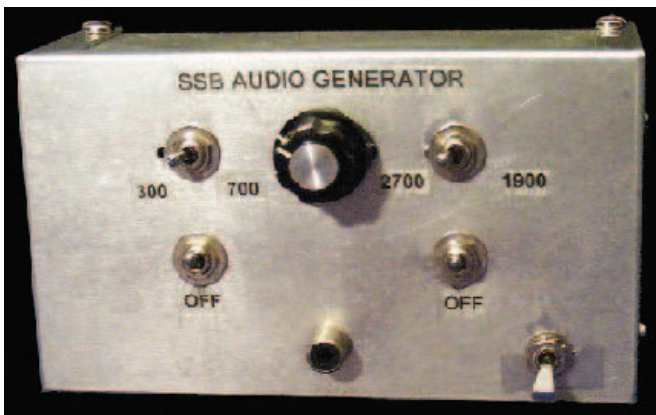
Figure 6 — Front panel of test generator. The OUTPUT jack (J1) and POWER switch (S5) are on the bottom. The knob adjusts R12, the OUTPUT LEVEL control.
