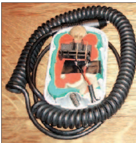
Figure 6 — The 12 V cord is attached to the connections removed from the dead battery pack.
