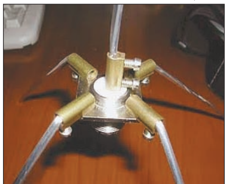
Figure 5 — Bend and trim the radials until you get a match and your antenna is ready to go.
