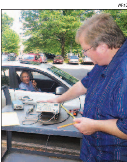
Figure 1 — Joel Hallas, W1ZR, transmits on 2 meters to a \frac{1}{4} wave whip on the rear fender while ARRL Lab Test Engineer Bob Allison, WB1GCM, measures the strong signal received on another \frac{1}{4} wave whip.
