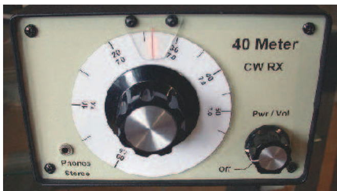
Figure 2 — This front panel view of the 40 meter receiver shows the tuning dial and indicator made by ACØDS.
