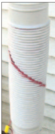
Figure 6 — The completed base coil. Note the slits that allow the wire to transition between grooves.
