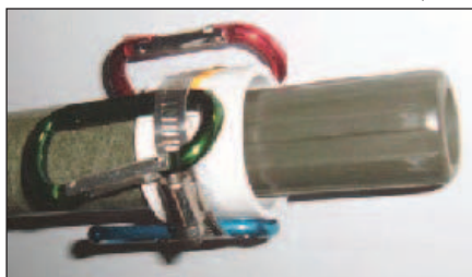
Figure 7 — Here is the temporary guy ring installed on the male end of a fiberglass mast section.
