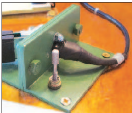
Figure 4 — Rear view of the paddle. The thumbscrew designed to hold the paddle in the KX1 is in its dedicated storage location so it will be there when needed for the trail.
