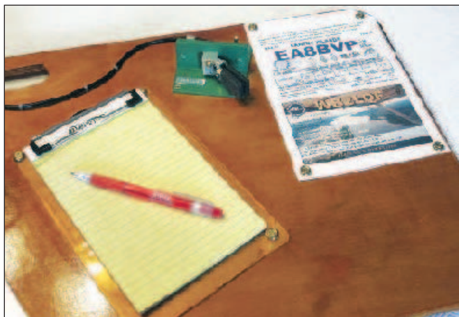
Figure 5 — The right side of the board includes the key, mounted at the correct angle for comfortable operation, a clipboard and a brag board to show off my latest QSL card.
