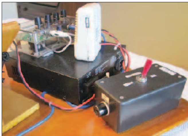
Figure 6 — The rear of the board's left side includes the power source switch to allow the station to be run from ac or dc power.
