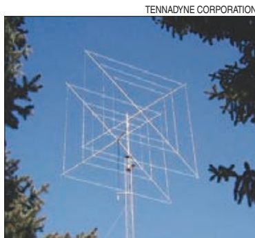
Figure 2 — A two element cubical quad from Cubex ( www.cubex.com ). Quads are also available in a diamond shape — mostly a matter of personal preference.
