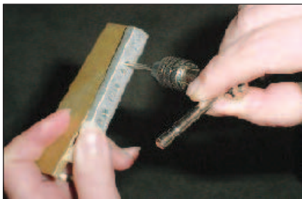
Figure 2 — Holding the tap guide against the work while starting to tap the hole will prevent the tap from entering the work at an angle, distorting the threads.
