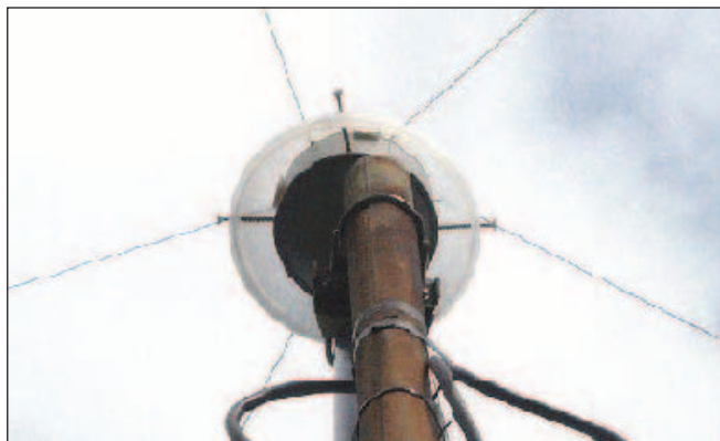
Figure 9 — Switch unit with dipole wires and weather protection cover placed on top of the supporting mast.
