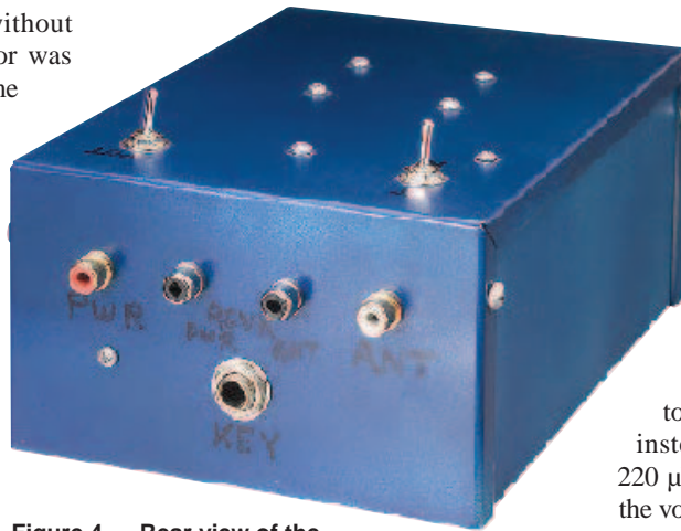
Figure 4 — Rear view of the transmitter. A somewhat large 3 × 5 × 7 inch aluminum enclosure (Mouser 546-1411QU) was used to avoid crowding.
