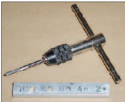
Figure 1 — The tap guide helps to keep the tap tool perpendicular to the work project's surface.
