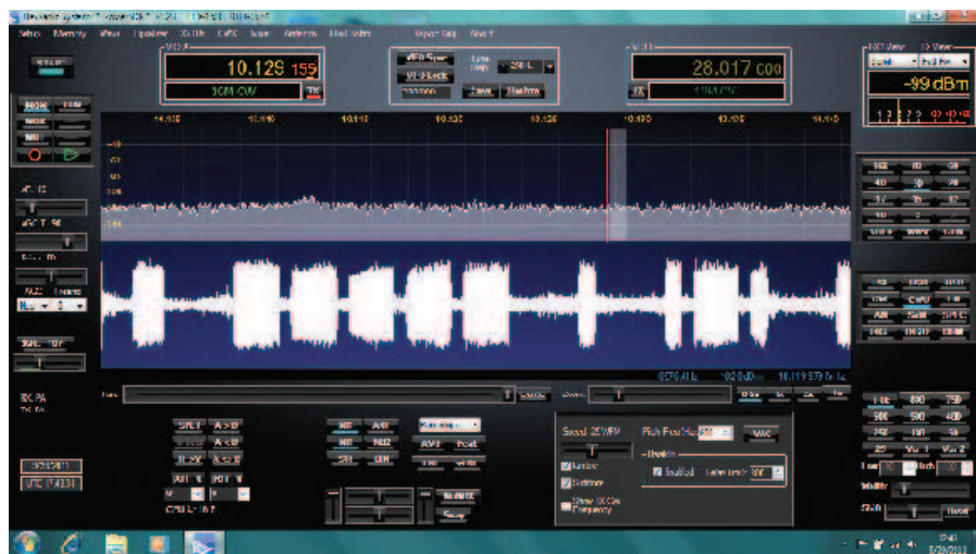
Figure 6 — A Panascope display shows both frequency domain (in the panadapter window) and time domain as an oscilloscope style trace on the bottom window. This is useful for CW and other keyed signals.
