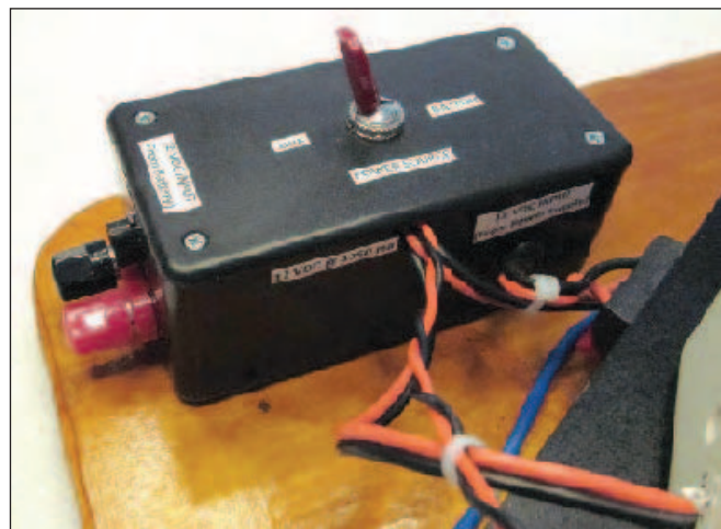
Figure 8 — The buttoned-up switch box. The terminals on the left allow easy connection of battery power.
