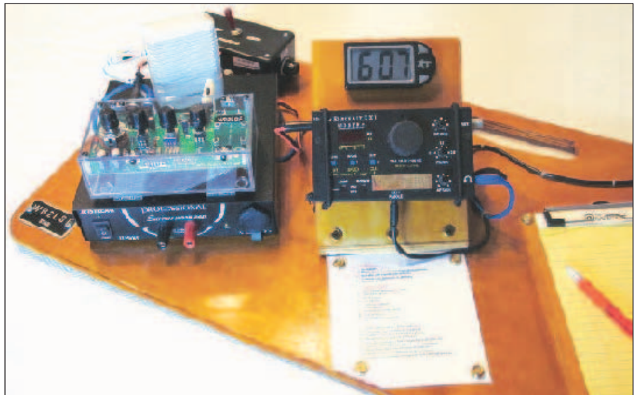
Figure 2 — Layout of the laptop station. The transceiver and clock are in the center, at appropriate angles and in clear view. Beneath the radio, an RST chart or other operating aid, mounted under plastic. On the left is a power supply, audio filter, amplified speaker and power source switch.
