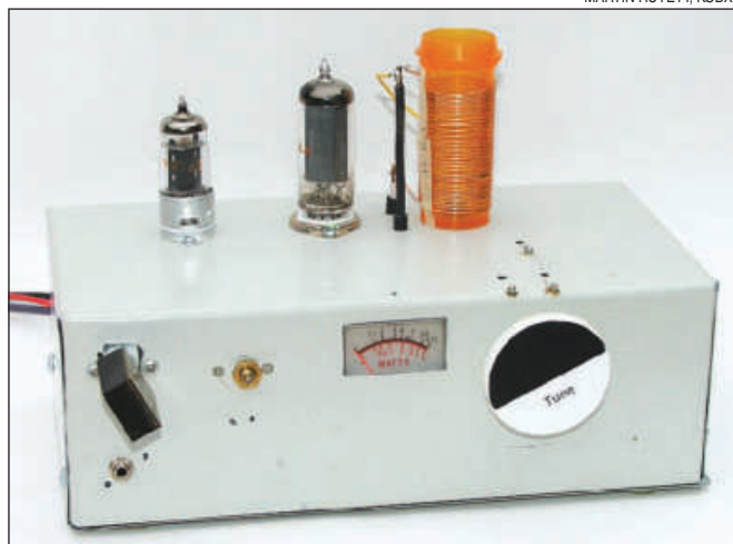
Martin, K0BXB, does like to build transmitters. This is his copy of the W1TS transmitter, which is quite compact since he used an external power supply.
