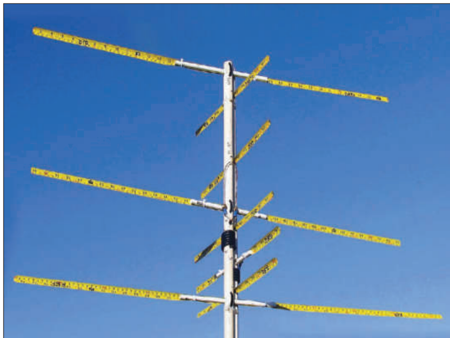
Figure 1 — Dual purpose, dual boom portable tape measure Yagi for 2 meters and 70 cm.
