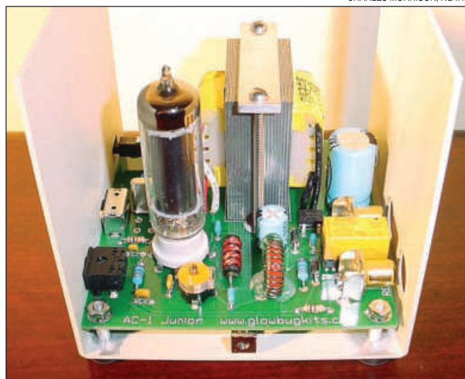
While most vintage projects are obviously scratch-built, there is at least one current kit on the market. This rig, the AC-1 ( www.glowbugkits.com ), puts out a 1 W signal and, as a result of the low power, keys beautifully with vintage or modern crystals.
