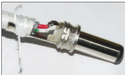
Figure 5 — Dental floss is thin, strong and heat resistant, making it an excellent choice for strain relief in a miniature connector.
