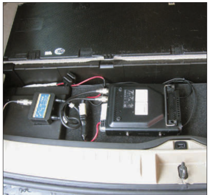
Figure 3 — Mounting of the main body of the transceiver, duplexer and associated cabling.
