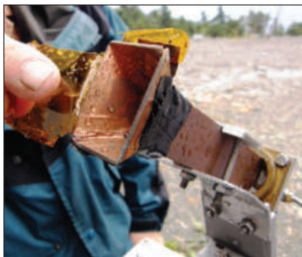
Figure 3 — Water in feedhorn.
