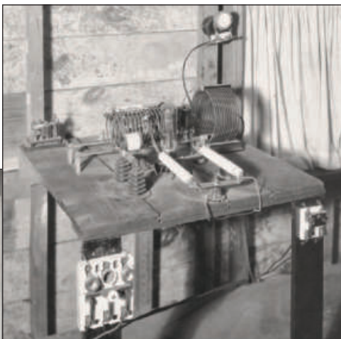
◀ 1928 shack receivers and controls for remote transmitter in attic.
