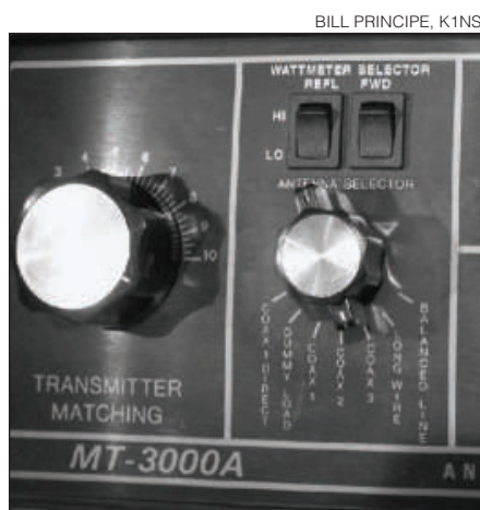
Figure 3 — The panel of my Dentron tuner is brushed aluminum with a painted background, making the white letters of my wattmeter selector switches' custom label appear slightly brighter.
