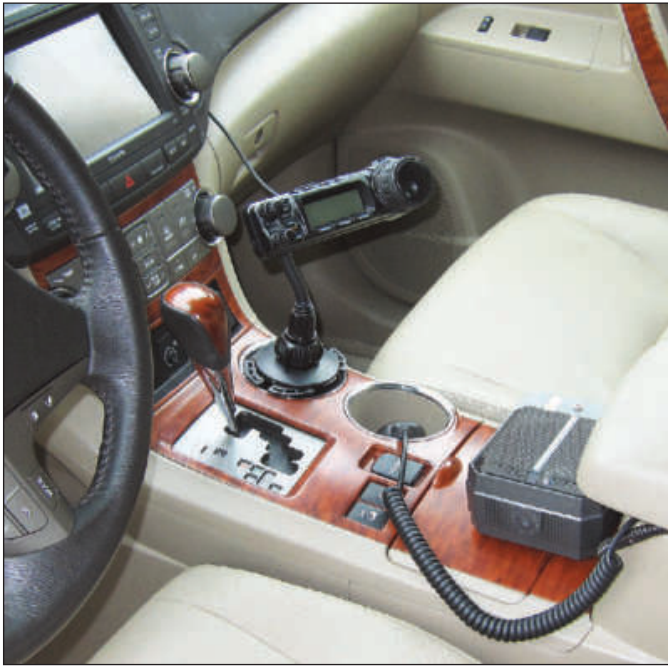
Figure 4 — Mounting of the front panel, DSP speaker and microphone on front console.
