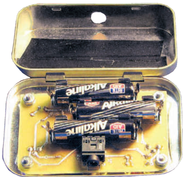
Figure 2 — Transistor tester circuit board mounted inside the case.
