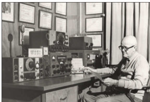
1961 — National NC-100, Collins 75A4 receivers, Viking Ranger and Collins 32V3 transmitters and Johnson Match Box tuner.
