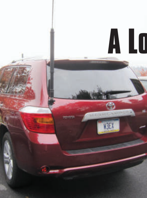
Figure 1 — Rear view of the Highlander with ATAS120 mounted on left side of the hatch door.
