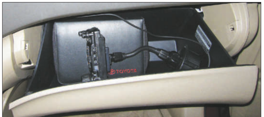
Figure 6 — Stealth mode location of front panel in glove compartment.
