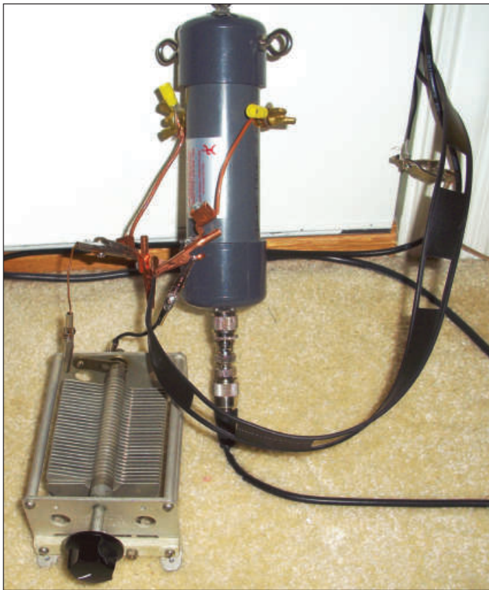
Figure 5 — With the single tuning element used at the antenna feed point (see Figure 4), I can tune the system in the shack (letting ladder line do some of the tuning job). A little less power efficiency but fewer “moving parts.”
