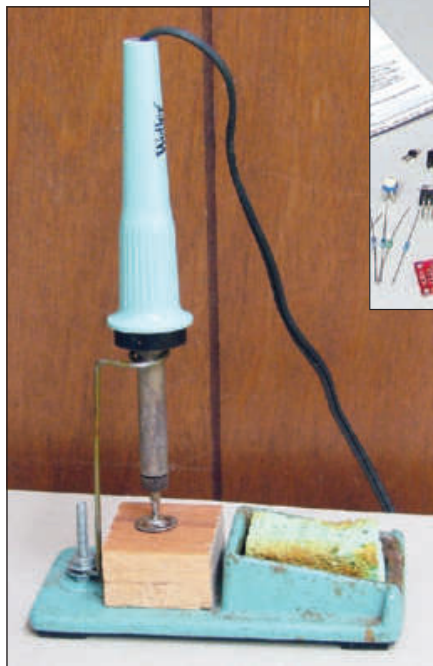
Figure 1 — The 25 W iron in its completed antioxidant holder.
