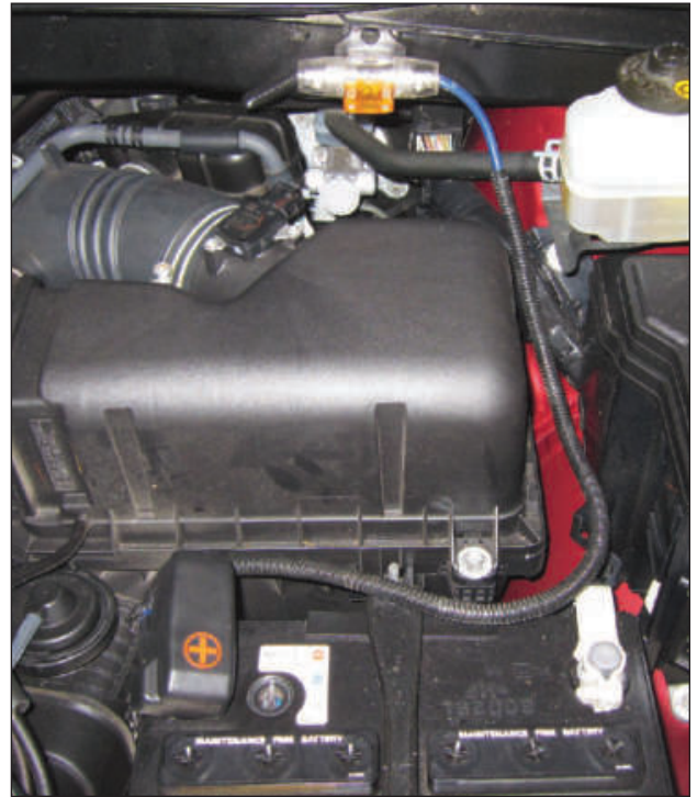
Figure 8 — Dedicated fused power cable installation in engine compartment.
