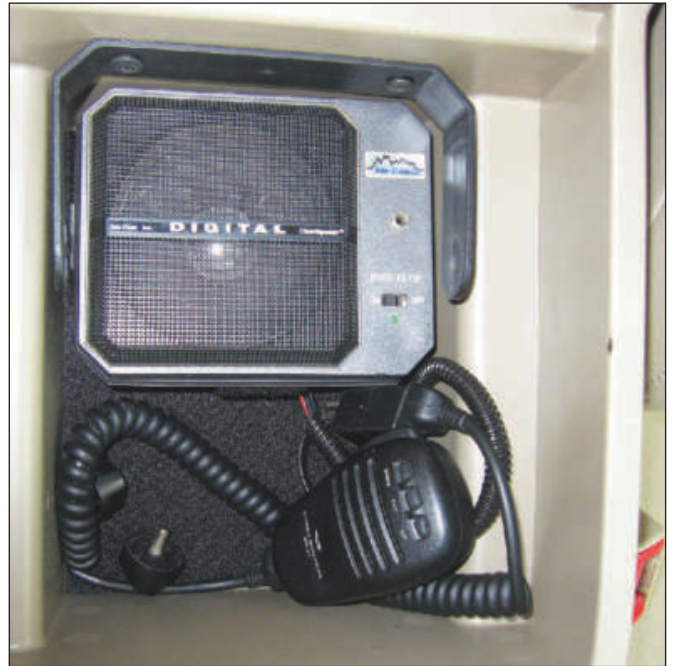
Figure 5 — Stealth mode location of speaker and microphone in front seat boot.
