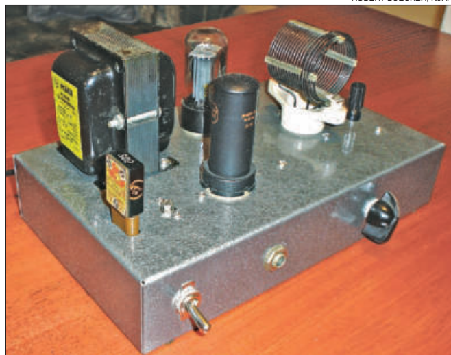
Bob, N9HAL, built this fine replica of a '50s 6AQ7 single-tube transmitter. This transmitter keys impeccably with vintage crystals but such designs, including more modern versions using the 6CL6 pentode, tend to have significant “chirp” when using modern crystals.
