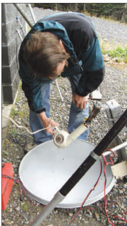
Figure 4 — Chip, W1AIM, drying out feedhorn with hair dryer.
