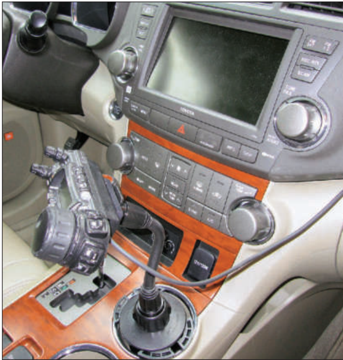
Figure 7 — Operating mode location of front panel showing routing of control cable from glove compartment.
