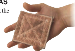
This wearable antenna is able to send a UHF signal to satellites using the Cospas-Sarsat worldwide search and rescue satellite system. It is made from highly flexible, lightweight material that is robust against water exposure and moist conditions and resistant to wear and tear.
