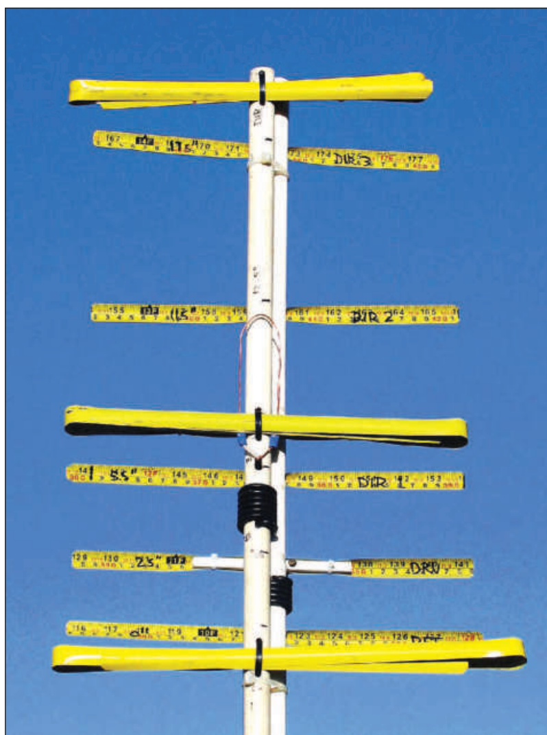
Figure 3 — Booms rotated 90° and 2 meter elements folded back. Note tie wraps to hold ends.
