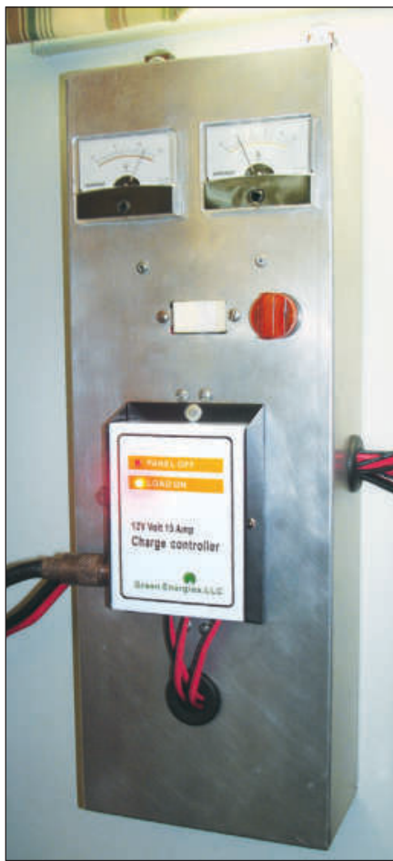
Figure 5 — Front panel view of the control box with the solar controller mounted on the front surface. The white rocker switch is a center off, three position switch that allows selection of BATTERY POWER, OFF or AC POWER SUPPLY.
