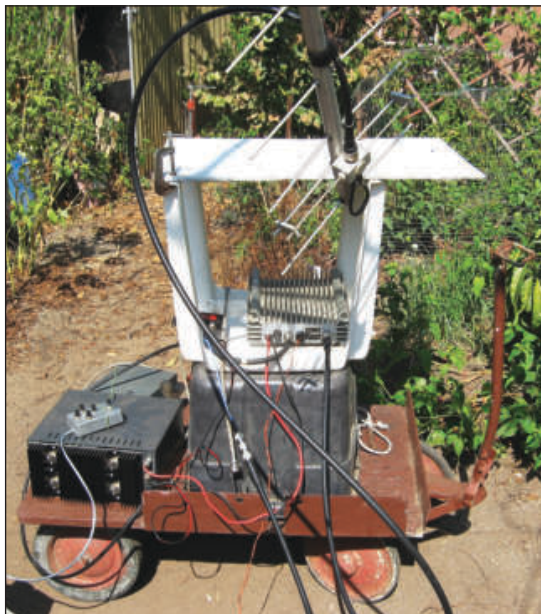
Figure 3 — The wagon holds the power amplifier, preamp and power supplies. The elevated platform raises the amplifier when the Yagi is horizontal and provides shade. The wired remote rotator switch box is shown on the left resting on the power supply.
