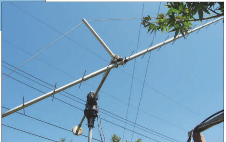
Figure 2 — This is the 28 element Yagi mounted on the directional and azimuth/elevation rotators.
