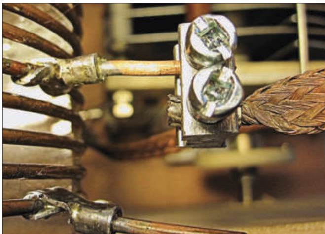
Figure 6 — The preliminary tap assembly showing the ring lug, the #10 AWG wire stub, the bus bar terminal strip and the coax braid jumper.
