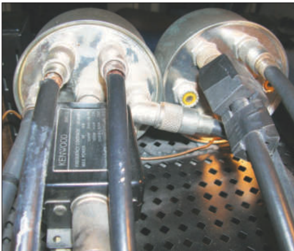
Figure 2 — Coax connectors and associated switches often add loss due to wear and tear — especially of the spring contacts on SO-239 sockets. Watch for oxidation under any riveted connections. They should read 0.0 \Omega when checked with an ohmmeter.
