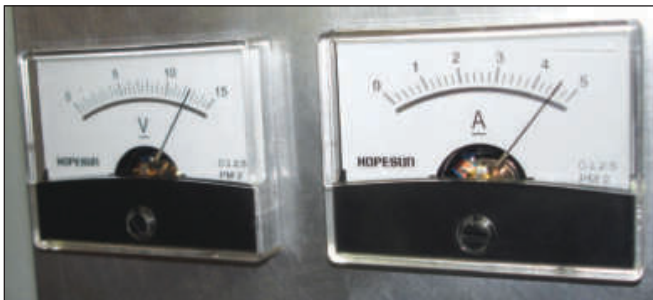
Figure 6 — The panel meters in operation. It is interesting to watch the charge current vary as clouds pass by, obscuring the direct sunlight.
