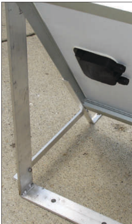
Figure 2 — Rear view showing the aluminum frame mounted to the solar panel itself.
