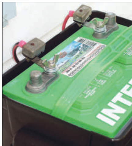
Figure 4 — The deep discharge battery mounted in a standard RV battery case. The top has been removed to show the connections via the two SAE 25 A automotive circuit breakers.
