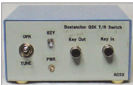
Figure 4 — The front panel includes controls, indicators and the key in and out jacks.
