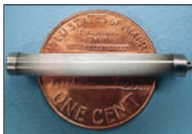
A implantable microstimulator of the kind that would be used with a wireless medical micropower network.
