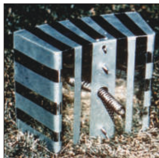
The underside of OSCAR 1, showing the $1.29 spring used to eject OSCAR from the host spacecraft. OSCAR was curved to fit the contour of the Thor-Agena rocket.
