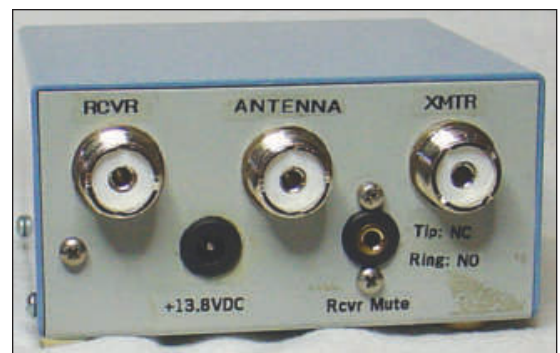
Figure 5 — The rear panel has the jacks for the antenna connections as well as power and standby switching.
