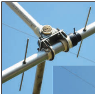
Figure 1 — The PVC bushings allow the boom to be twisted in its mount to adjust the polarization for receiving and transmitting.
