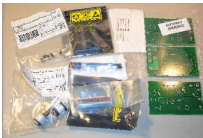
Figure 1 — Before beginning assembly make a thorough inspection of all parts and the finished PC boards. Be sure custom components fit their hole pattern properly.
