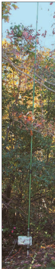
Figure 1 — A representative electrical quarter wave long HF vertical antenna. This is the SmallIR from SteppIR. The motor control unit near the bottom moves a metal tape up and down within the fiberglass radome to set the resonant frequency.
