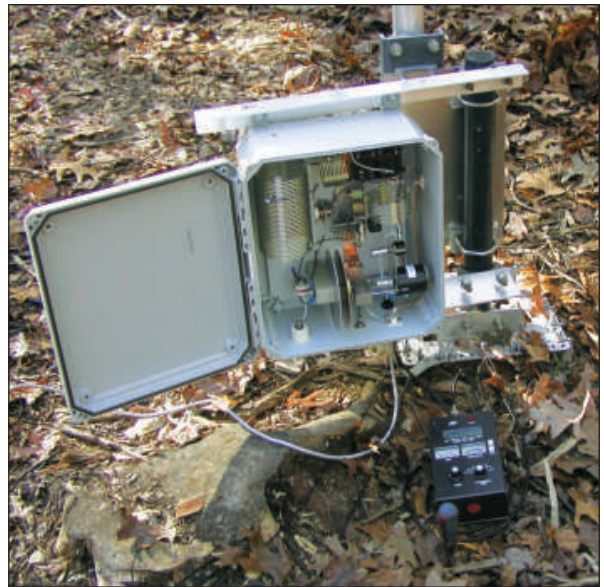
Figure 10 — The finished RF deck and enclosure, mounted at the antenna base.
