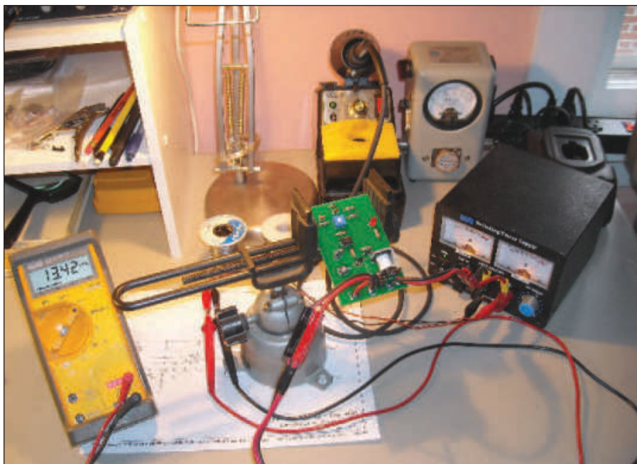
Figure 3 — The completed board being tested on the workbench. Anderson Powerpole connections were used to connect to the adjustable power supply and the ICOM IC-207H mobile rig serving as a test load.
