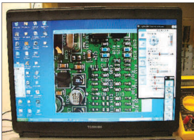
Figure 2 — The laptop screen showing a portion of the PCB with the tiny surface mounted components.
