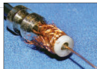
Figure 4 — Placing a plastic washer or other insulator on the end of the cable before inserting it into the connector body will prevent the shield from shorting against the center-pin rim.
