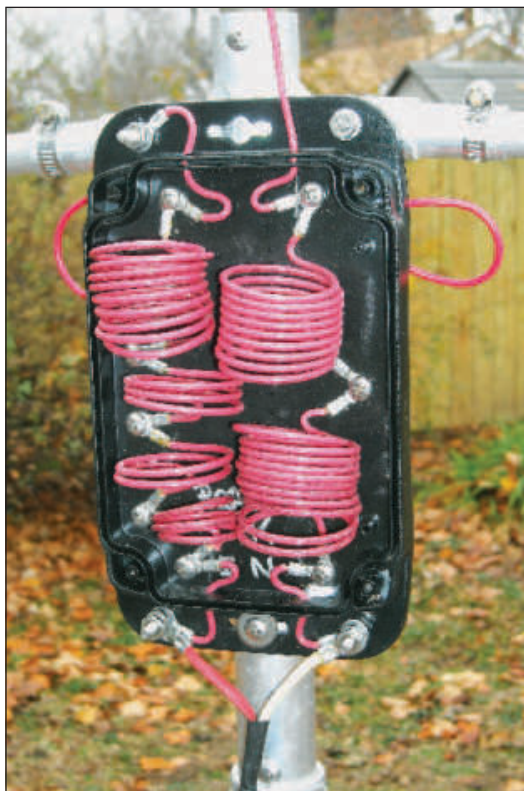
Figure 10 — Loading inductors are added in series with the vertical and radial elements on different bands. No inductance is required on 10 and 12 meters. Mounting screws have been turned around from the stock configuration.
