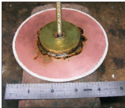
Figure 3 — Rotating disk of the tuning capacitor made from high frequency PC board material.
