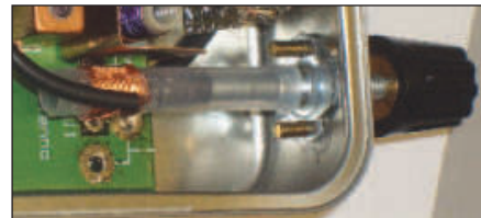
Figure 5 — Here is the mechanical arrangement HB9WI uses to tune the frequency of a small 14 MHz transmitter. The knob turns a piece of machine screw, which threads a piece of ferrite core material into and out of the tuning coil.
