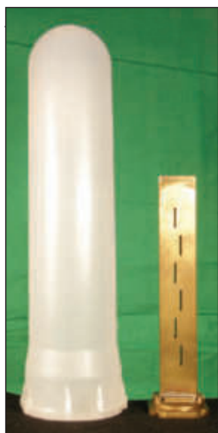
Figure 3 — Slot antennas require weatherproofing. Here is one possible radome for the 12 slot antenna.
