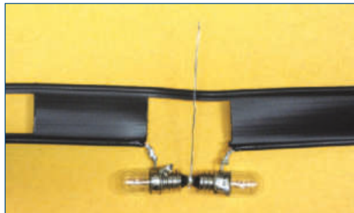
Figure 2 — A 2011 rebuild of the 1947 circuit. The window line section is 18 inches long.
