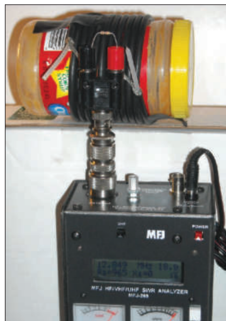
Figure 3 — A smaller diameter coil may have similar inductance to a larger coil but its lower Q causes its impedance curve to be broader. All coils in this article are made from the same length of coax feed line.
