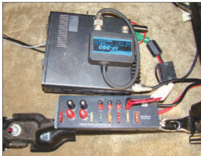
Figure 7 — ICOM IC-706 body and power distribution, located behind the driver under the second row seats of the SUV.
