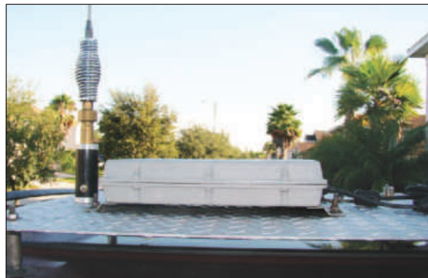
Figure 3 — Mounting service plate that holds the automatic antenna tuner and antenna mount.
