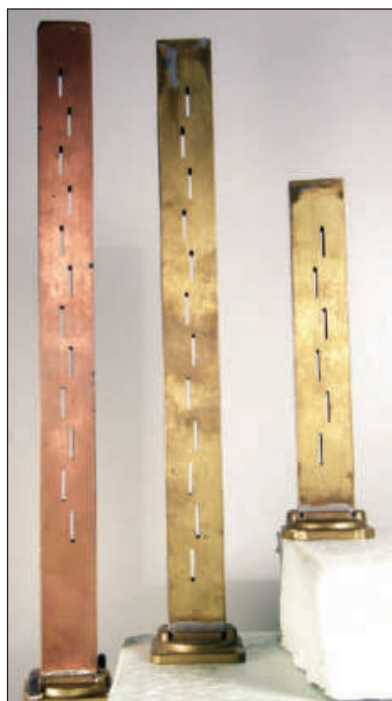
Figure 1 — These are three waveguide slot array antennas for 10 GHz made from WR-90 waveguide.
