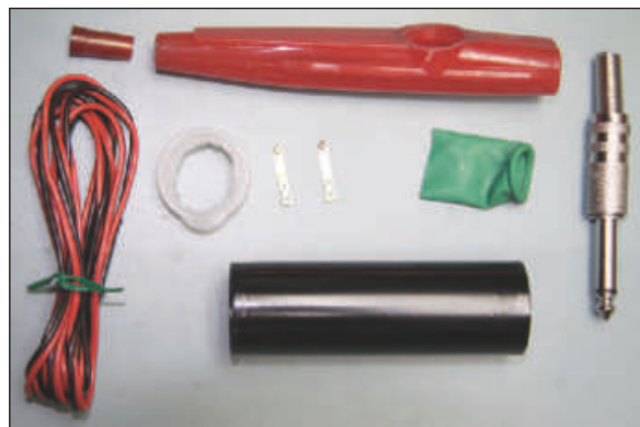
Figure 3 — The parts needed to create your own breath-activated key are, clockwise from left, wire, stopper, kazoo, transceiver plug, shell, shell cover, contacts and balloon.
