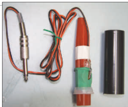
Figure 5 — The breath-activated key ready for you to plug into your transceiver and make CW music on the bands.
