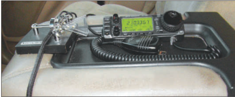
Figure 8 — Paddle and radio remote control panel located on driver's armrest.
