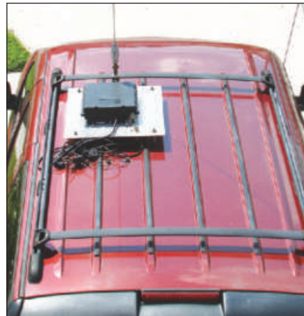
Figure 2 — Top view of mounting. The plate location aligns with second row seats just behind driver seat.
