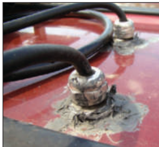
Figure 5 — Close-up of RG-58 entering cabin via waterproof cable grips. Note the application of RTV sealant.
