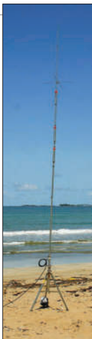
The NP3PR operation used this homebrew vertical for 10-15-20-40 meters.
