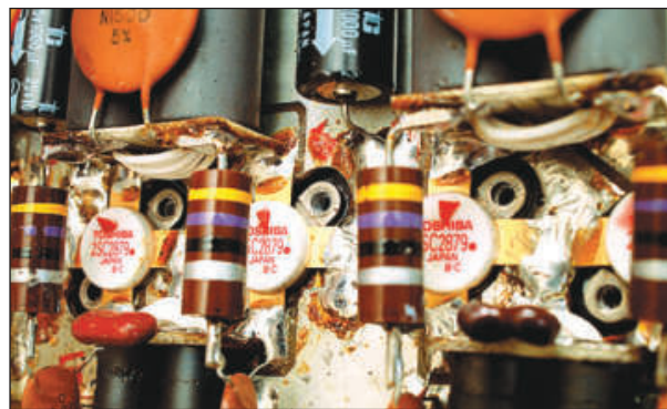
Figure 1 — To begin the test, place small chips of candle wax on each of the transistors to be tested. Here the wax chips are visible at the 12 o'clock position.
