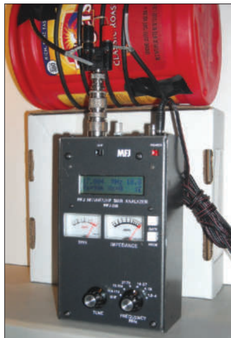
Figure 1 — The coiled-coax choke balun is wound on a plastic form and attached to the analyzer using a binding-post adaptor. The analyzer then reads R_S and X_S . A 1 k \Omega swamping resistor across the binding posts limits the variations in R_S and X_S to displayable values.
