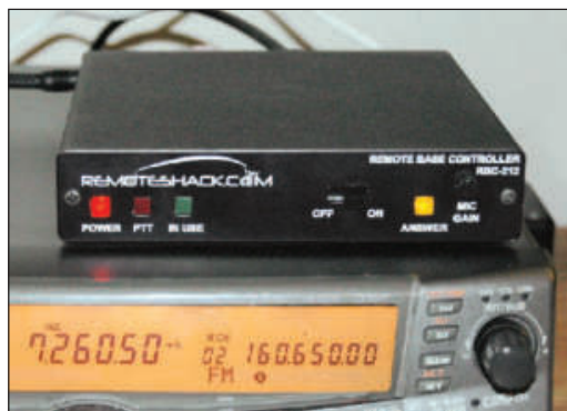
The RemoteShack RBC-212 controlling the author's Kenwood TS-2000 transceiver.
