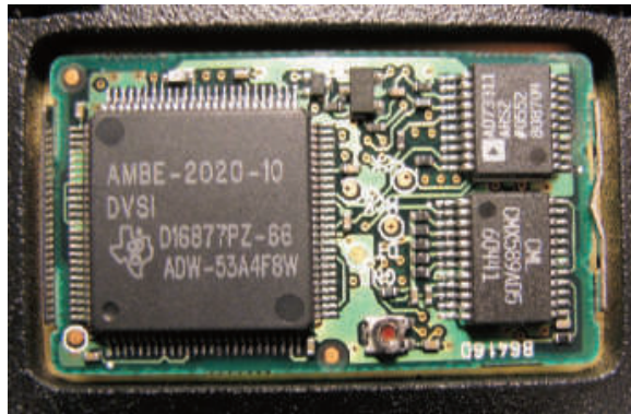
Figure 9 — The AMBE 2020 Vocoder in this IC-91AD handheld does the analog to digital encoding and decoding. It is the only proprietary component of the D-STAR system.
