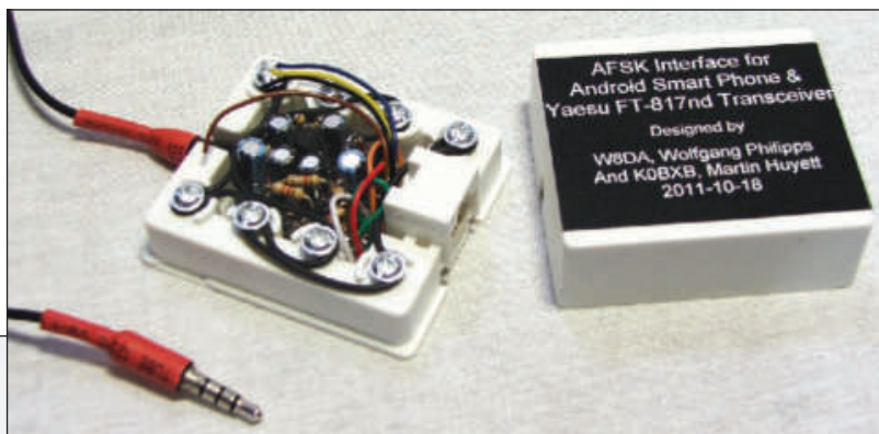
Figure 3 — The K0BxB interface in RJ45 wall mount box.
