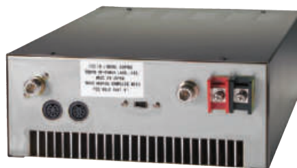
Figure 1 — Rear panel of the HL-350V DX linear amplifier. The RF INPUT and RF OUTPUT connectors are both Type-N. The slide switch selects nominal 10, 25 or 50 W nominal drive levels (see text). Mini DIN connectors are for a remote control option and for TR control. Note that the identification markings are on a sticker on the bottom of the amplifier.
