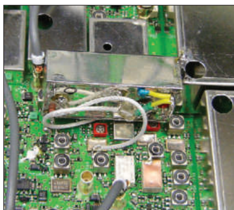
Figure 3 — Initially we installed the filter as shown here. It didn't perform as expected, and we learned that the leads were too long and the capacitor was not needed with our radio.
