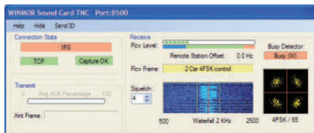
Figure 4 — WINMOR virtual terminal node controller screen showing connection state, receive waterfall and received constellation (phase display).
