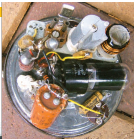
A close-up of the 3 W coffee-can transmitter built using the "ugly" construction method. [George Dörner, W9ZSJ, photo]
