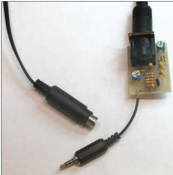
Figure 4 — W8DA's interface built using a home designed and etched printed circuit board.
