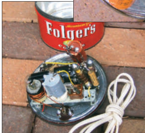
The completed 1953 coffee can transmitter. Its 3 W provided the author with his first low-power experience. [George Dörner, W9ZSJ, photo]
