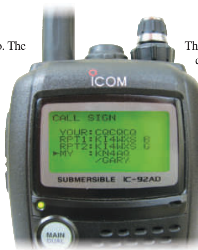
Figure 1 — The four D-STAR call sign fields are shown in the display of this ICOM IC-92AD handheld. Note that the RPT1 and RPT2 call signs have a port letter appended.
