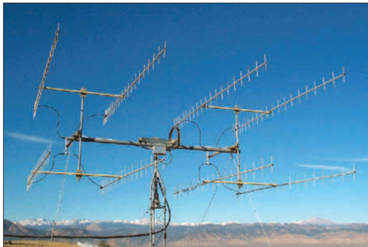
Figure 1 — Bill McCaa's, KØRZ, array of eight, 22 element Yagis used to set the 75 mile DTV DX record. [Bill McCaa, KØRZ, photo]
