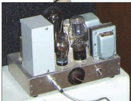
This photo shows Don's version of the Collins 7X speech amplifier/control-grid modulator.
