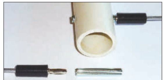
Figure 5 — A ¼ inch wide by 1½ inch long roll pin driven through the PVC boom of the portable Yagi will replace the two banana jacks used in the original design. [Richard Gillette, W9PE, photo]
