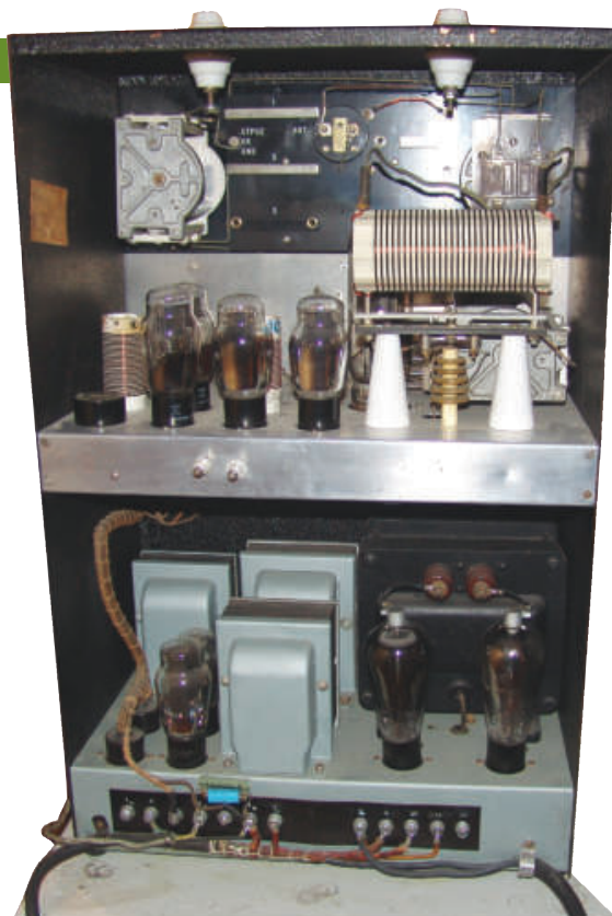
This rear view shows the interior of the Collins 30FX transmitter after Don's exceptional restoration job.
